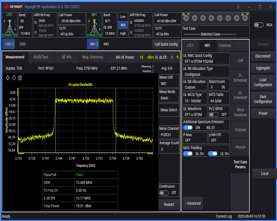
n77 SCS=30kHz DFT_QAM16 BW=20MHz Channel=650000 RB=50@0
