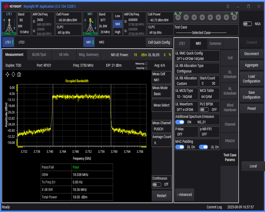
n77 SCS=30kHz DFT_QAM16 BW=50MHz Channel=650000 RB=128@0
