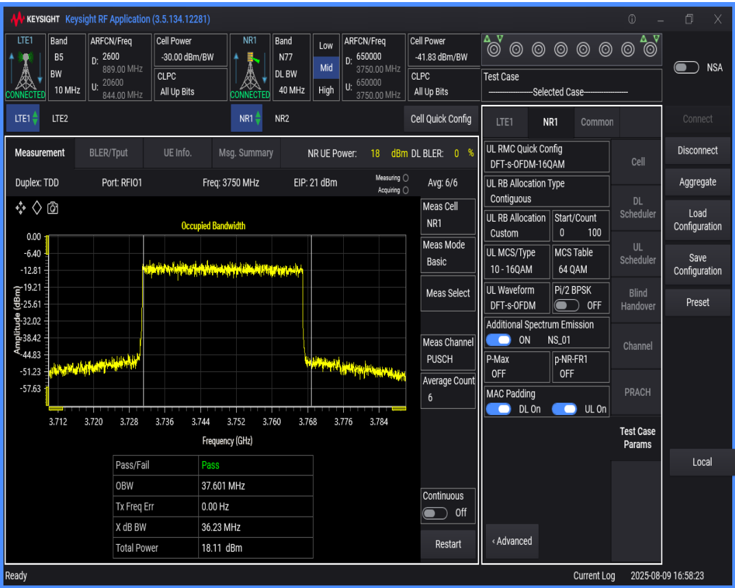
n77 SCS=30kHz DFT_QAM16 BW=60MHz Channel=650000 RB=162@0
