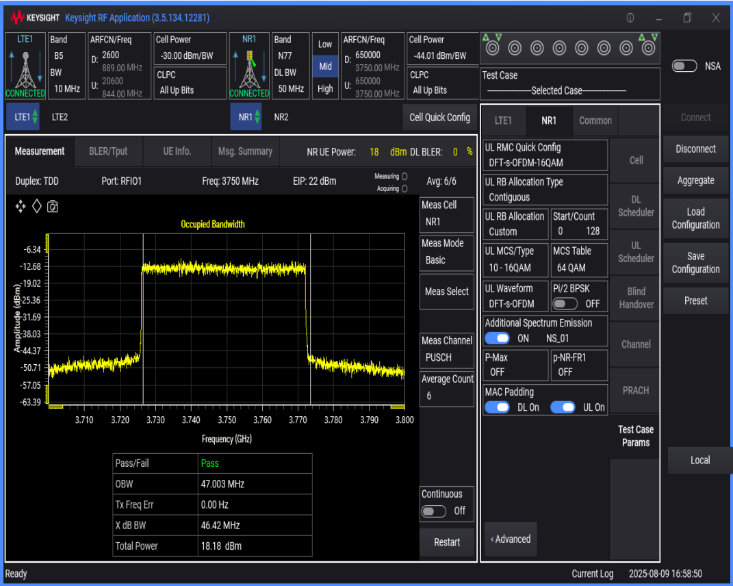
n77 SCS=30kHz DFT_QAM16 BW=40MHz Channel=650000 RB=100@0
