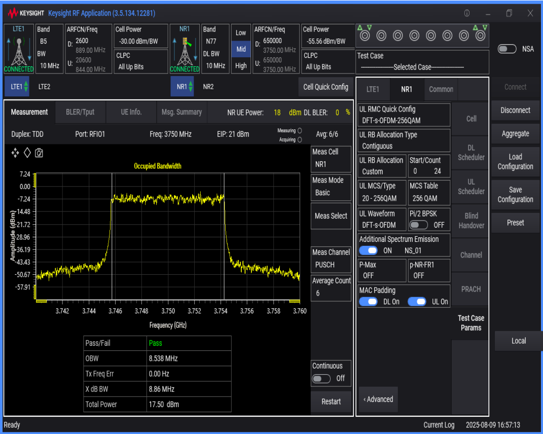
n77 SCS=30kHz DFT_QAM256 BW=40MHz Channel=650000 RB=100@0
