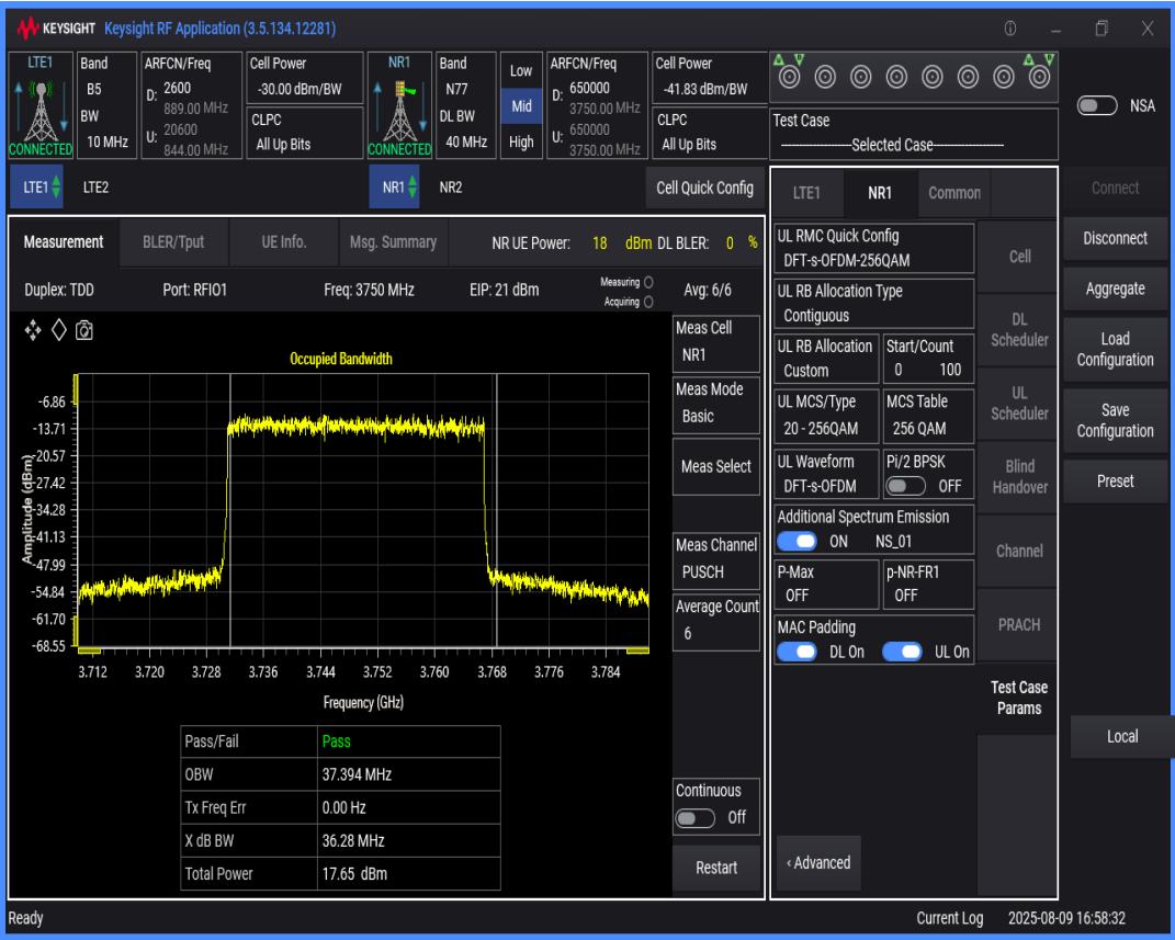
n77 SCS=30kHz DFT_QAM256 BW=60MHz Channel=650000 RB=162@0
