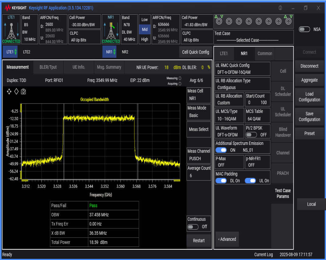
n78 SCS=30kHz DFT_QAM16 BW=90MHz Channel=636666 RB=240@0
