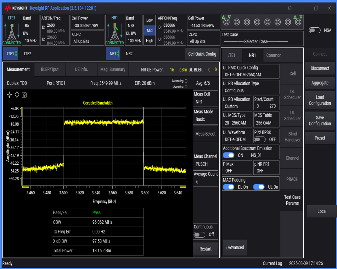
n78 SCS=30kHz DFT_QAM256 BW=10MHz Channel=636666 RB=24@0
