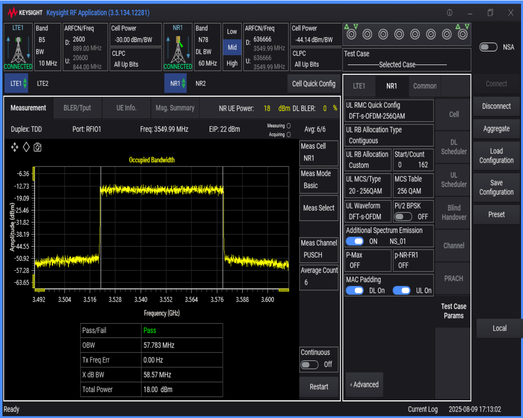
n78 SCS=30kHz DFT_QAM256 BW=40MHz Channel=636666 RB=100@0
