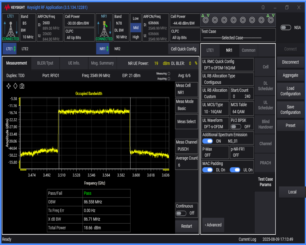
n78 SCS=30kHz DFT_QAM256 BW=100MHz Channel=636666 RB=270@0
