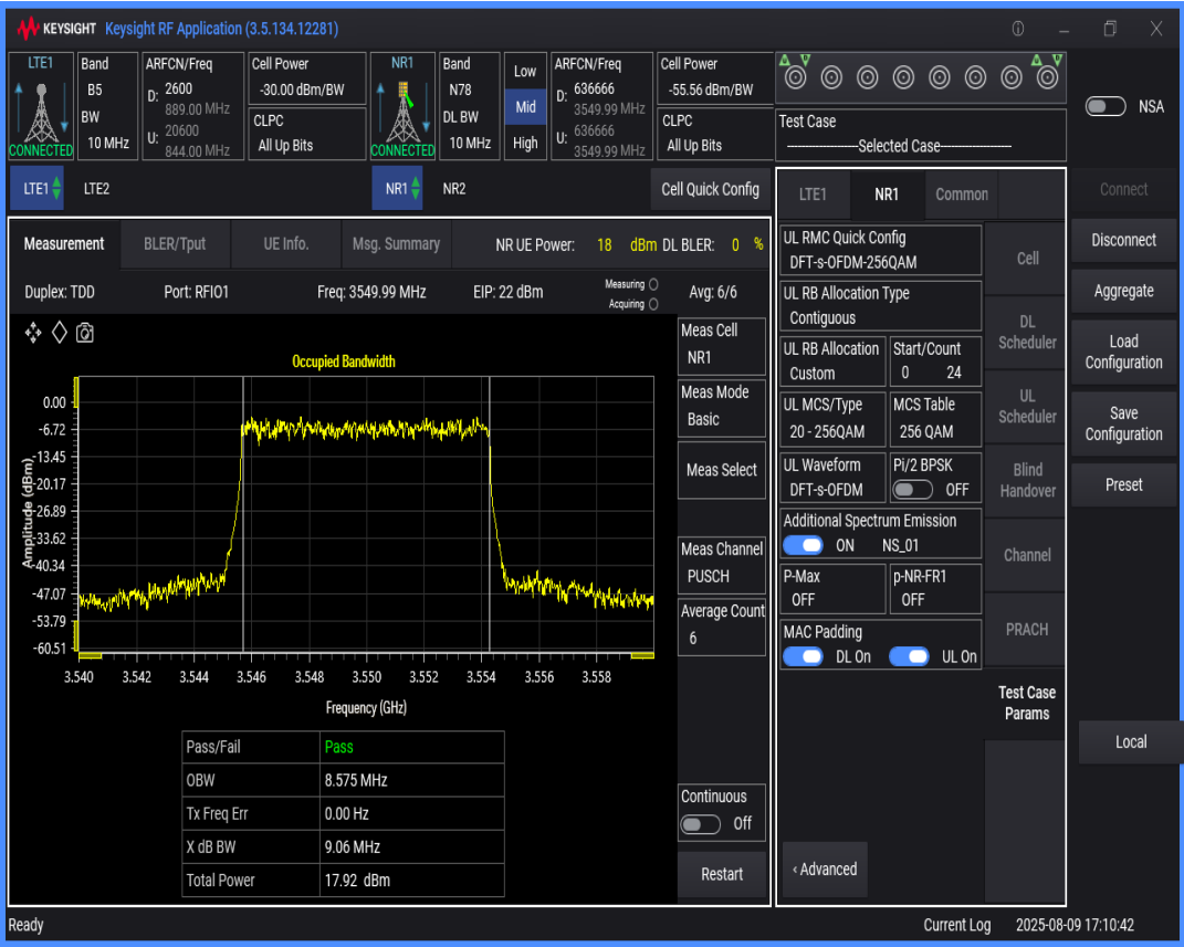
n78 SCS=30kHz DFT_QAM16 BW=50MHz Channel=636666 RB=128@0
