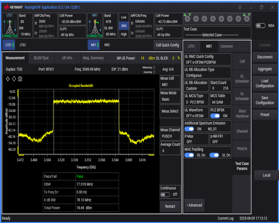
n78 SCS=30kHz DFT_BPSK BW=90MHz Channel=636666 RB=240@0
