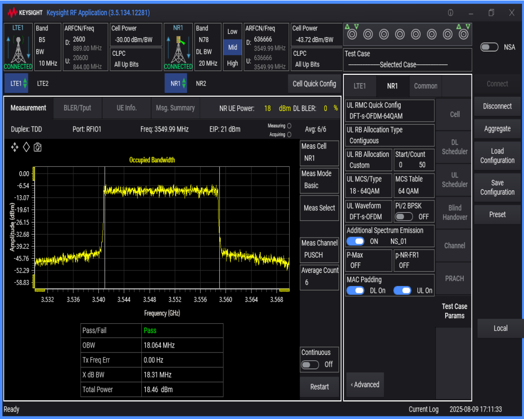
n78 SCS=30kHz DFT_QAM64 BW=40MHz Channel=636666 RB=100@0
