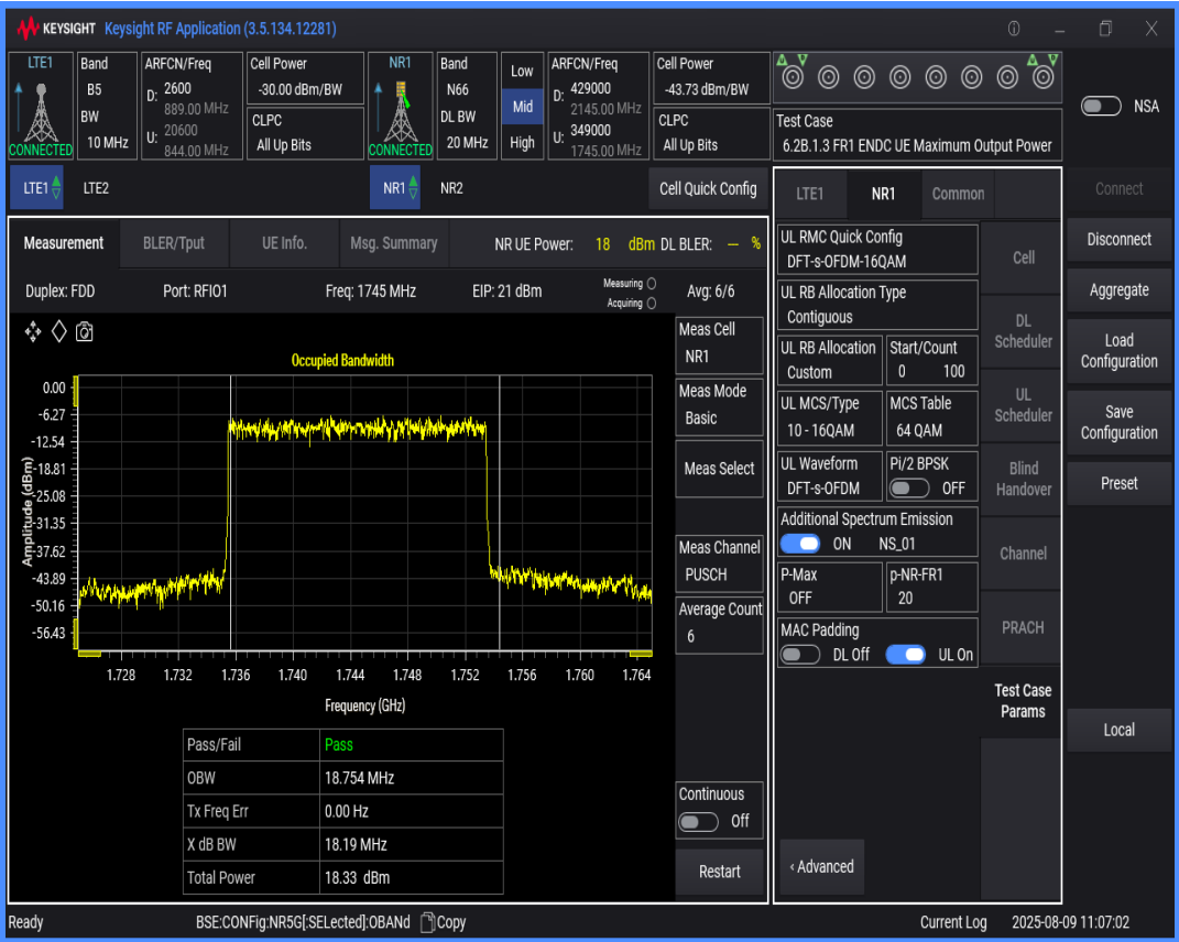
n66 SCS=15kHz DFT_QAM16 BW=15MHz Channel=349000 RB=75@0
