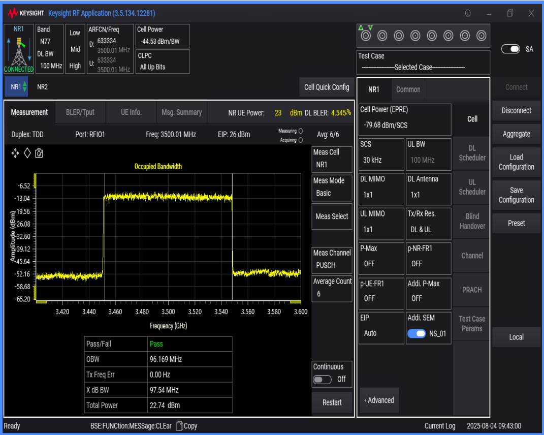
n77(3450-3550) SCS=30kHz DFT_QAM64 BW=60MHz Channel=633334 RB=162@0
