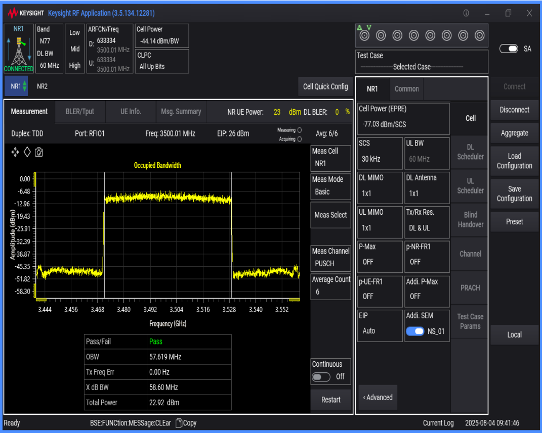
n77(3450-3550) SCS=30kHz DFT_QAM64 BW=80MHz Channel=633334 RB=216@0
