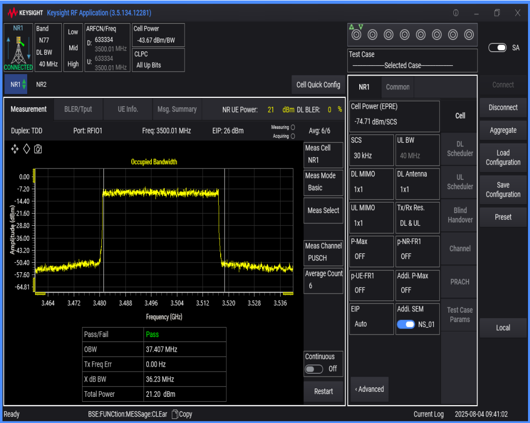
n77(3450-3550) SCS=30kHz DFT_QAM256 BW=50MHz Channel=633334 RB=128@0
