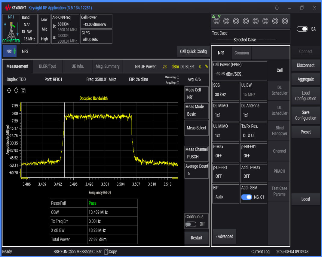
n77(3450-3550) SCS=30kHz DFT_QAM64 BW=20MHz Channel=633334 RB=50@0
