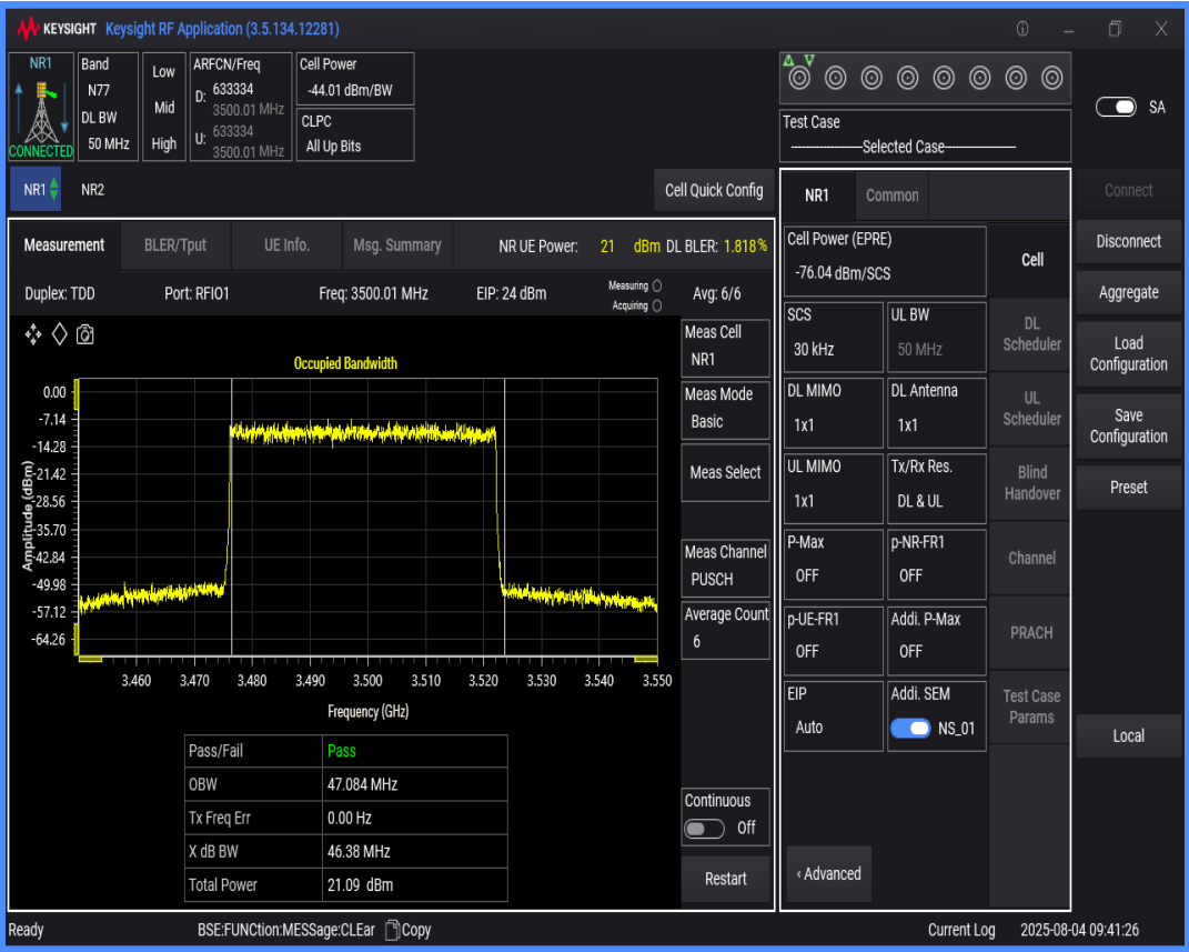
n77(3450-3550) SCS=30kHz DFT_QAM64 BW=15MHz Channel=633334 RB=36@0
