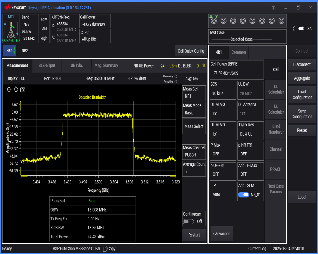
n77(3450-3550) SCS=30kHz DFT_QPSK BW=80MHz Channel=633334 RB=216@0
