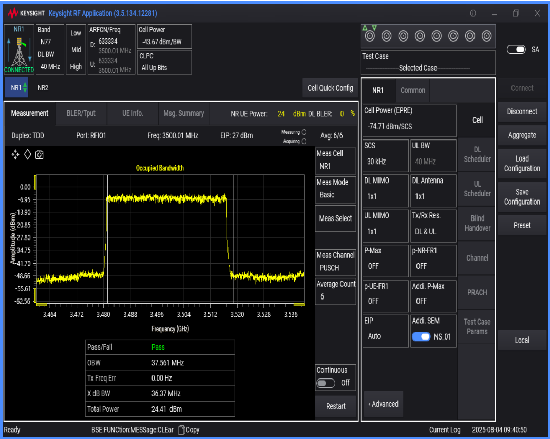
n77(3450-3550) SCS=30kHz DFT_QPSK BW=15MHz Channel=633334 RB=36@0
