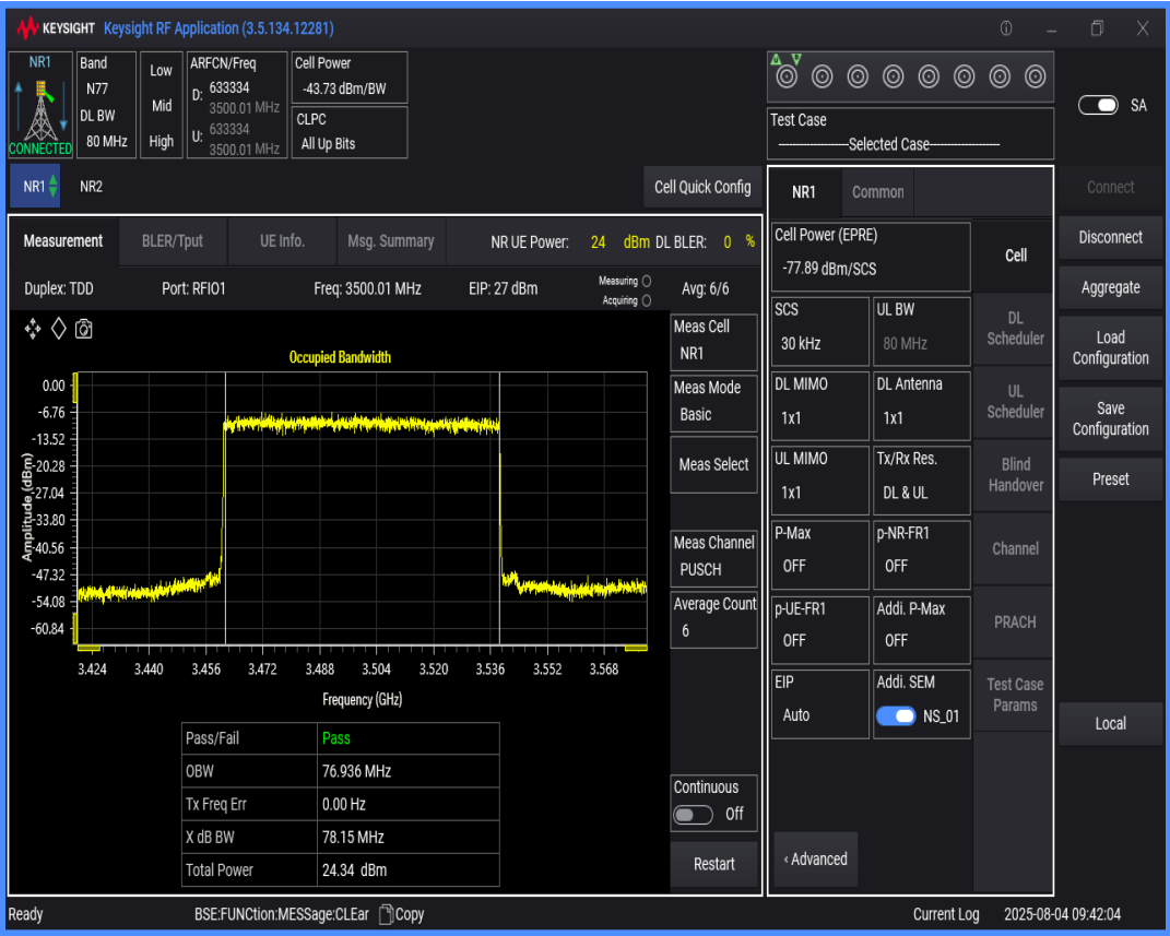
n77(3450-3550) SCS=30kHz DFT_QPSK BW=90MHz Channel=633334 RB=240@0
