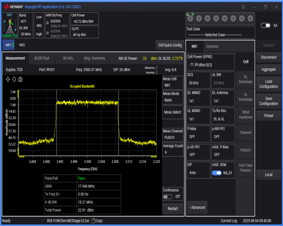
n77(3450-3550) SCS=30kHz DFT_QAM64 BW=10MHz Channel=633334 RB=24@0
