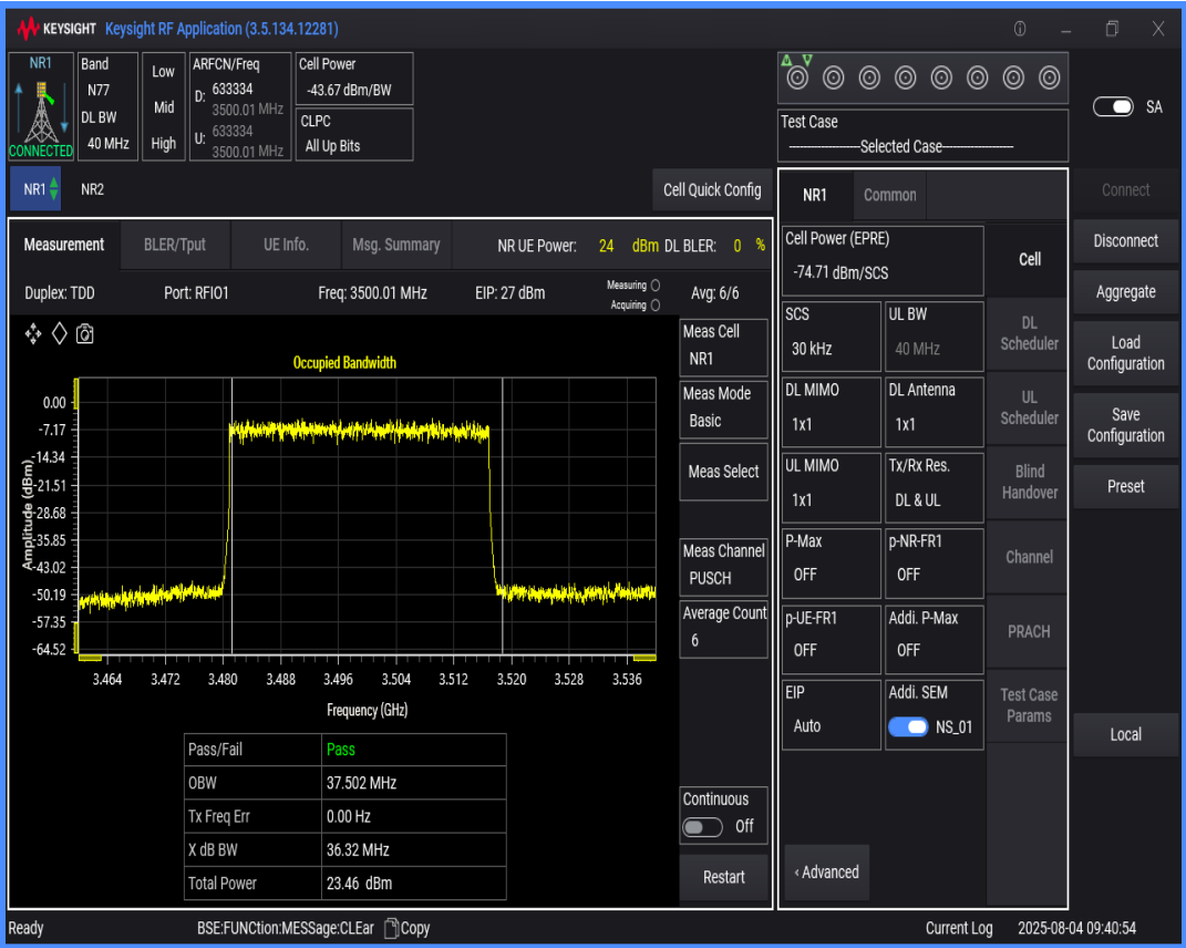
n77(3450-3550) SCS=30kHz DFT_QAM16 BW=80MHz Channel=633334 RB=216@0
