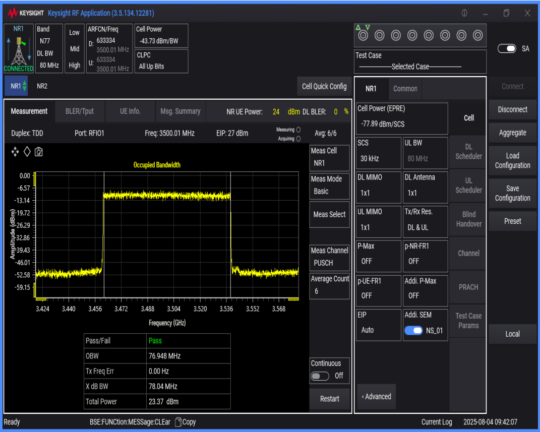
n77(3450-3550) SCS=30kHz DFT_QAM16 BW=90MHz Channel=633334 RB=240@0
