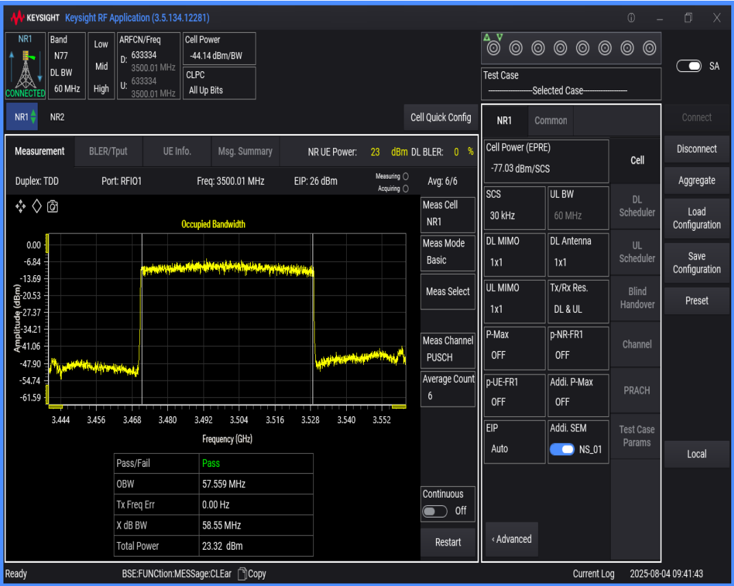
n77(3450-3550) SCS=30kHz DFT_QAM16 BW=50MHz Channel=633334 RB=128@0
