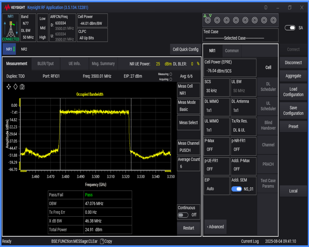
n77(3450-3550) SCS=30kHz DFT_QAM16 BW=10MHz Channel=633334 RB=24@0
