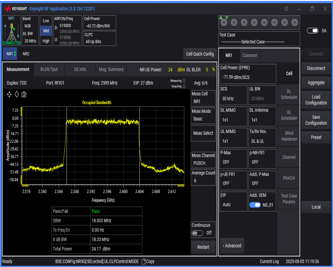
n38 SCS=30kHz DFT_QAM16 BW=10MHz Channel=519000 RB=24@0
