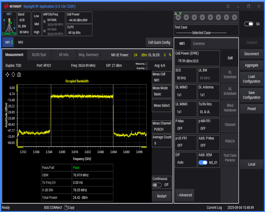
n78(3550-3700) SCS=30kHz DFT_QAM16 BW=10MHz Channel=641666 RB=24@0
