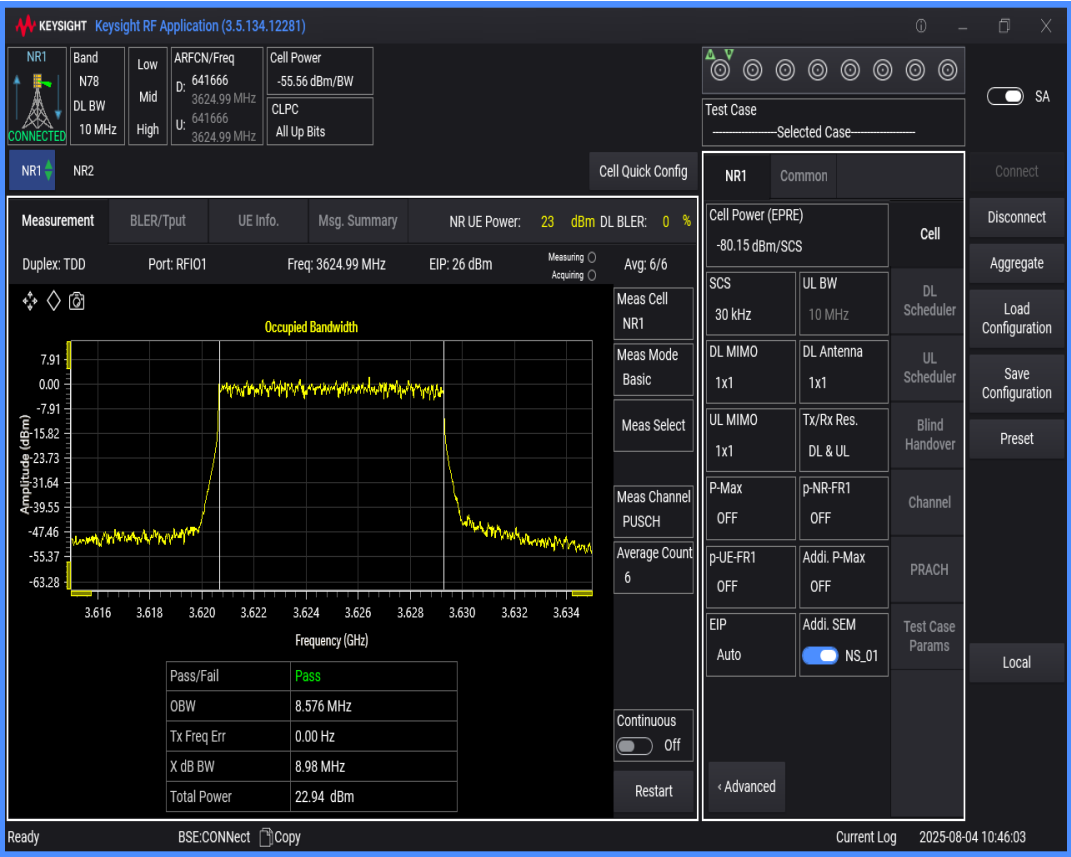
n78(3550-3700) SCS=30kHz DFT_QAM16 BW=100MHz Channel=641666 RB=270@0
