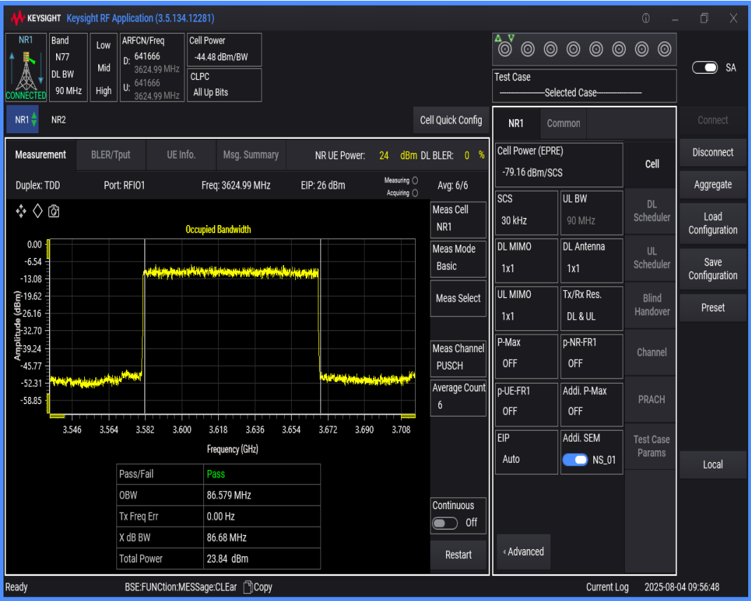
n77(3550-3700) SCS=30kHz DFT_QPSK BW=80MHz Channel=641666 RB=216@0
