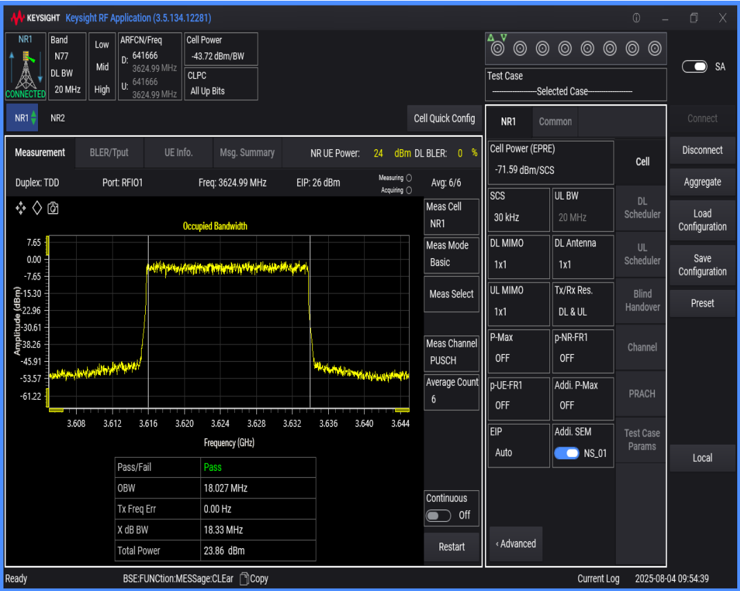
n77(3550-3700) SCS=30kHz DFT_QPSK BW=90MHz Channel=641666 RB=240@0
