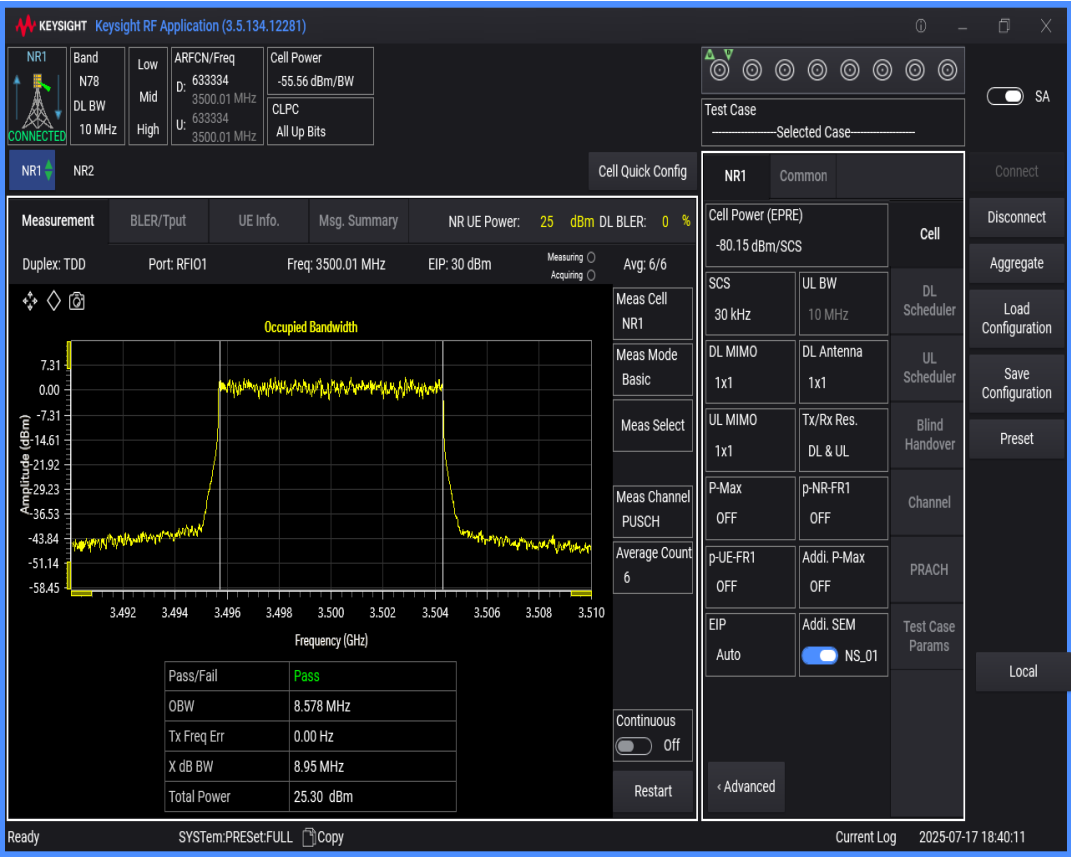
n78(3450-3550) SCS=30kHz DFT_QAM64 BW=30MHz Channel=633334 RB=75@0
