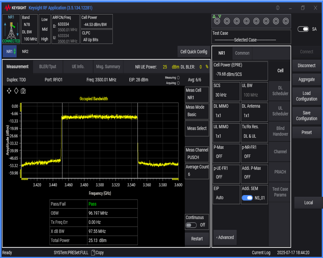
n78(3450-3550) SCS=30kHz DFT_QAM64 BW=10MHz Channel=633334 RB=24@0
