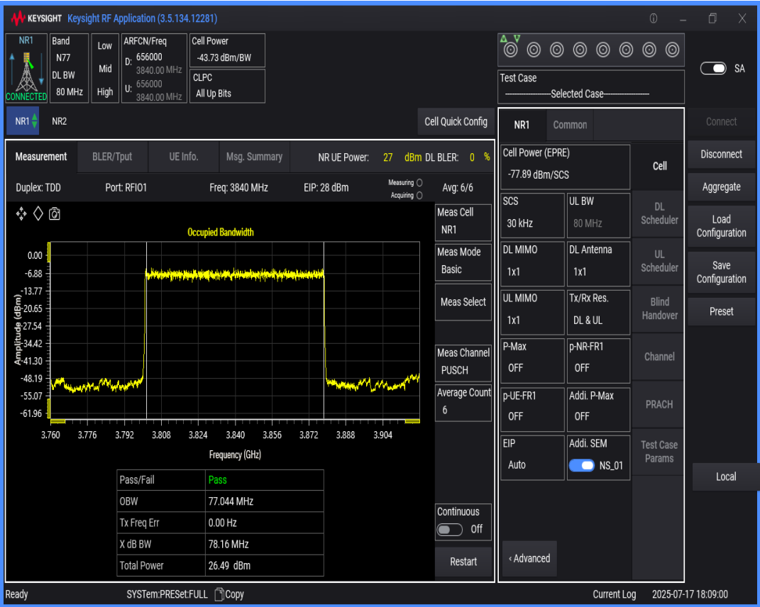
n77(3700-3980) SCS=30kHz DFT_BPSK BW=60MHz Channel=656000 RB=162@0
