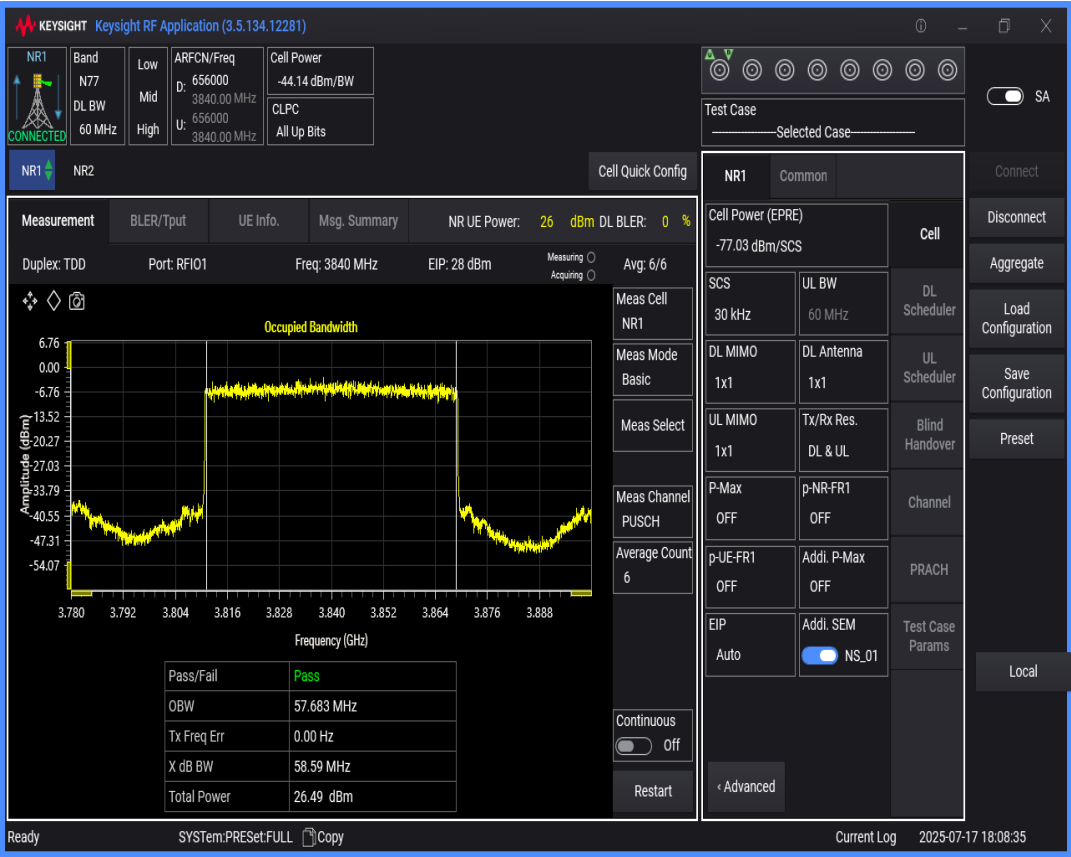
n77(3700-3980) SCS=30kHz DFT_QAM16 BW=10MHz Channel=656000 RB=24@0
