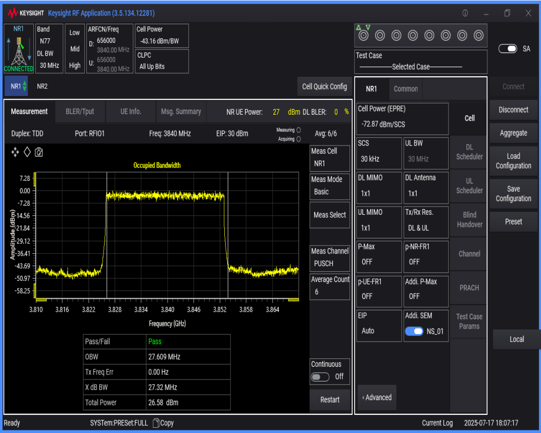
n77(3700-3980) SCS=30kHz DFT_BPSK BW=80MHz Channel=656000 RB=216@0
