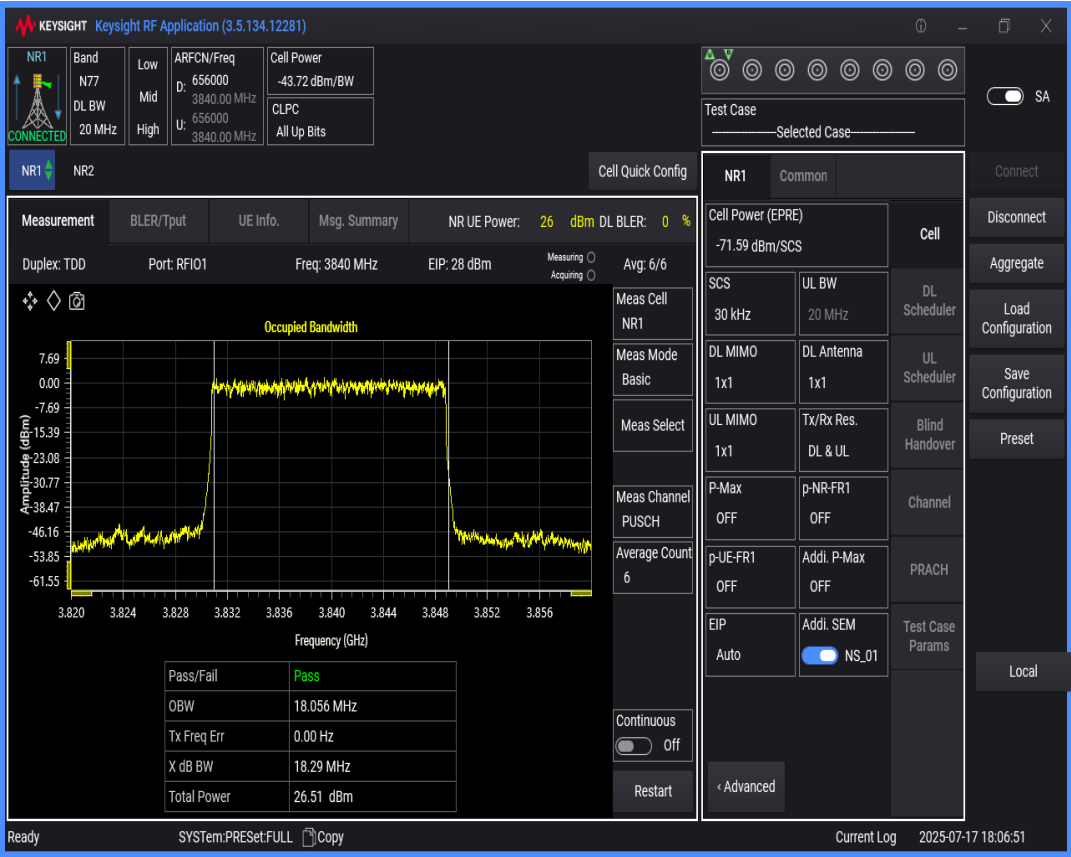
n77(3700-3980) SCS=30kHz DFT_BPSK BW=15MHz Channel=656000 RB=36@0
