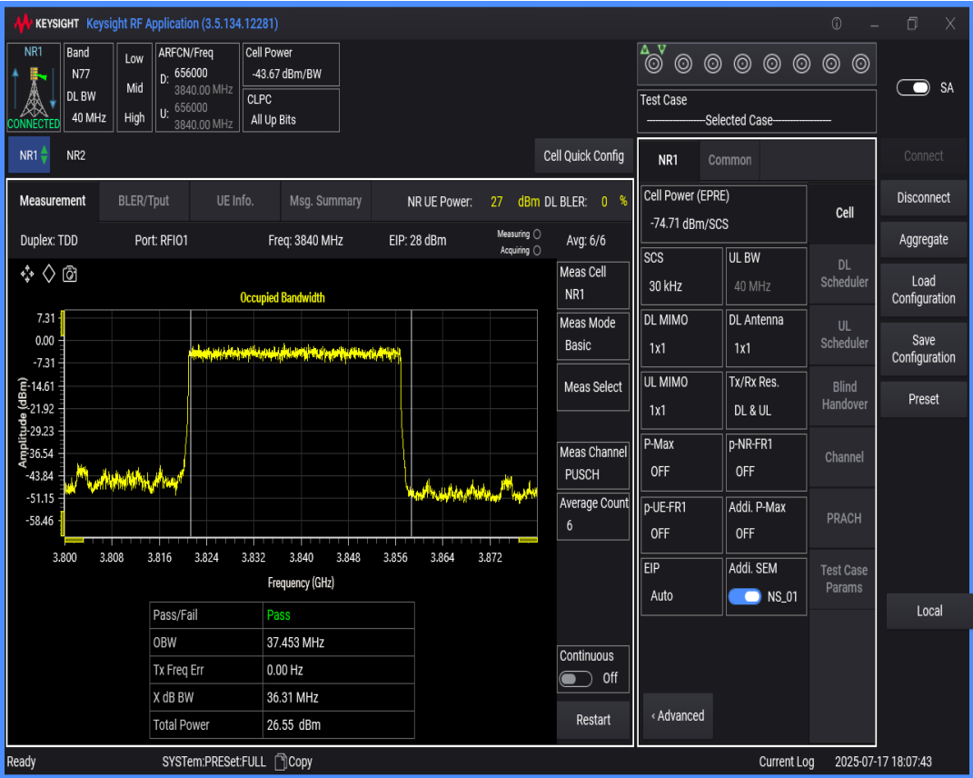
n77(3700-3980) SCS=30kHz DFT_BPSK BW=30MHz Channel=656000 RB=75@0
