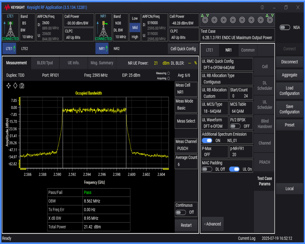
n38 SCS=30kHz DFT_QAM16 BW=15MHz Channel=519000 RB=36@0
