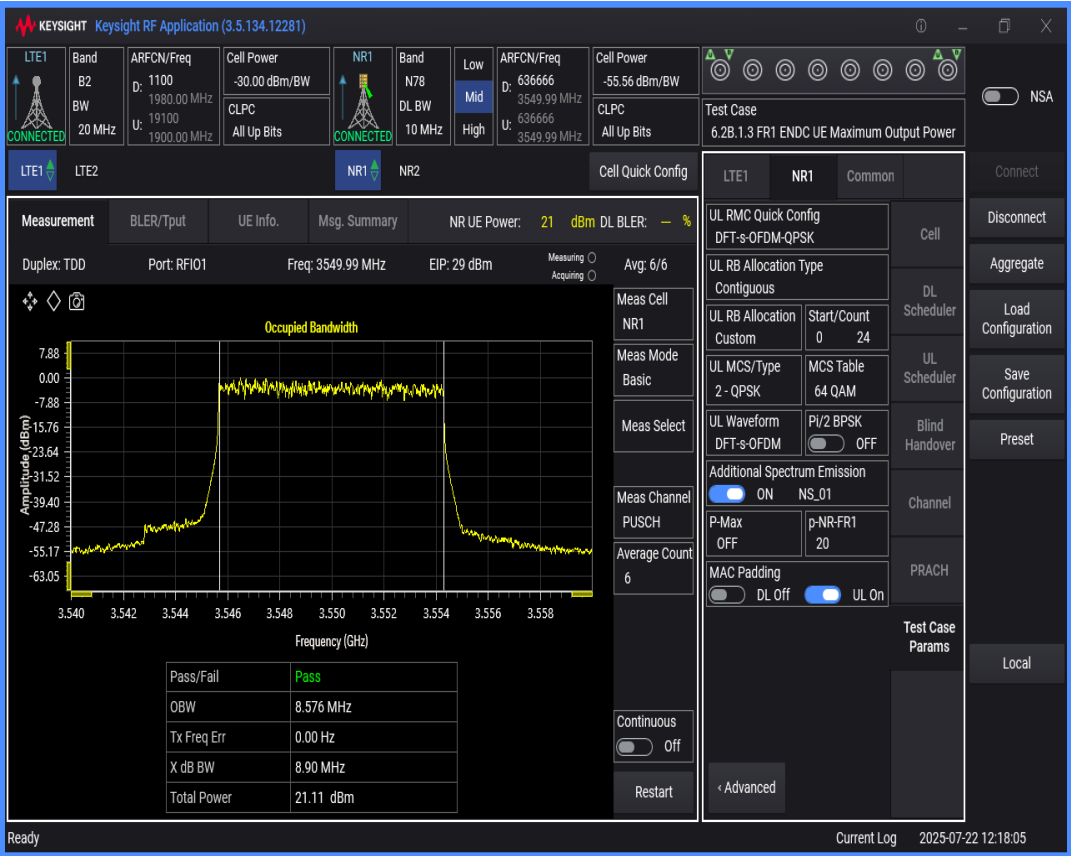
n78 SCS=30kHz DFT_QPSK BW=100MHz Channel=636666 RB=270@0
