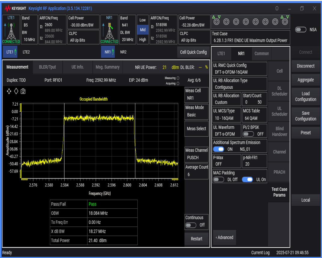
n41 SCS=30kHz DFT_BPSK BW=50MHz Channel=518598 RB=128@0
