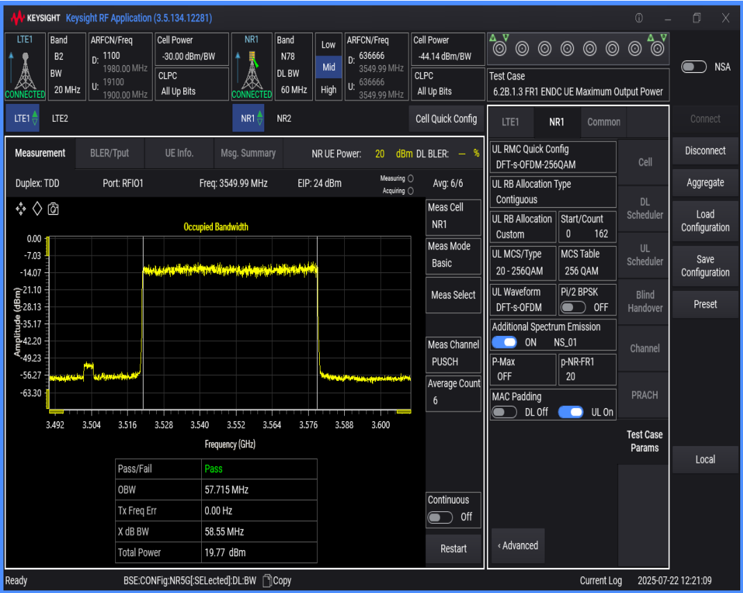
n78 SCS=30kHz DFT_QAM256 BW=10MHz Channel=636666 RB=24@0
