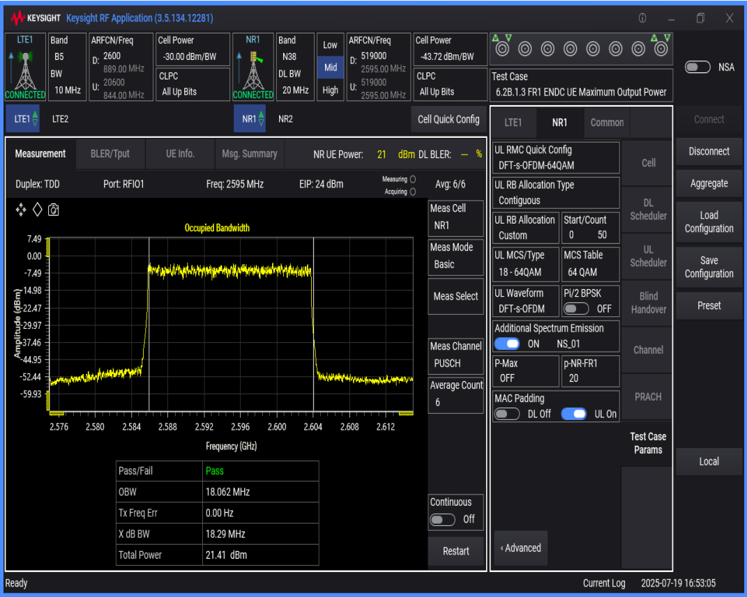
n38 SCS=30kHz DFT_QAM64 BW=15MHz Channel=519000 RB=36@0
