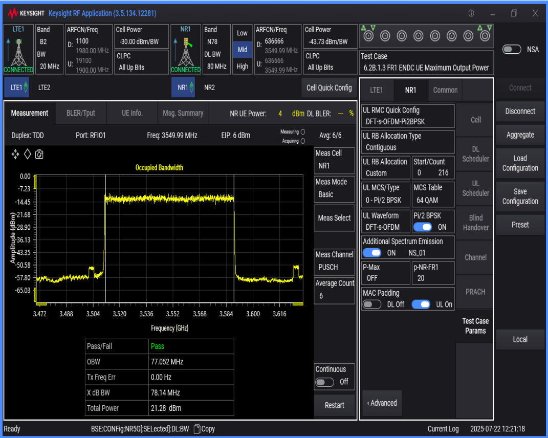
n78 SCS=30kHz DFT_BPSK BW=90MHz Channel=636666 RB=240@0
