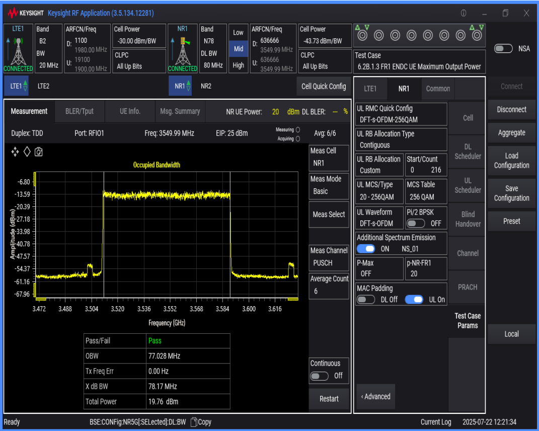
n78 SCS=30kHz DFT_QAM256 BW=40MHz Channel=636666 RB=100@0
