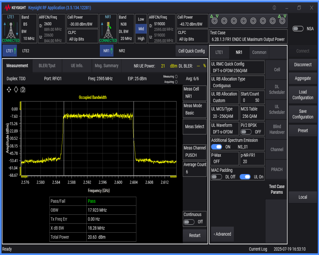
n38 SCS=30kHz DFT_QAM64 BW=10MHz Channel=519000 RB=24@0
