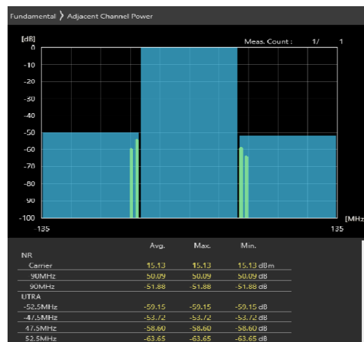
90MHz_30kHz_3655MHz-OFDM QPSK_RB120@60 -52.97,-54.22dB
