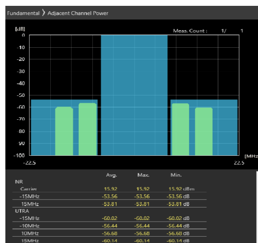
15MHz_30kHz_3692.5MHz-OFDM QPSK_RB36@0 -53.09,-53.12dB
