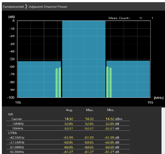
70MHz_30kHz_3585MHz-OFDM QPSK_RB90@45 -53.58,-54.62dB
