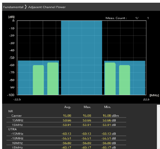
15MHz_30kHz_3557.5MHz-OFDM QPSK_RB36@0 -52.51,-52.67dB
