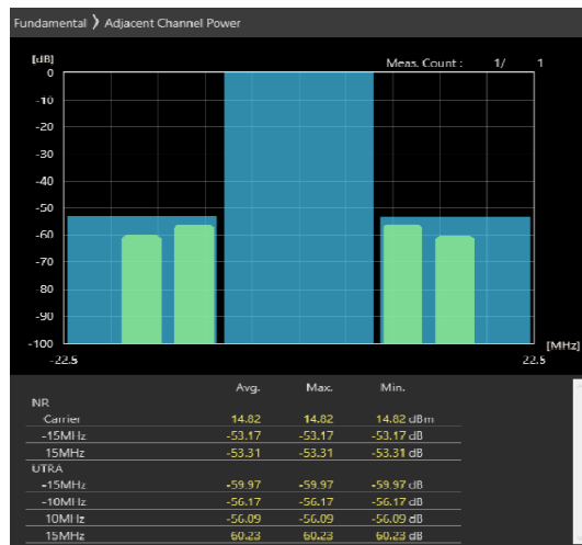
15MHz_30kHz_3692.5MHz-OFDM QPSK_RB36@0 -53.17,-53.31dB
