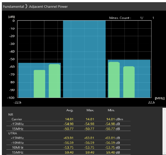
15MHz_30kHz_3692.5MHz-OFDM QPSK_RB1@37 -54.98,-50.77dB
