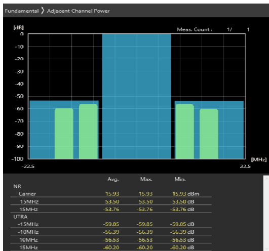
15MHz_30kHz_3557.5MHz-OFDM QPSK_RB36@0 -53.04,-53.07dB
