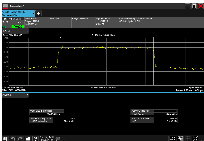
n78_2_90MHz_30kHz_3625MHz_DFT-s-OFDM 256 QAM_RB243@0 86.412MHz
