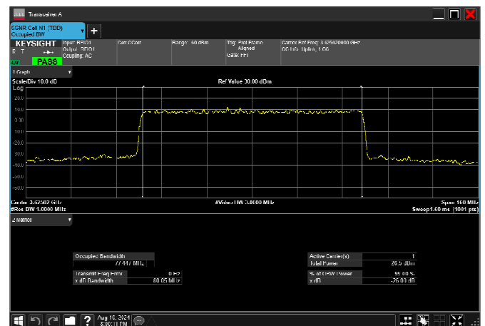
n78_2_80MHz_30kHz_3625MHz_CP-OFDM 256 QAM_RB217@0 77.447MHz
