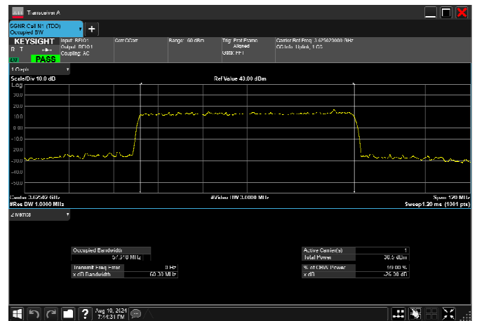
n78_2_60MHz_30kHz_3625MHz_DFT-s-OFDM 16 QAM_RB162@0 57.618MHz
