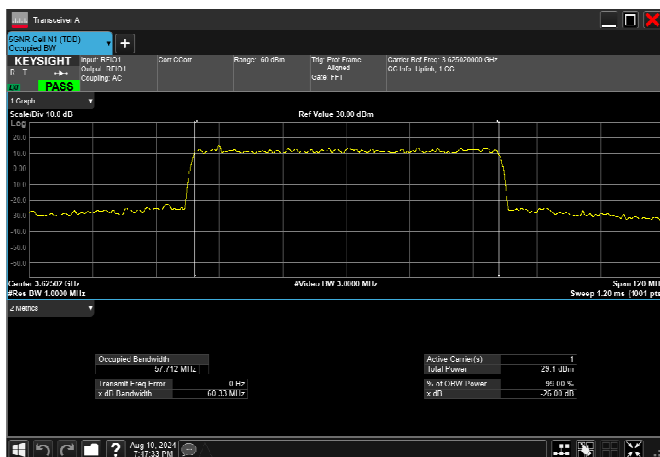
n78_2_60MHz_30kHz_3625MHz_CP-OFDM 64 QAM_RB162@0 57.712MHz
