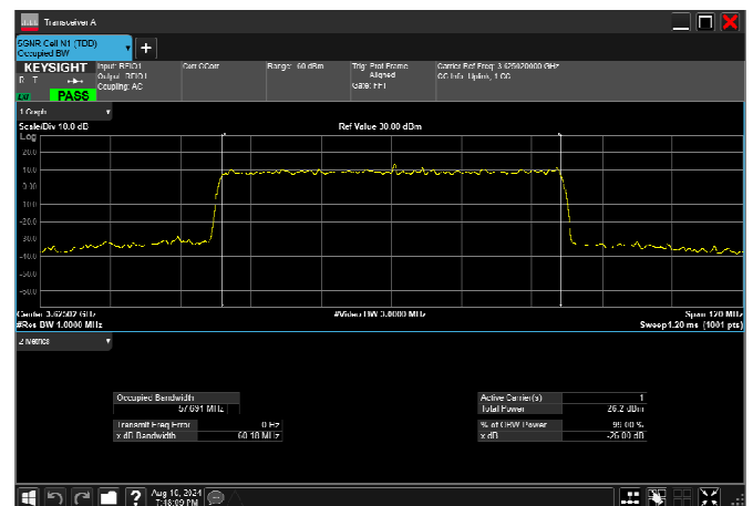
n78_2_60MHz_30kHz_3625MHz_CP-OFDM 256 QAM_RB162@0 57.691MHz
