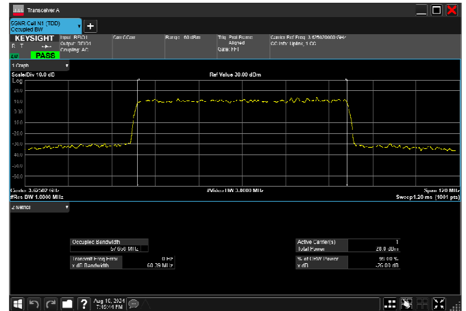
n78_2_60MHz_30kHz_3625MHz_CP-OFDM 16 QAM_RB162@0 57.712MHz
