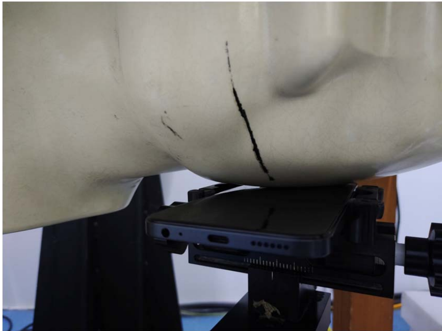
Head Left Tilt Setup Photo (0mm)
