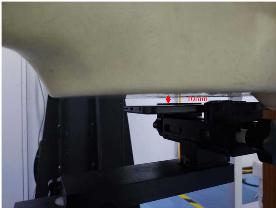
Body(Wron) Back Setup Photo (10mm)
