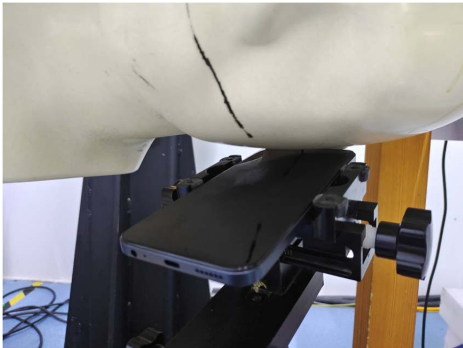
Head Left Tilt Setup Photo (0mm)
