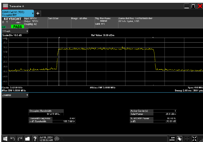
n78_2_100MHz_30kHz_3625MHz_CP-OFDM 64 QAM_RB273@0 97.279MHz
