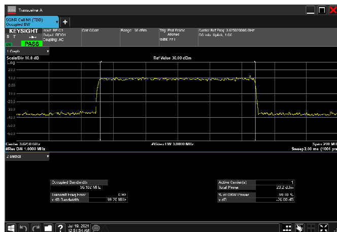
n78_2_100MHz_30kHz_3625MHz_DFT-s-OFDM 16 QAM_RB270@0 96.102MHz
