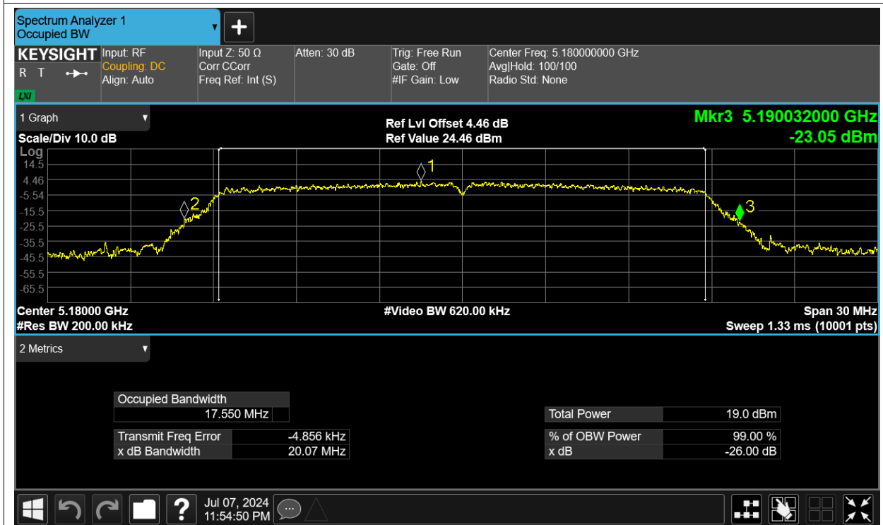
-26dB Bandwidth NVNT n20 5200MHz Ant2
