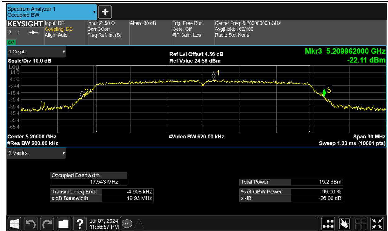
-26dB Bandwidth NVNT n20 5240MHz Ant2
