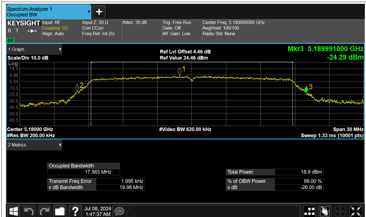
-26dB Bandwidth NVNT ac20 5200MHz Ant2
