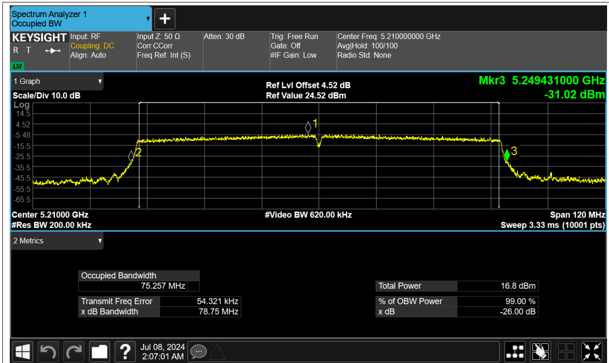
-26dB Bandwidth NVNT n20 5180MHz Ant2
