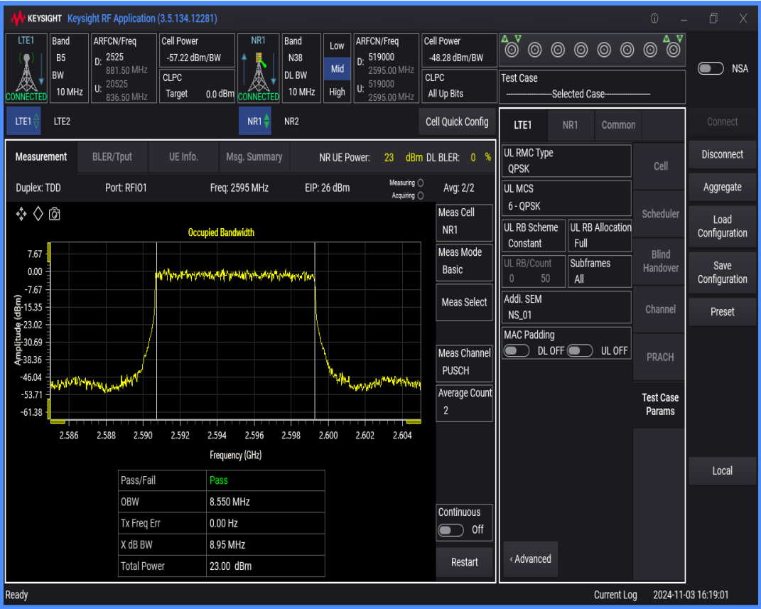
n38 SCS=30kHz DFT_QAM16 BW=10MHz Channel=519000 RB=24@0
