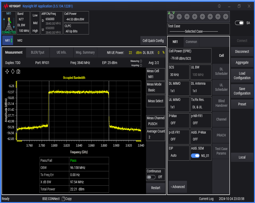
n77(3700-3980) SCS=30kHz DFT_QAM256 BW=100MHz Channel=656000 RB=270@0
