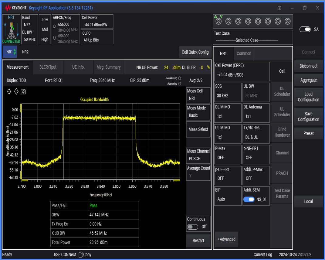
n77(3700-3980) SCS=30kHz DFT_QPSK BW=50MHz Channel=656000 RB=128@0
