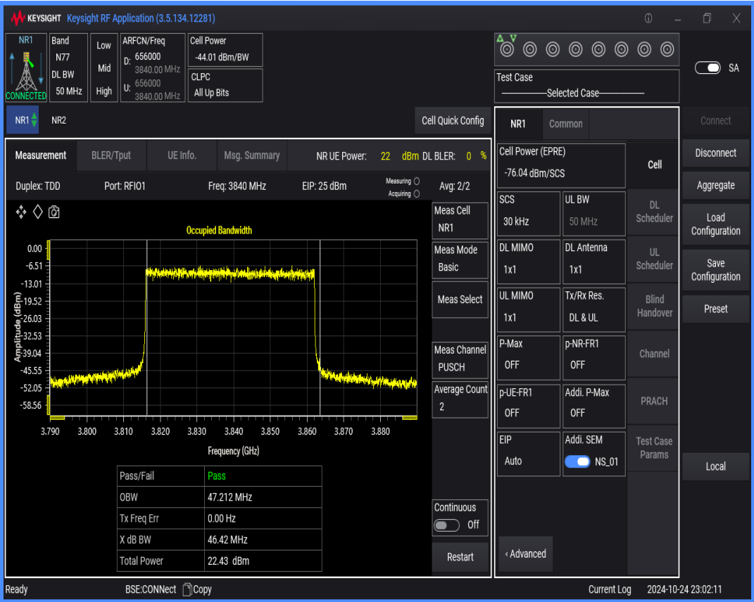
n77(3700-3980) SCS=30kHz DFT_QAM64 BW=50MHz Channel=656000 RB=128@0
