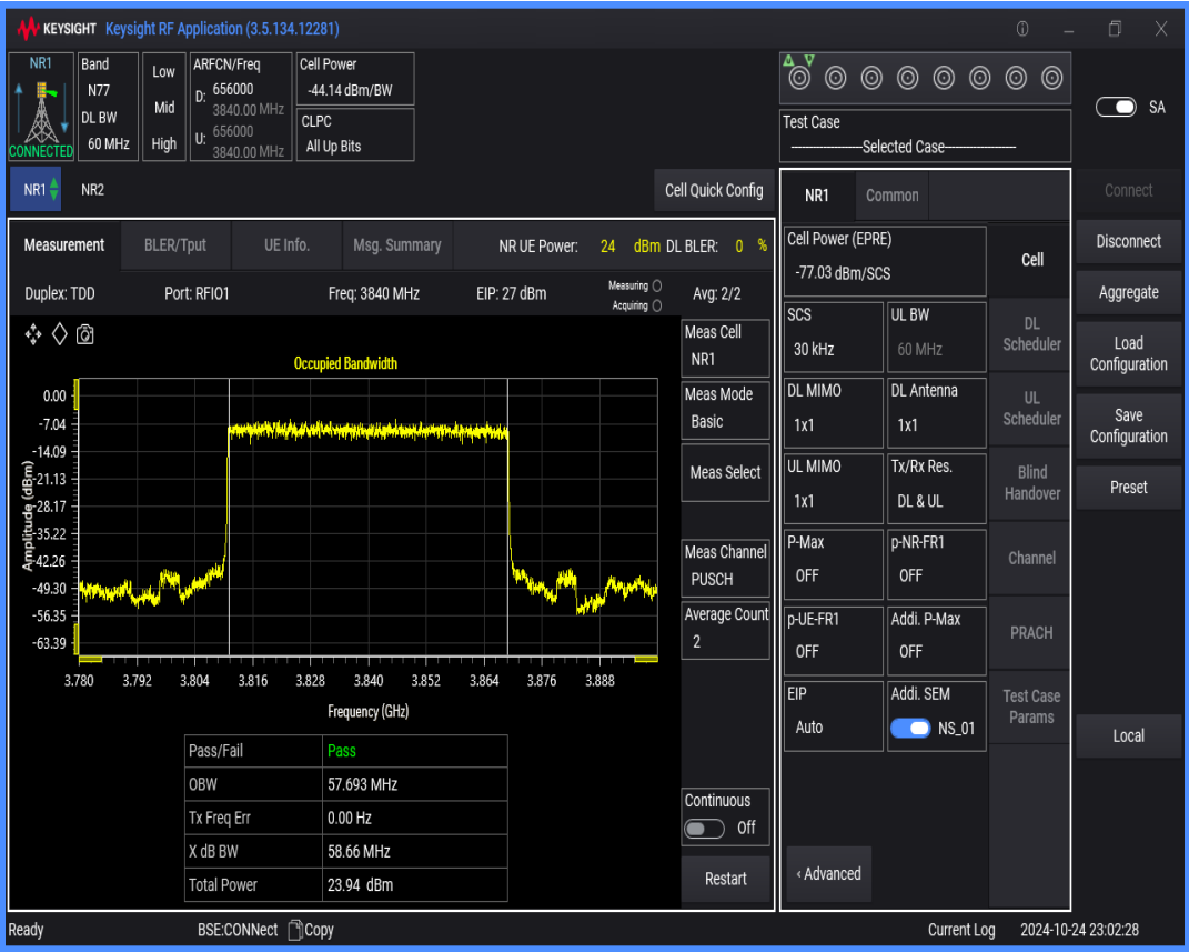
n77(3700-3980) SCS=30kHz DFT_QAM16 BW=60MHz Channel=656000 RB=162@0
