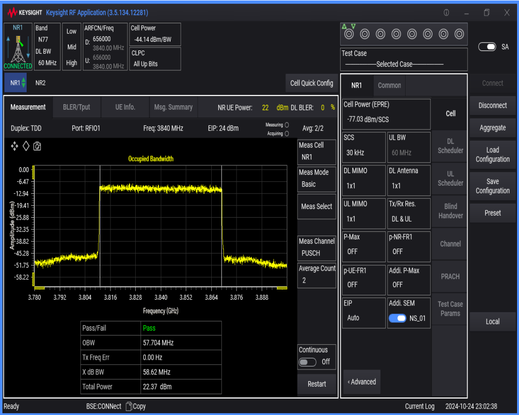
n77(3700-3980) SCS=30kHz DFT_QPSK BW=60MHz Channel=656000 RB=162@0
