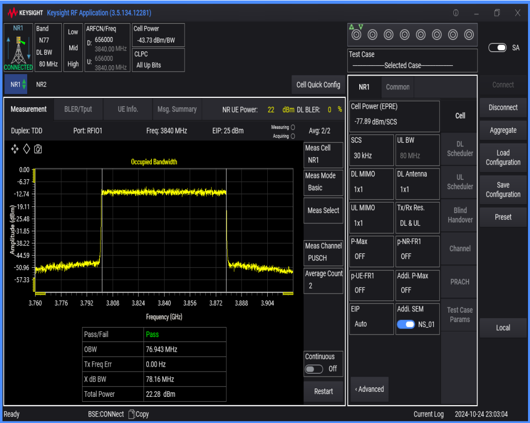
n77(3700-3980) SCS=30kHz DFT_QAM64 BW=80MHz Channel=656000 RB=216@0
