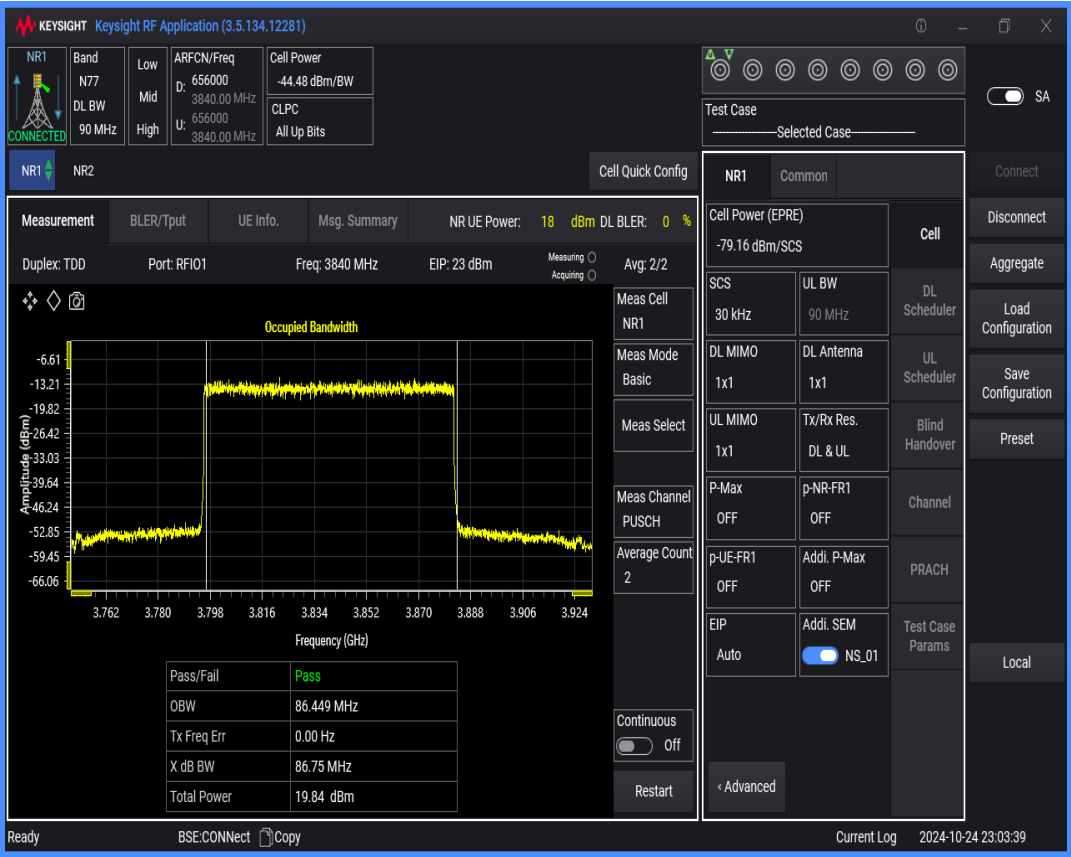
n77(3700-3980) SCS=30kHz DFT_BPSK BW=100MHz Channel=656000 RB=270@0
