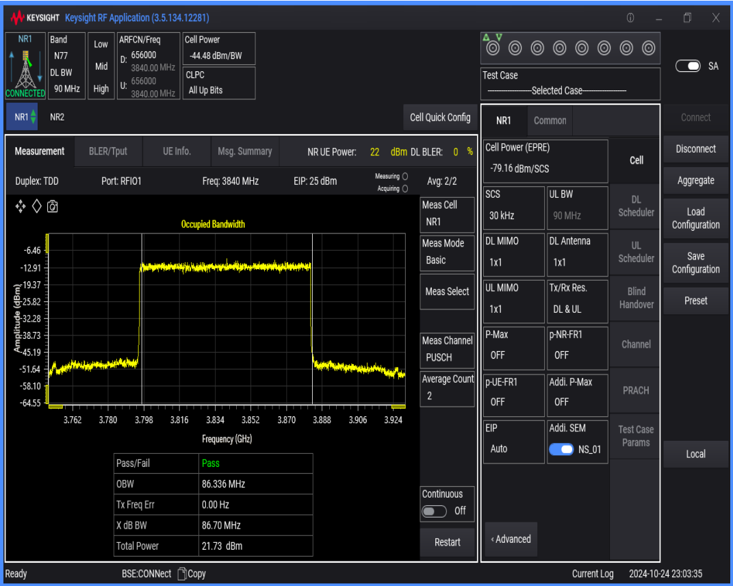
n77(3700-3980) SCS=30kHz DFT_QAM256 BW=90MHz Channel=656000 RB=240@0
