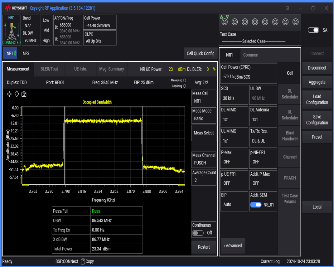
n77(3700-3980) SCS=30kHz DFT_QAM16 BW=90MHz Channel=656000 RB=240@0
