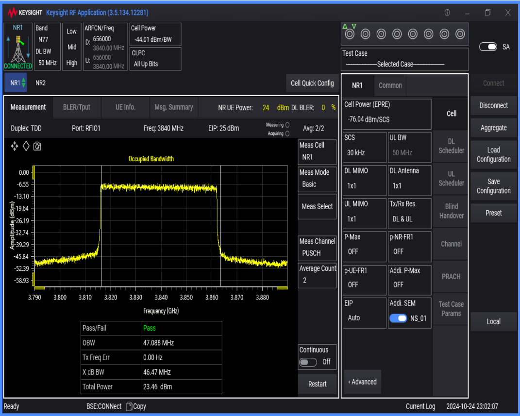
n77(3700-3980) SCS=30kHz DFT_QAM16 BW=50MHz Channel=656000 RB=128@0
