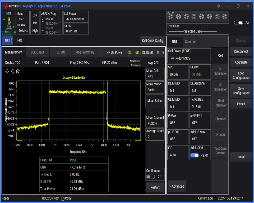
n77(3700-3980) SCS=30kHz DFT_QAM256 BW=50MHz Channel=656000 RB=128@0
