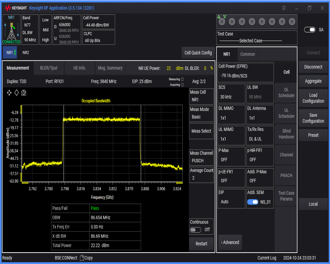
n77(3700-3980) SCS=30kHz DFT_QAM64 BW=90MHz Channel=656000 RB=240@0
