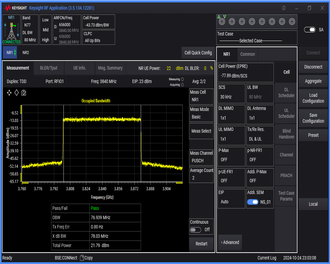
n77(3700-3980) SCS=30kHz DFT_BPSK BW=90MHz Channel=656000 RB=240@0
