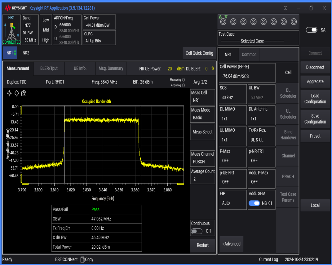
n77(3700-3980) SCS=30kHz DFT_BPSK BW=60MHz Channel=656000 RB=162@0
