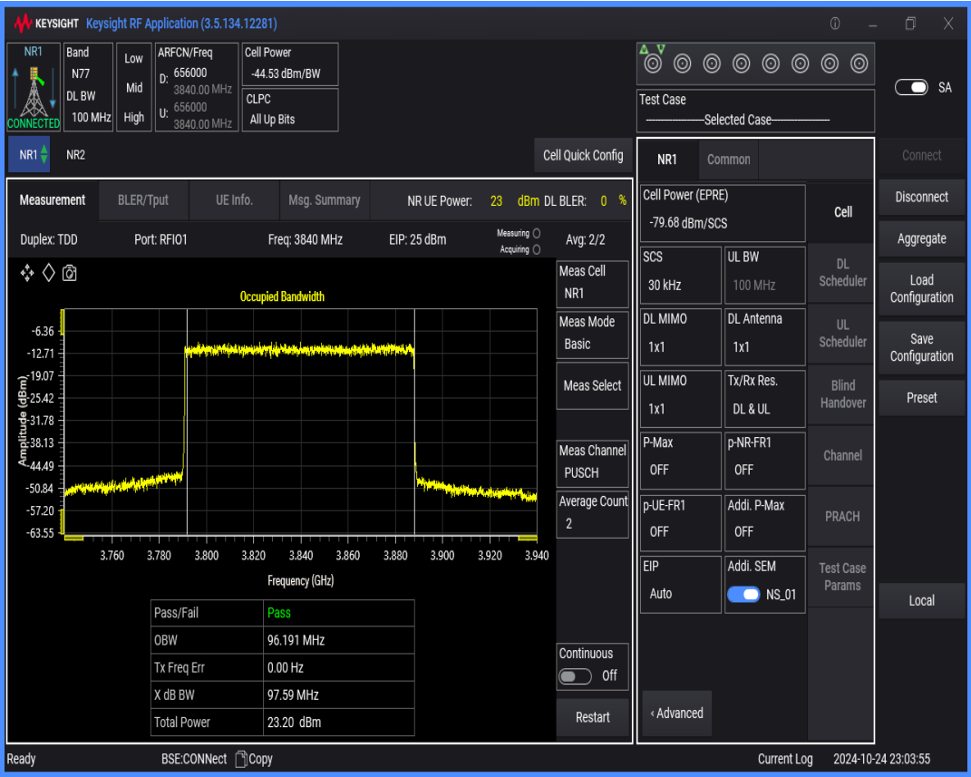
n77(3700-3980) SCS=30kHz DFT_QAM16 BW=100MHz Channel=656000 RB=270@0
