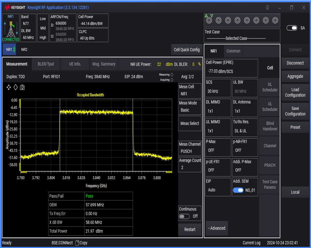
n77(3700-3980) SCS=30kHz DFT_QAM256 BW=60MHz Channel=656000 RB=162@0
