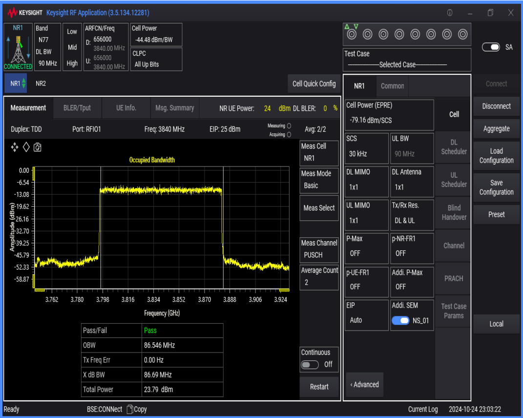
n77(3700-3980) SCS=30kHz DFT_QAM256 BW=80MHz Channel=656000 RB=216@0
