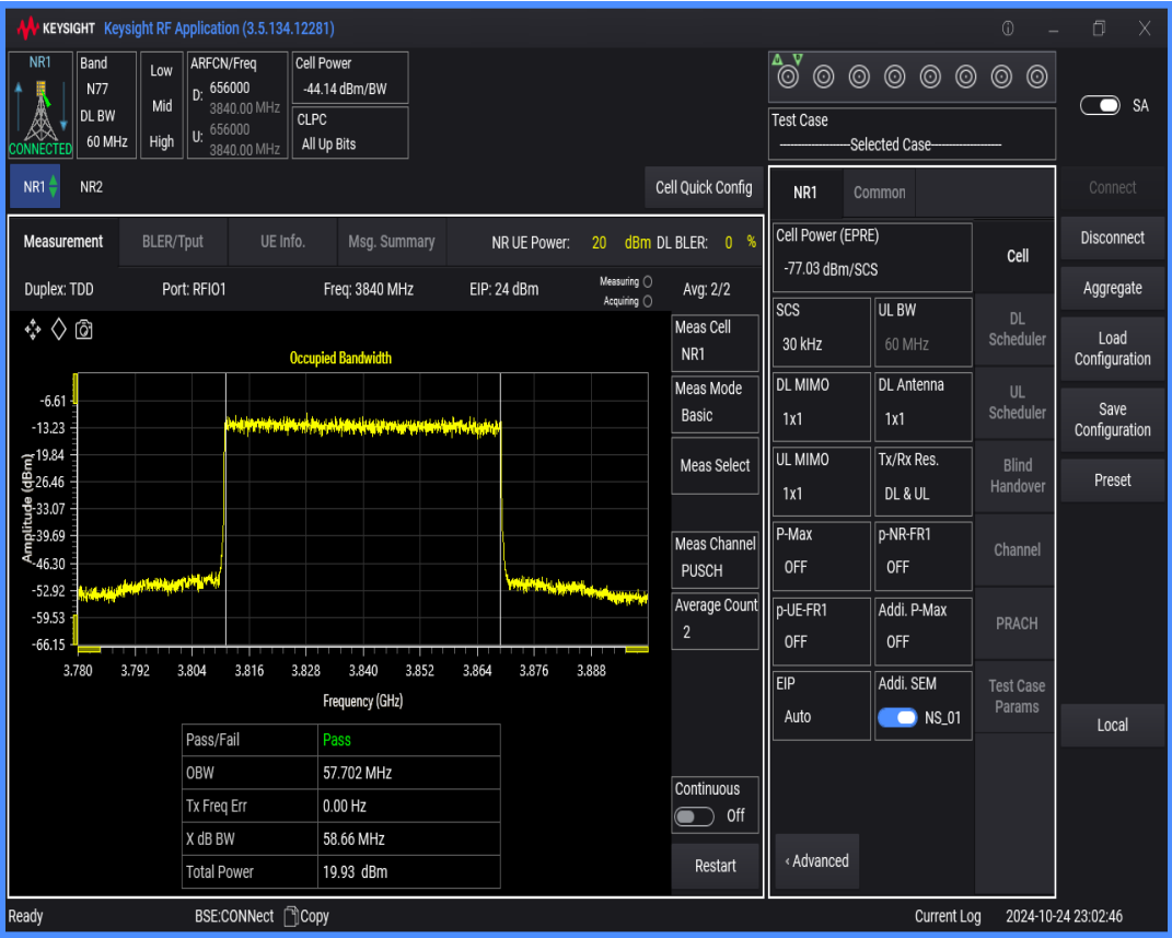
n77(3700-3980) SCS=30kHz DFT_BPSK BW=80MHz Channel=656000 RB=216@0
