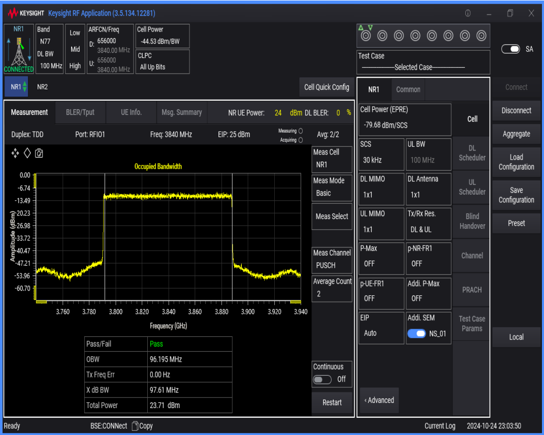
n77(3700-3980) SCS=30kHz DFT_QPSK BW=100MHz Channel=656000 RB=270@0
