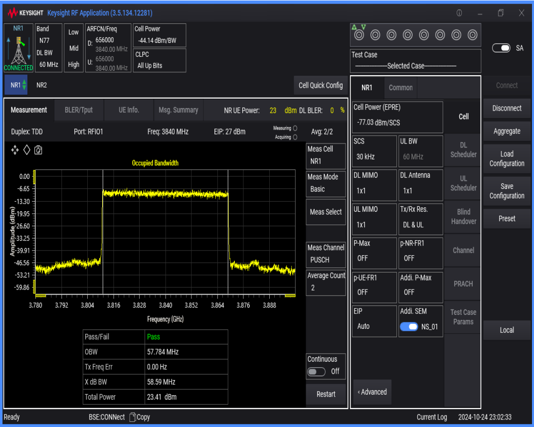
n77(3700-3980) SCS=30kHz DFT_QAM64 BW=60MHz Channel=656000 RB=162@0
