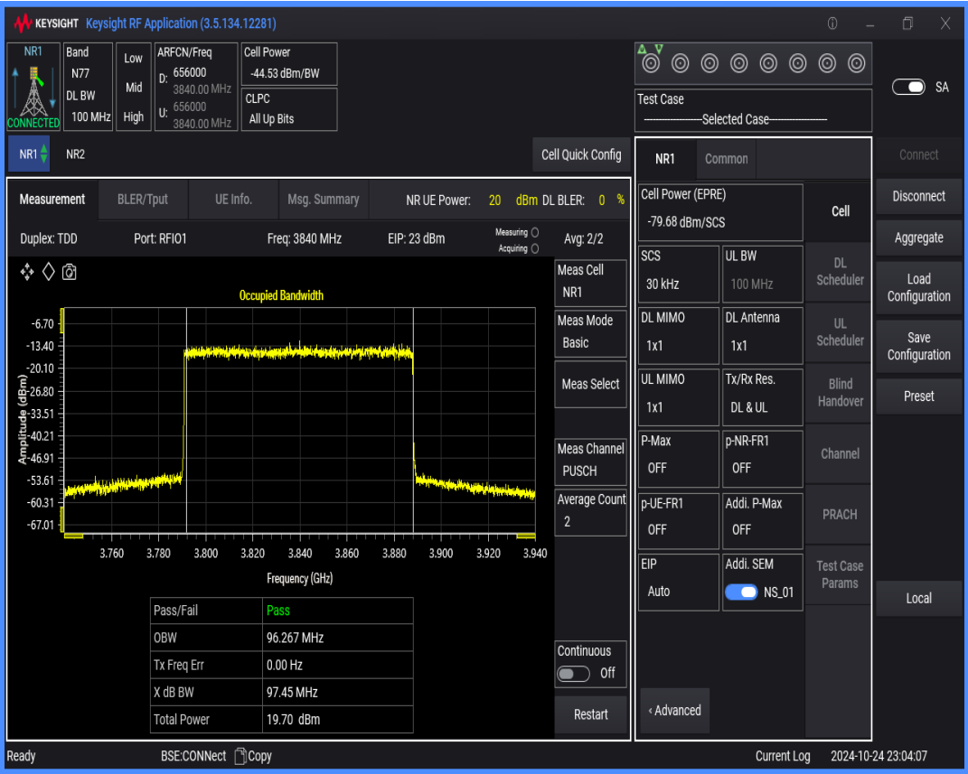
n77(3700-3980) SCS=30kHz DFT_QAM64 BW=100MHz Channel=656000 RB=270@0
