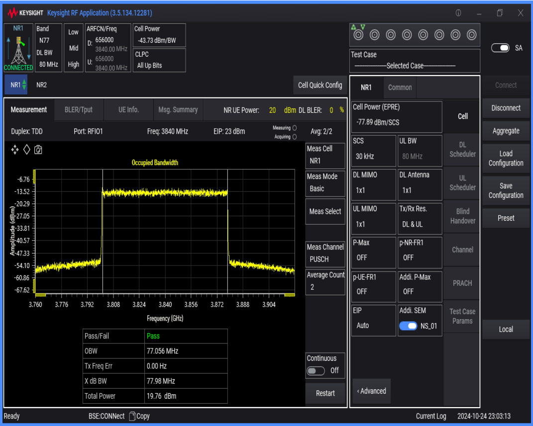
n77(3700-3980) SCS=30kHz DFT_QPSK BW=90MHz Channel=656000 RB=240@0
