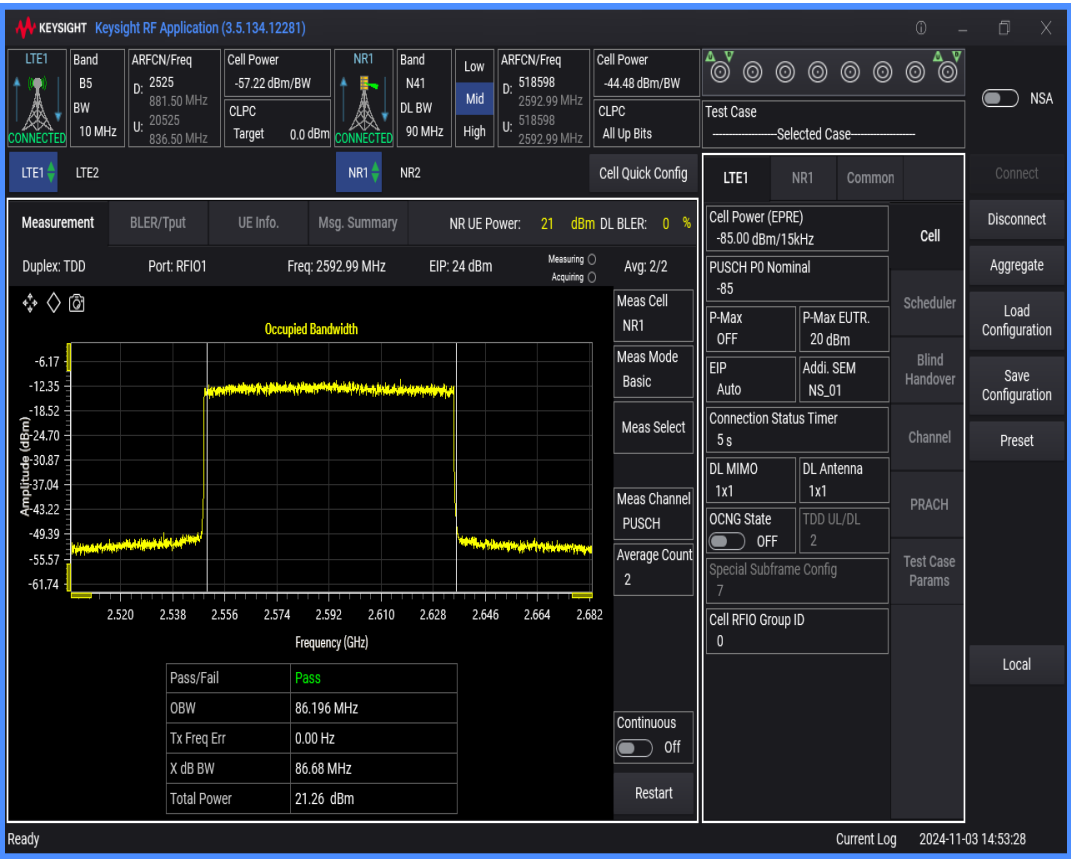
n41 SCS=30kHz DFT_QPSK BW=100MHz Channel=518598 RB=270@0
