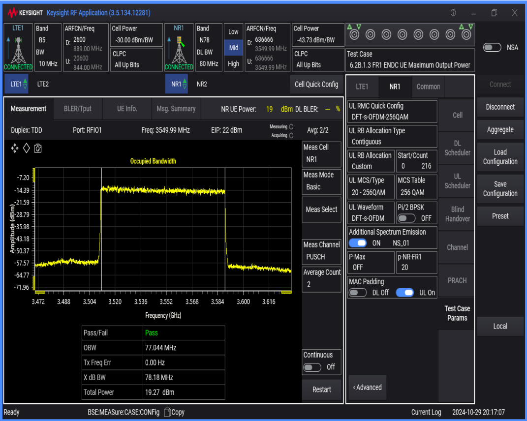
n78 SCS=30kHz DFT_QPSK BW=15MHz Channel=636666 RB=36@0
