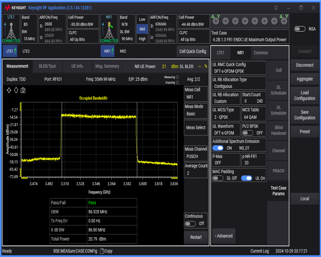
n78 SCS=30kHz DFT_QPSK BW=80MHz Channel=636666 RB=216@0
