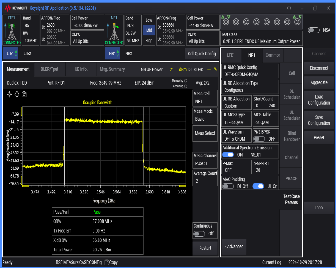
n78 SCS=30kHz DFT_QPSK BW=90MHz Channel=636666 RB=240@0
