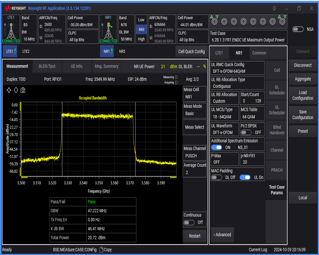
n78 SCS=30kHz DFT_QAM64 BW=80MHz Channel=636666 RB=216@0
