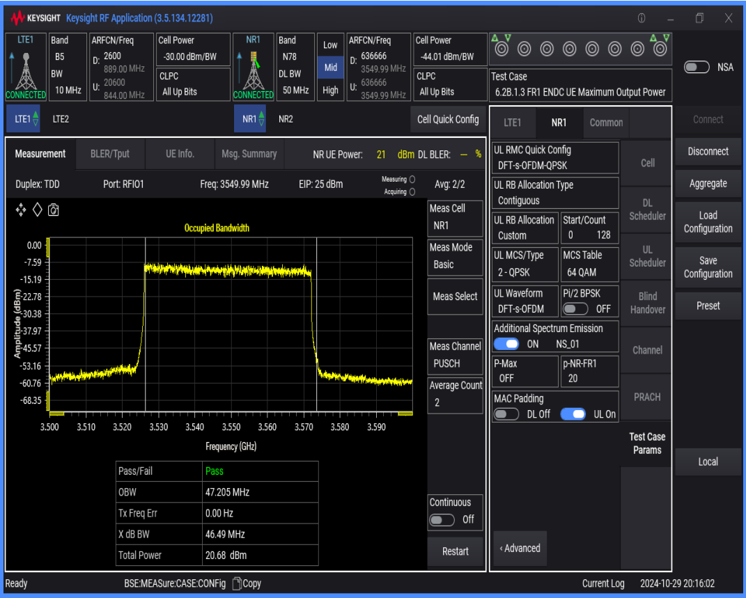
n78 SCS=30kHz DFT_QPSK BW=40MHz Channel=636666 RB=100@0
