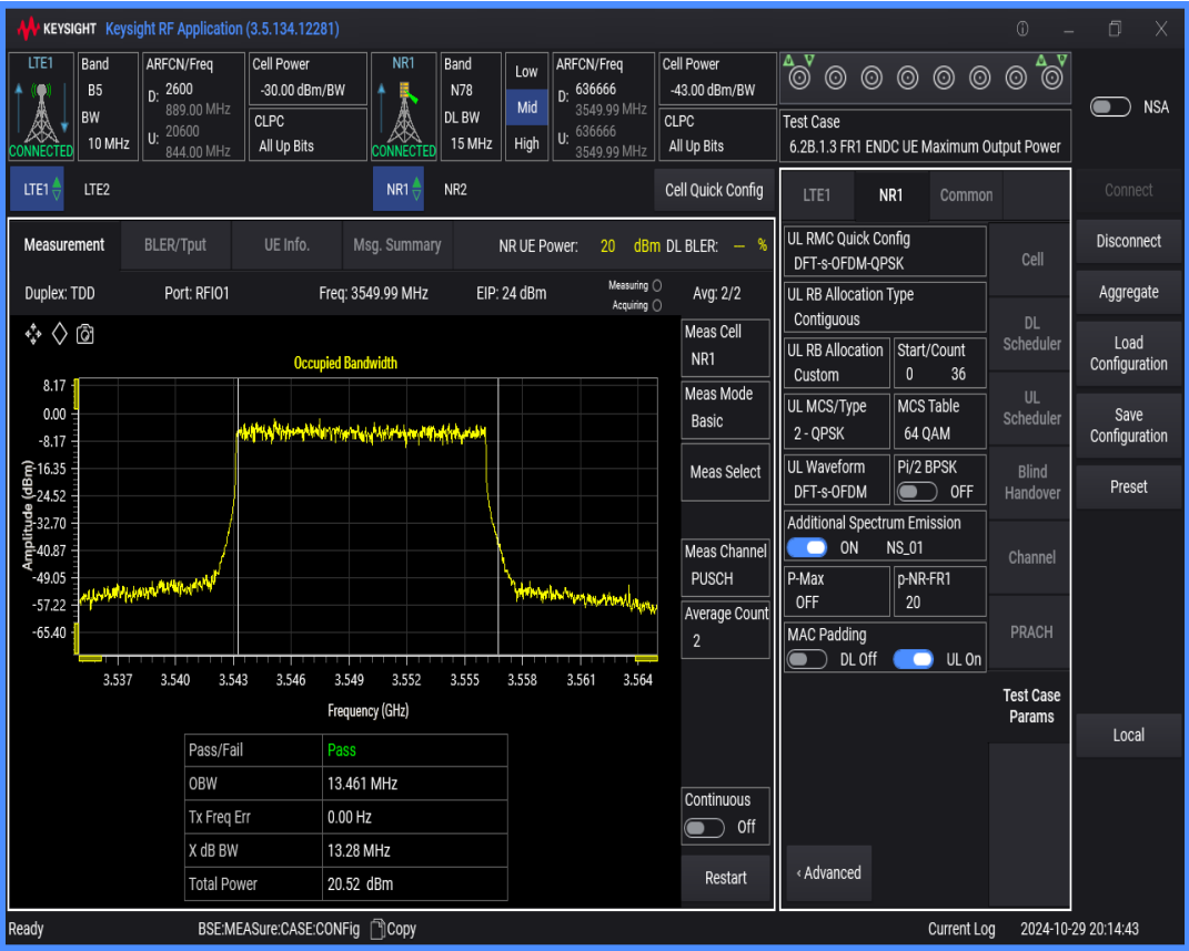
n78 SCS=30kHz DFT_QPSK BW=10MHz Channel=636666 RB=24@0
