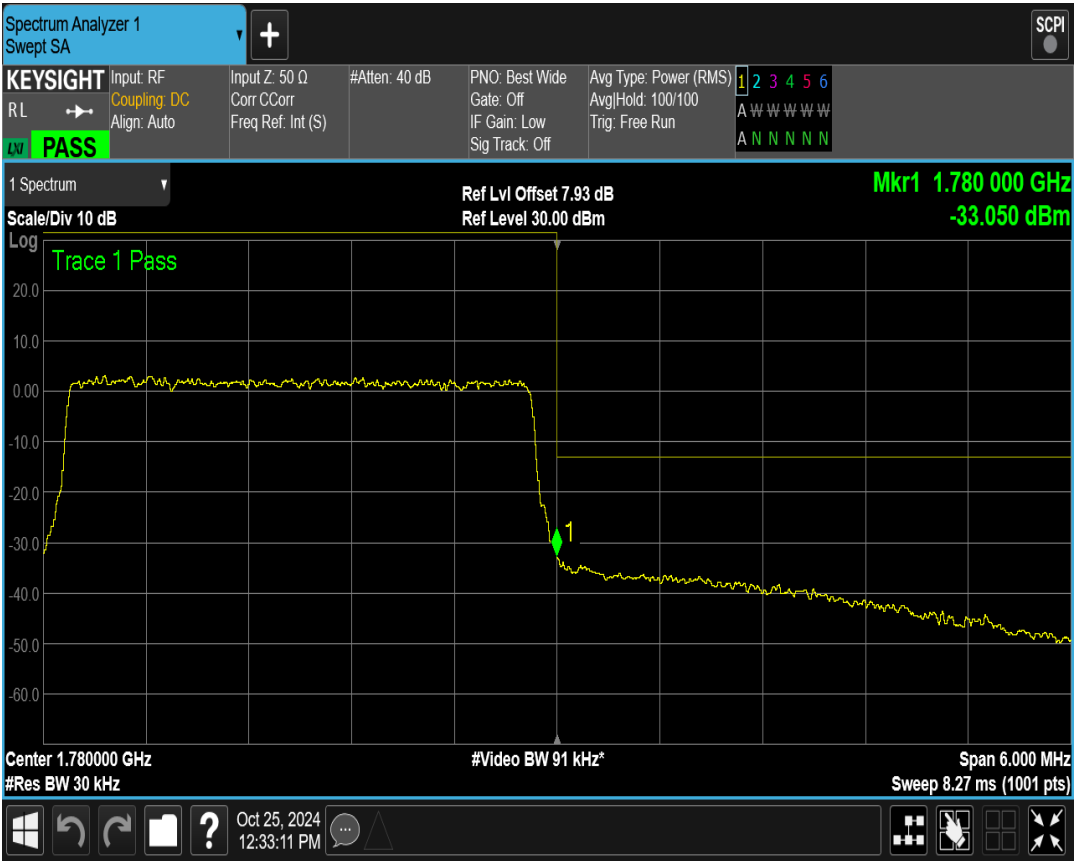
Band66 QPSK BW=1.4MHz Channel=131979 RB Size=6 Position=#0
