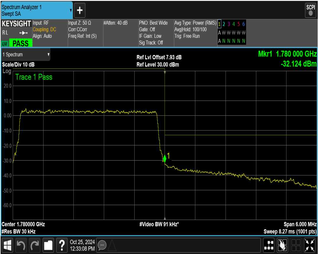
Band66 QPSK BW=5MHz Channel=131997 RB Size=25 Position=#0
