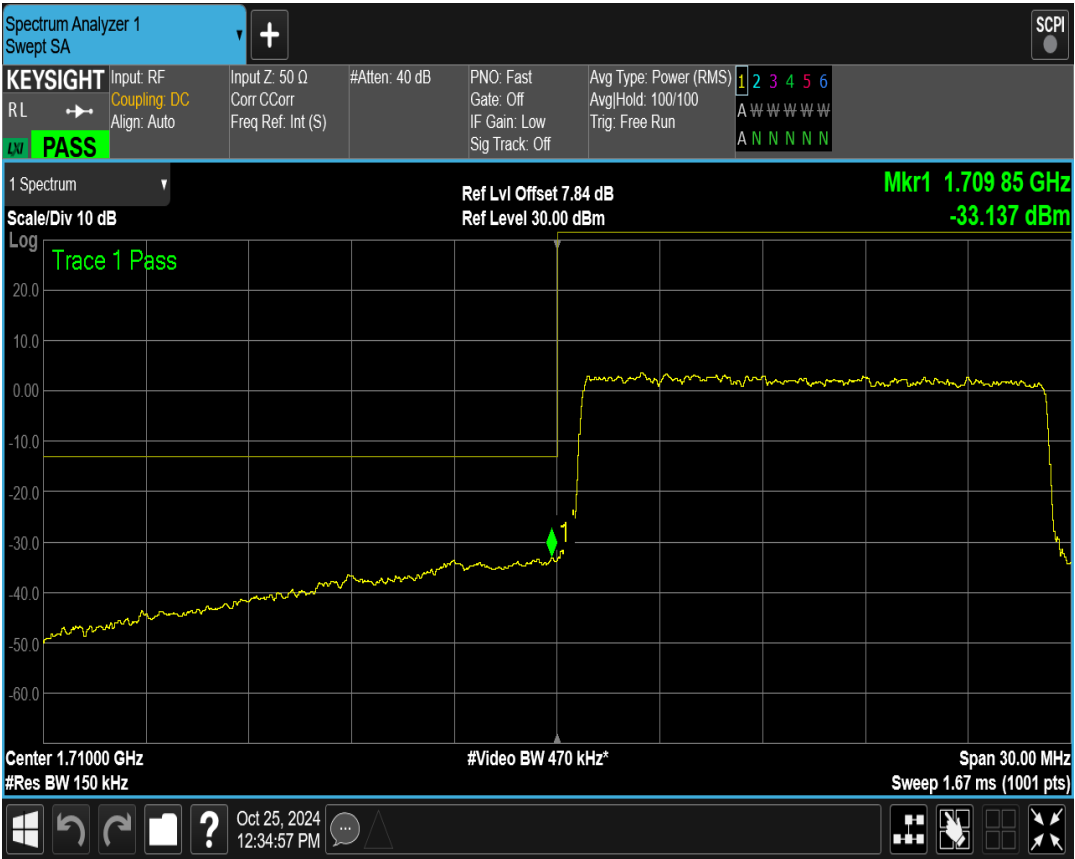
Band66 QAM16 BW=15MHz Channel=132597 RB Size=75 Position=#0
