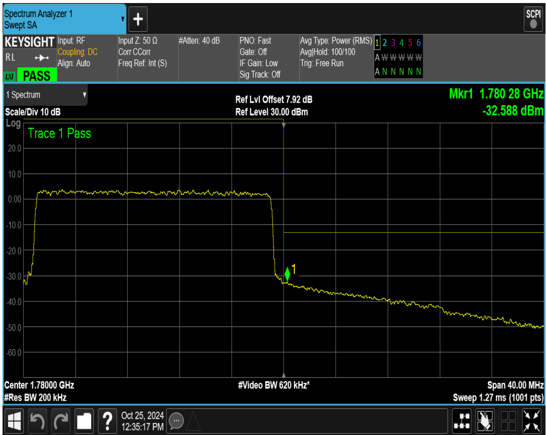
Band66 QPSK BW=3MHz Channel=131987 RB Size=15 Position=#0
