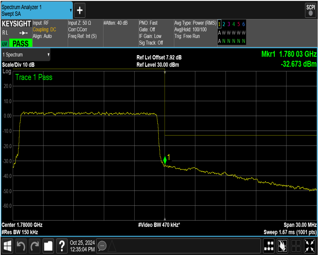
Band66 QAM16 BW=5MHz Channel=131997 RB Size=25 Position=#0
