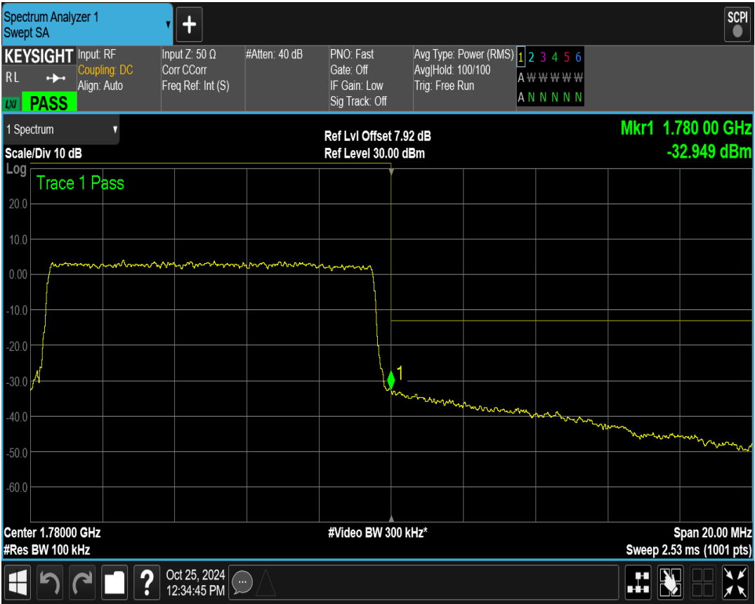
Band66 QPSK BW=3MHz Channel=132657 RB Size=15 Position=#0
