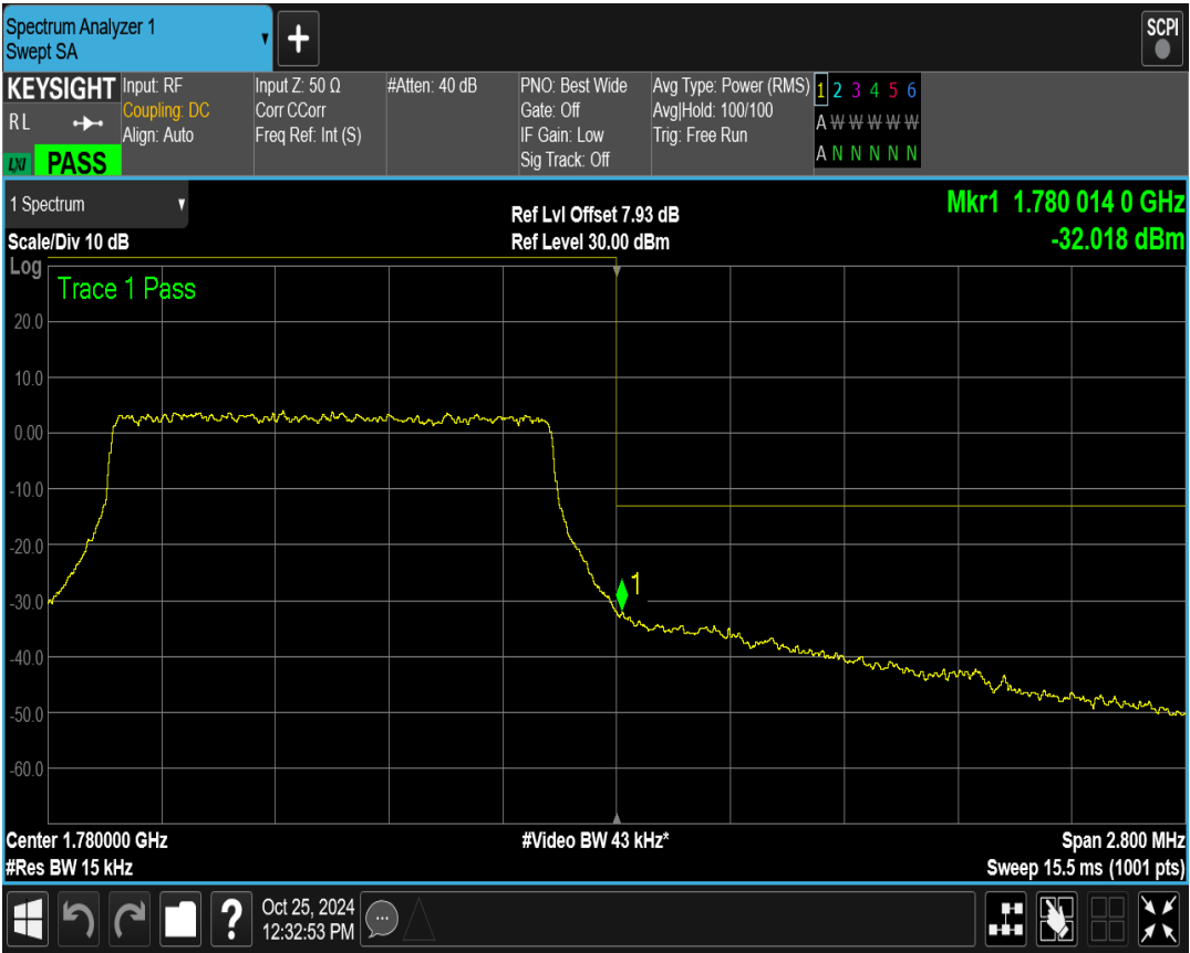
Band66 QAM16 BW=1.4MHz Channel=131979 RB Size=6 Position=#0
