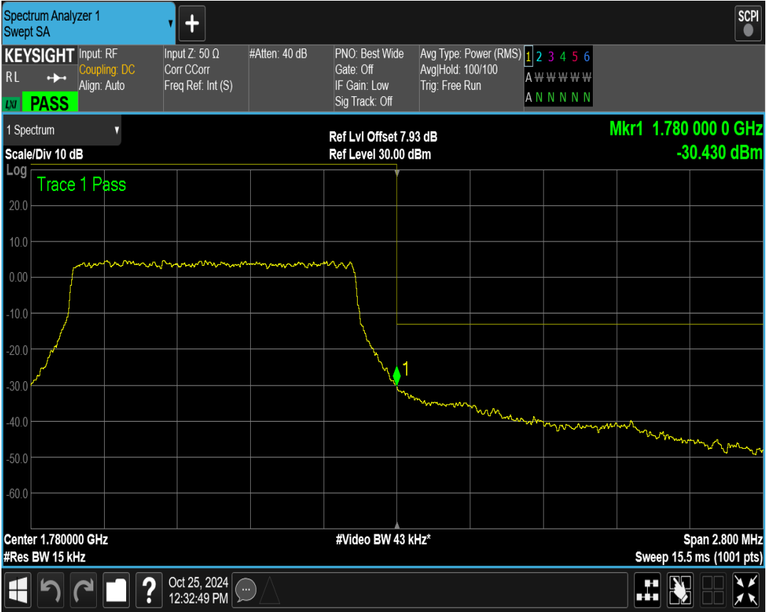
Band66 QPSK BW=10MHz Channel=132022 RB Size=50 Position=#0
