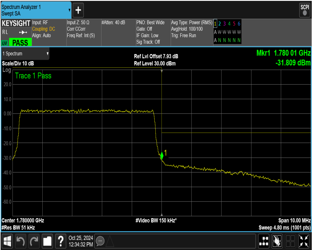
Band66 QPSK BW=15MHz Channel=132047 RB Size=75 Position=#0
