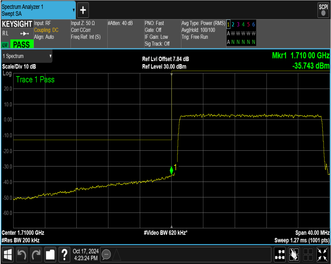
Band4 QPSK BW=20MHz Channel=20300 RB Size=100 Position=#0
