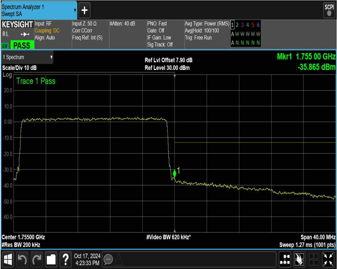
Band4 QAM16 BW=3MHz Channel=19965 RB Size=15 Position=#0
