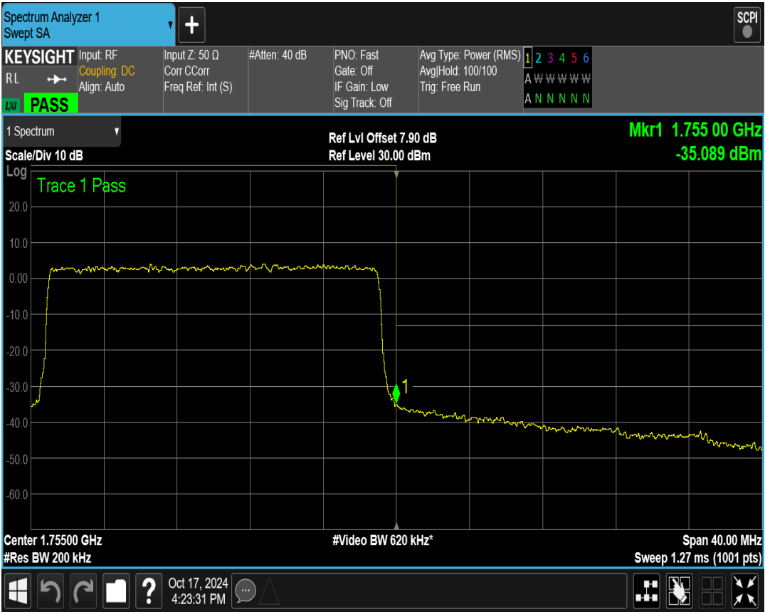
Band4 QPSK BW=20MHz Channel=20300 RB Size=100 Position=#0
