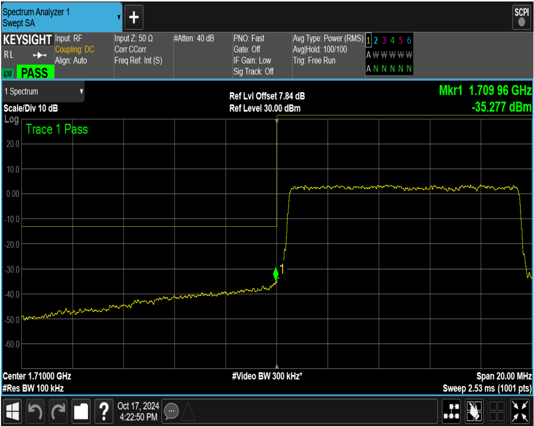
Band4 QPSK BW=1.4MHz Channel=20393 RB Size=6 Position=#0
