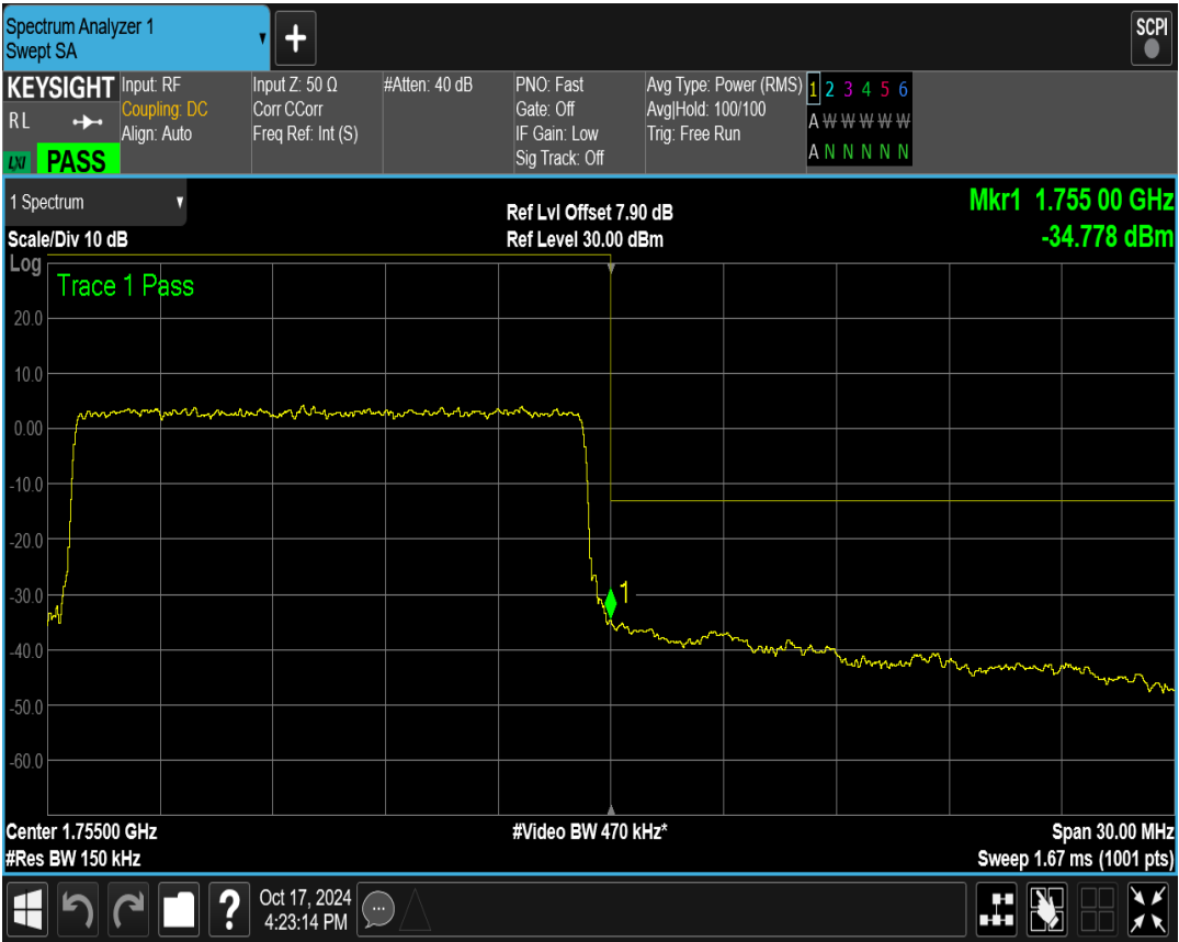
Band4 QPSK BW=20MHz Channel=20050 RB Size=100 Position=#0
