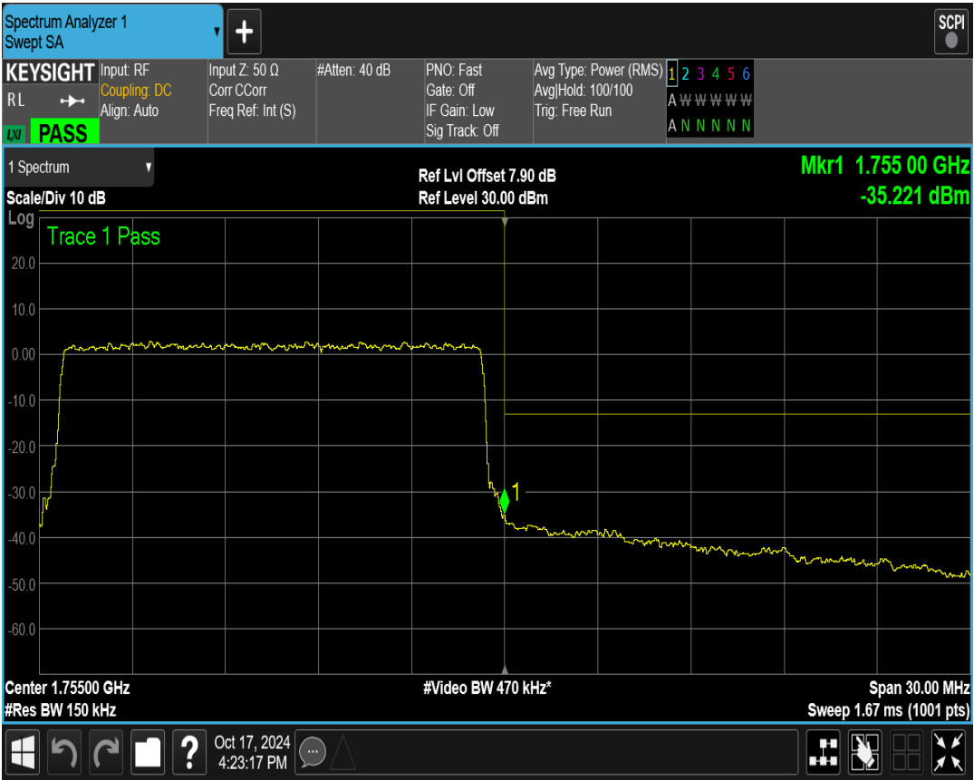
Band4 QPSK BW=10MHz Channel=20000 RB Size=50 Position=#0
