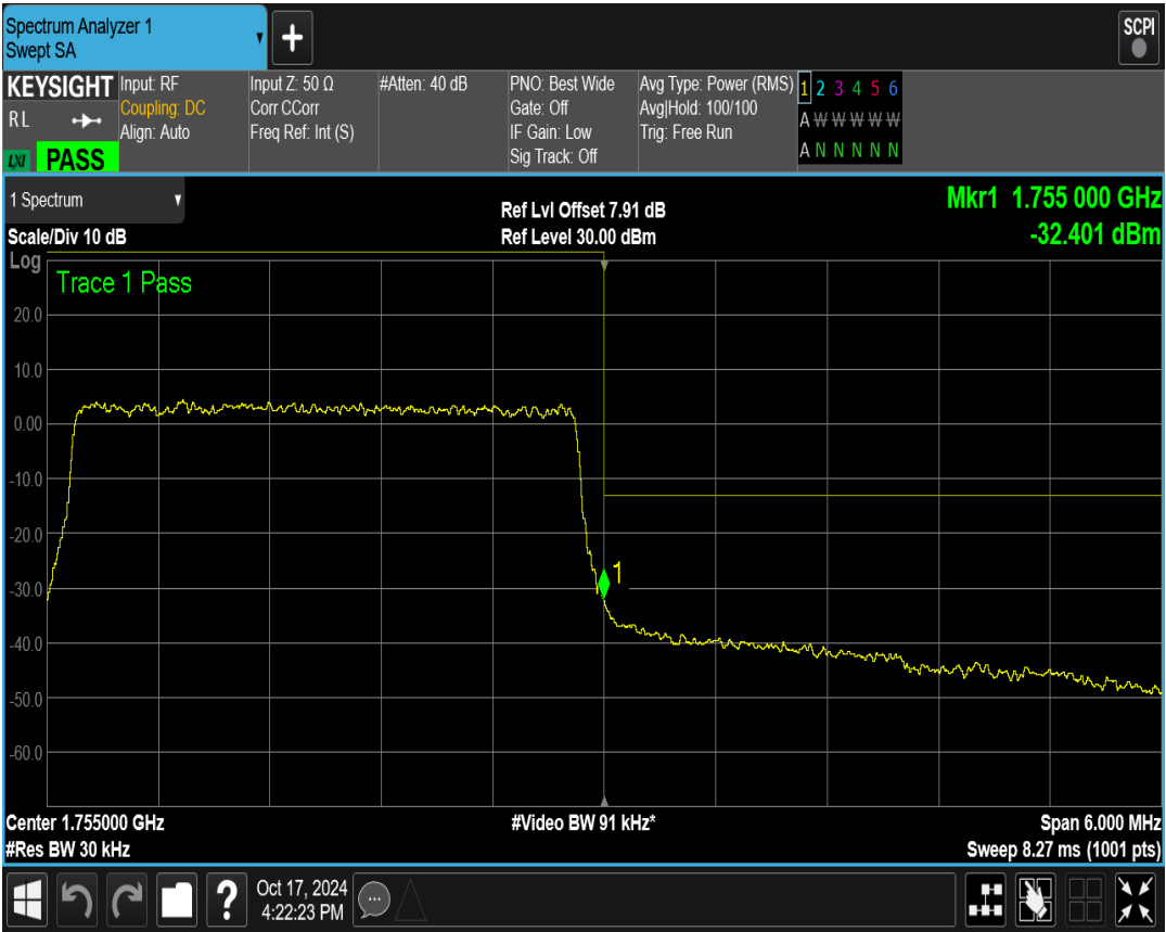
Band4 QPSK BW=5MHz Channel=19975 RB Size=25 Position=#0
