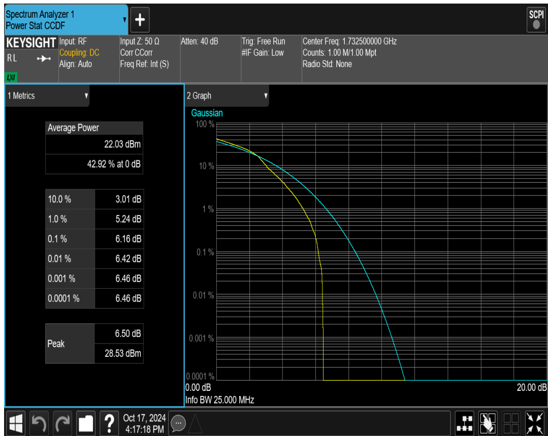
Band4 QAM16 BW=10MHz Channel=20175 RB Size=1 Position=#0
