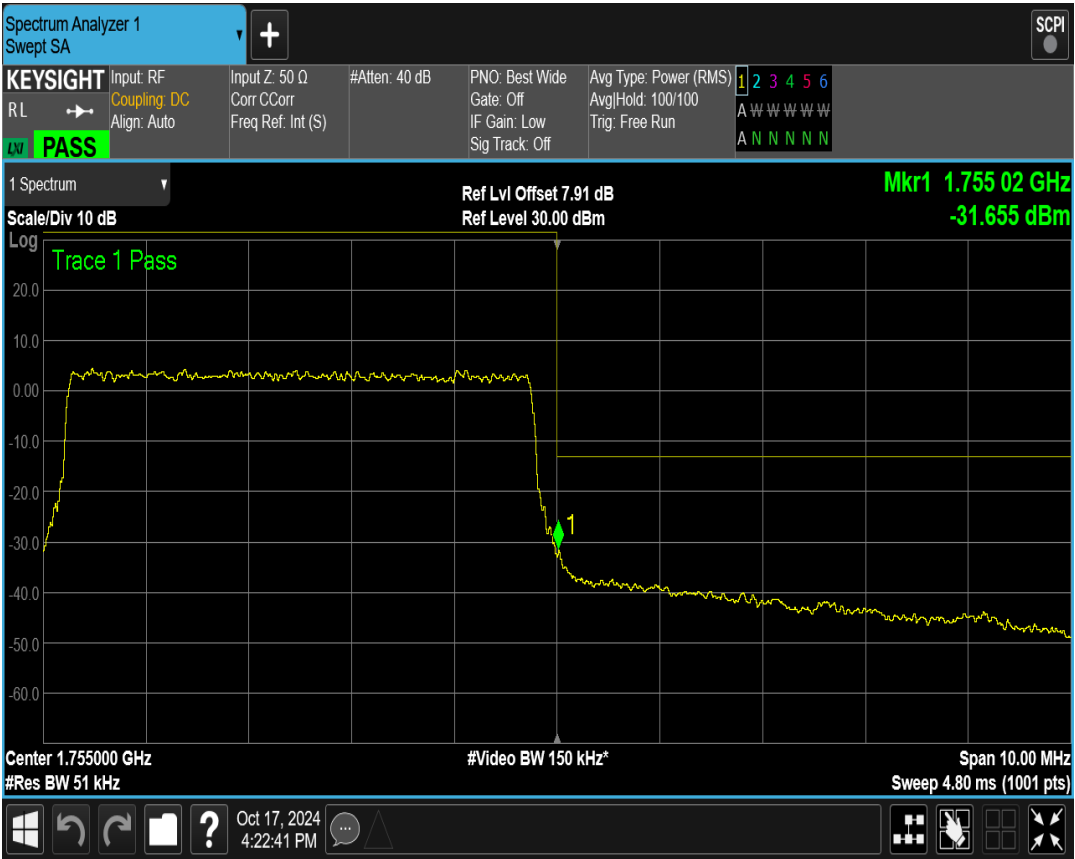
Band4 QPSK BW=3MHz Channel=19965 RB Size=15 Position=#0
