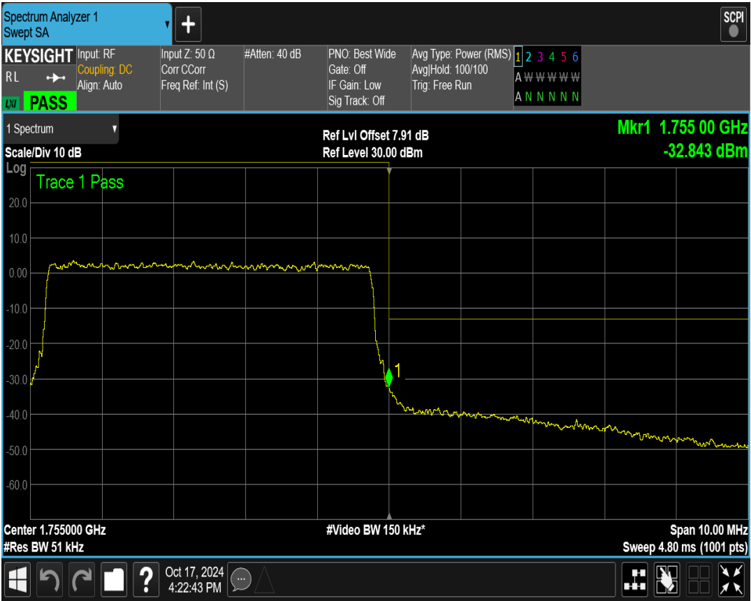
Band4 QPSK BW=3MHz Channel=20385 RB Size=15 Position=#0
