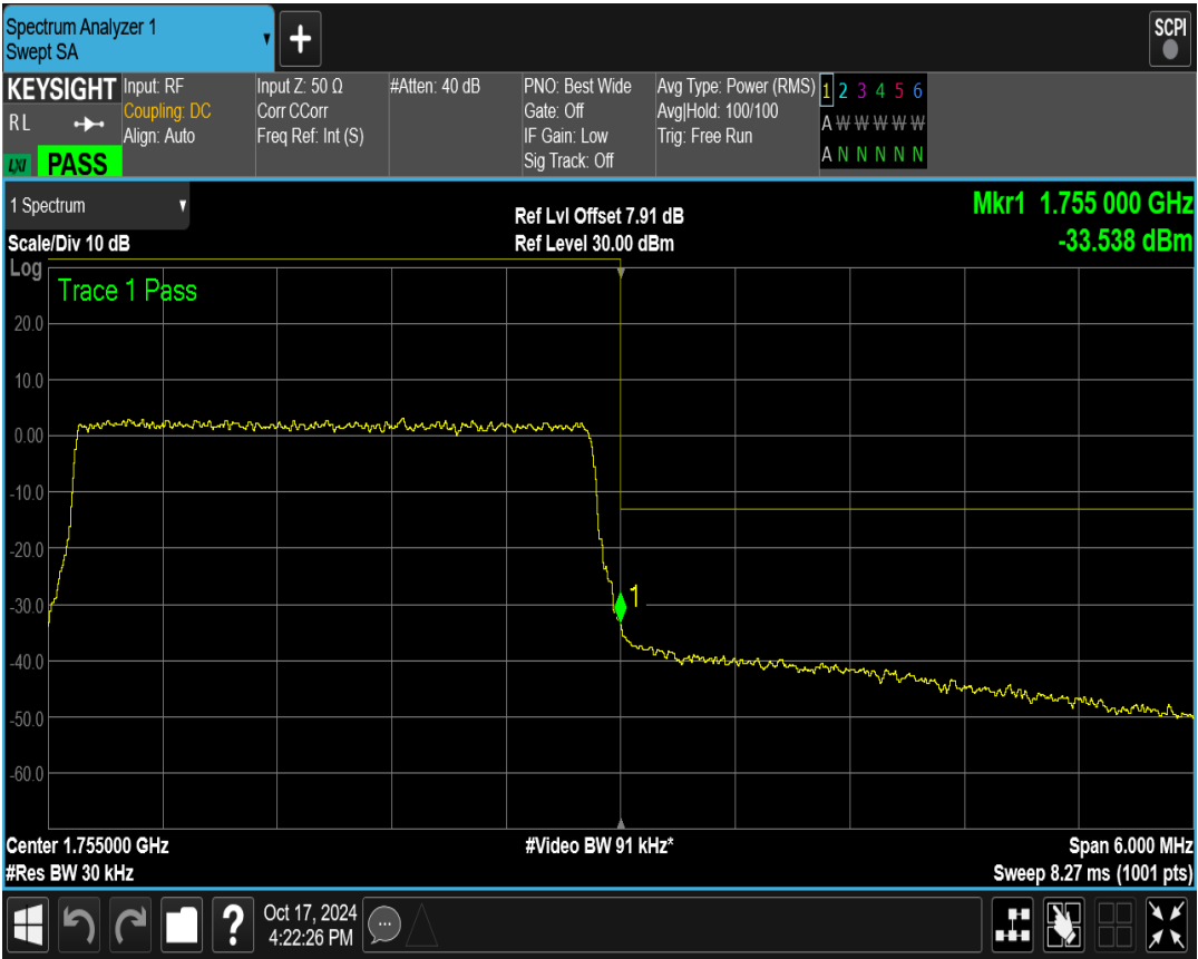
Band4 QPSK BW=1.4MHz Channel=19957 RB Size=6 Position=#0
