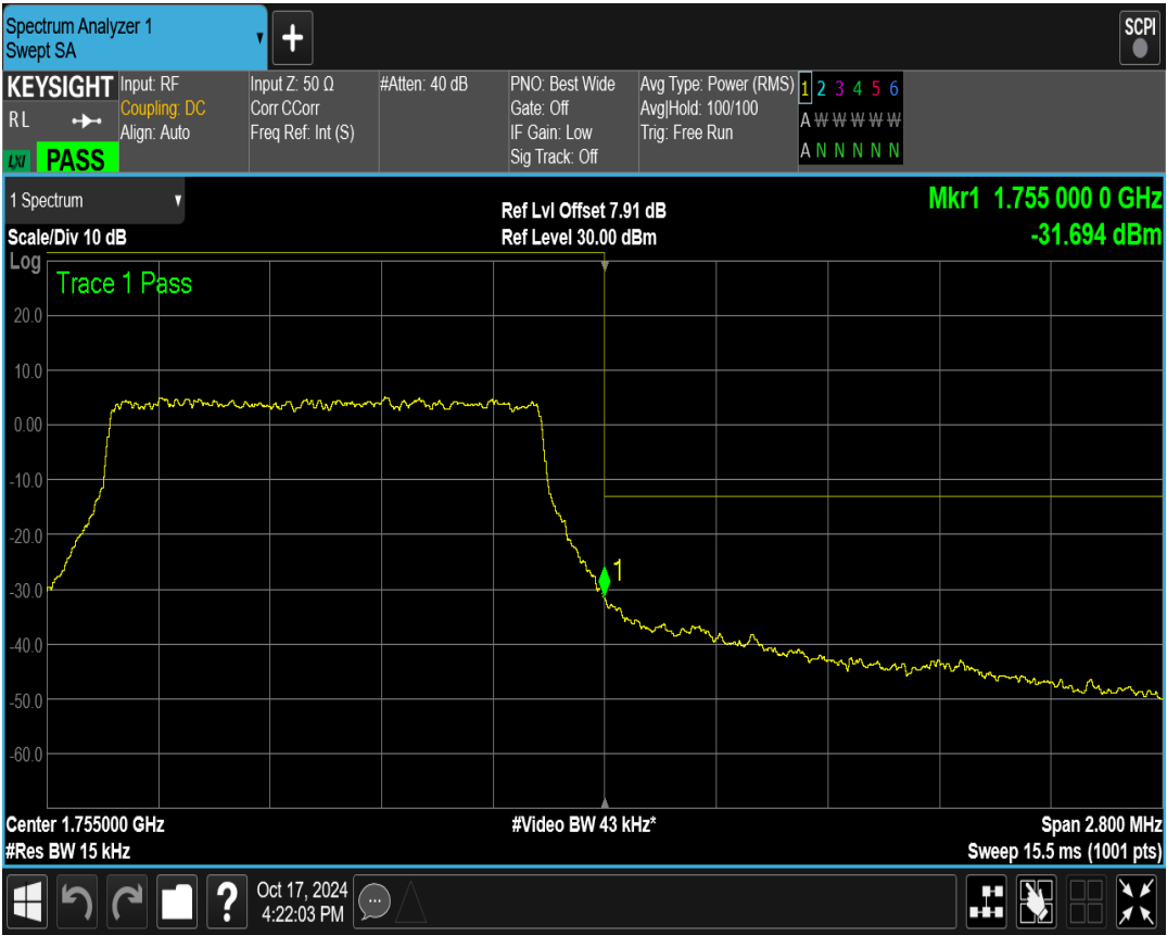
Band4 QPSK BW=15MHz Channel=20025 RB Size=75 Position=#0
