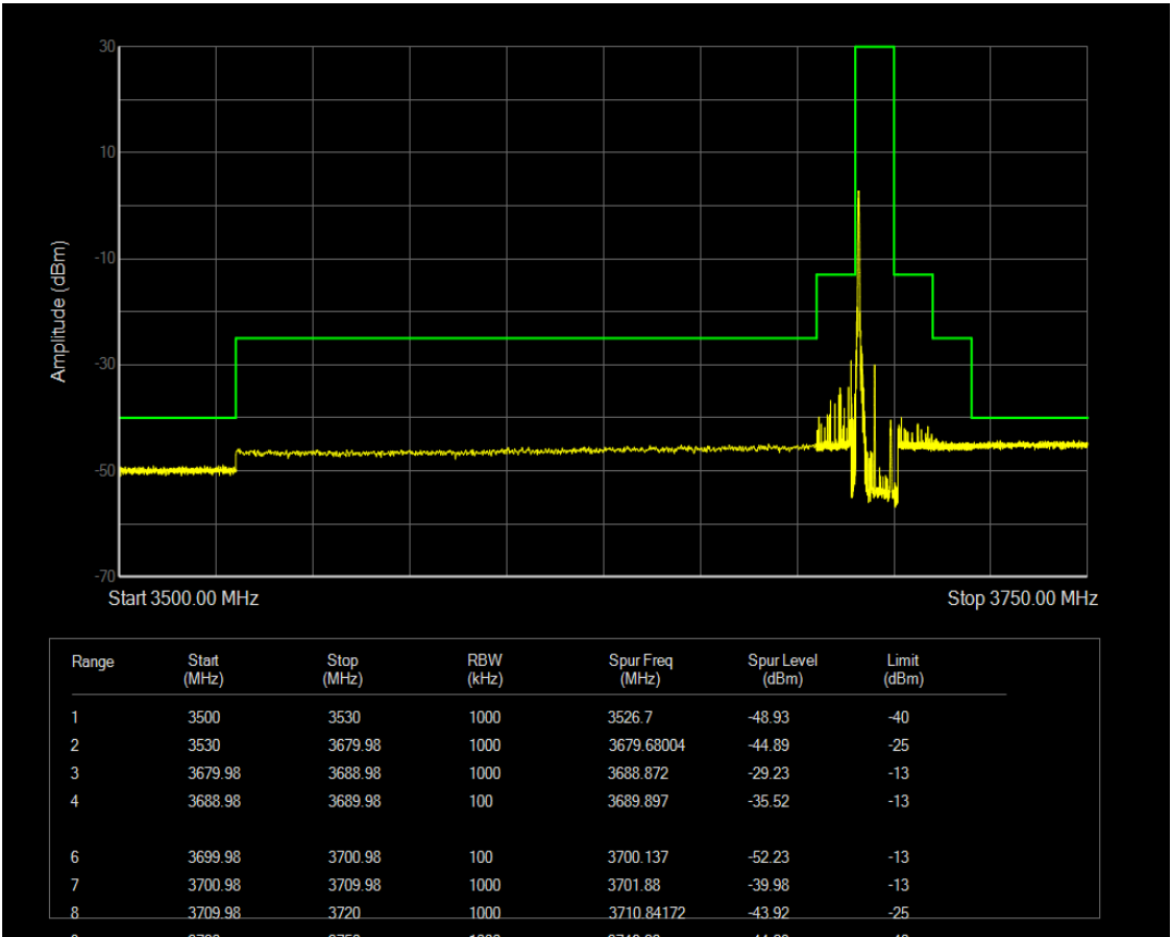
n78(3550-3700) SCS=30kHz CP_QPSK BW=10MHz Channel=646332 RB=1@23
