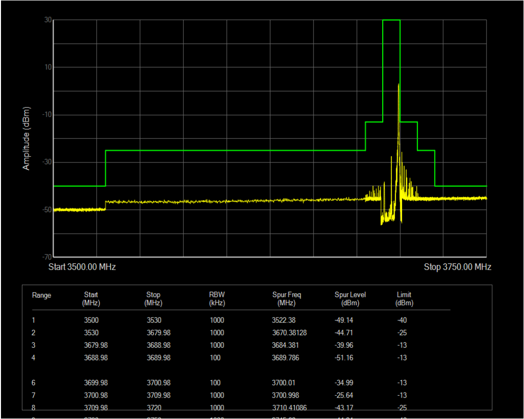
n78(3550-3700) SCS=30kHz CP_QPSK BW=50MHz Channel=638334 RB=133@0
