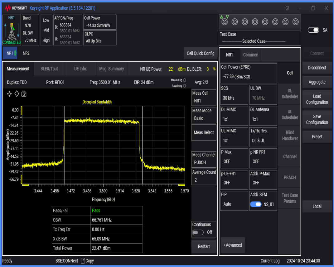
n78(3450-3550) SCS=30kHz DFT_QAM256 BW=70MHz Channel=633334 RB=180@0
