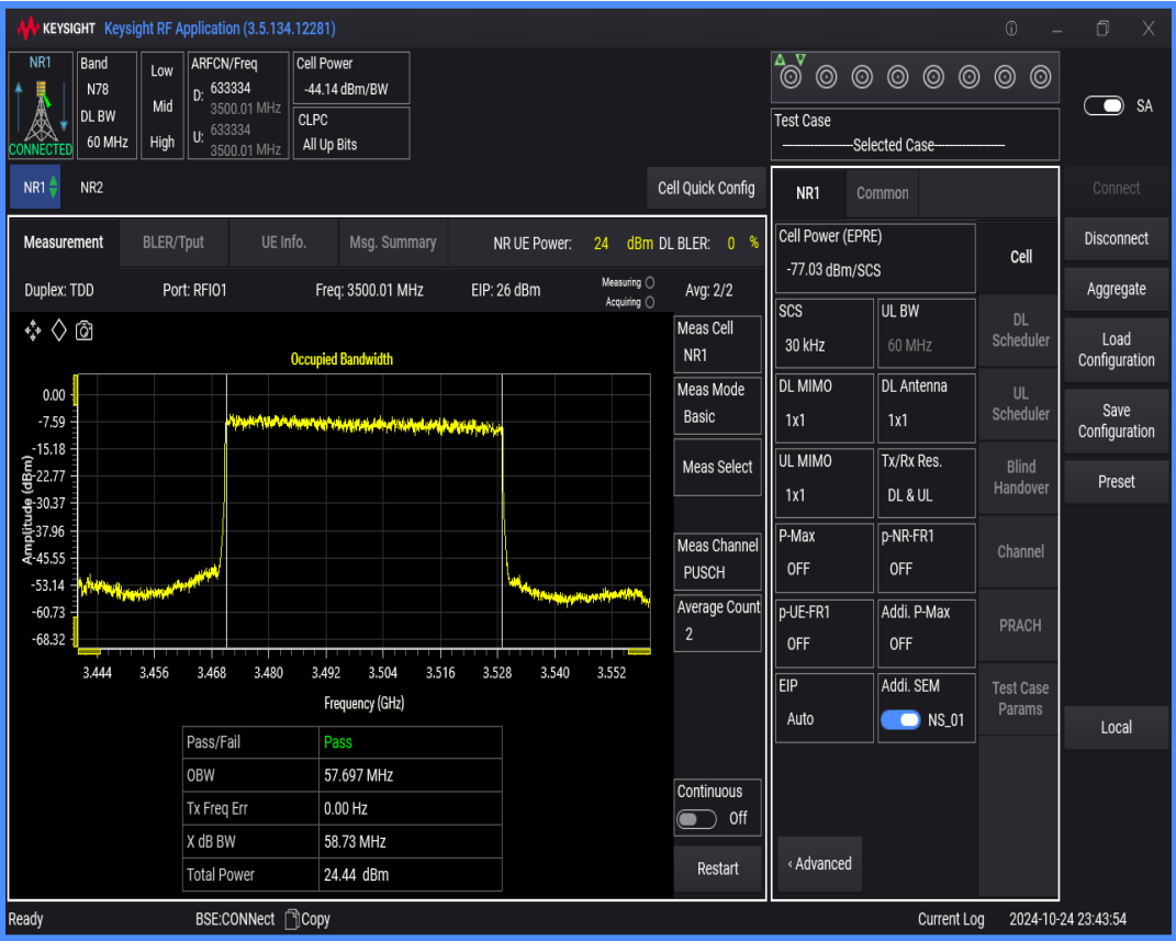
n78(3450-3550) SCS=30kHz DFT_QPSK BW=60MHz Channel=633334 RB=162@0
