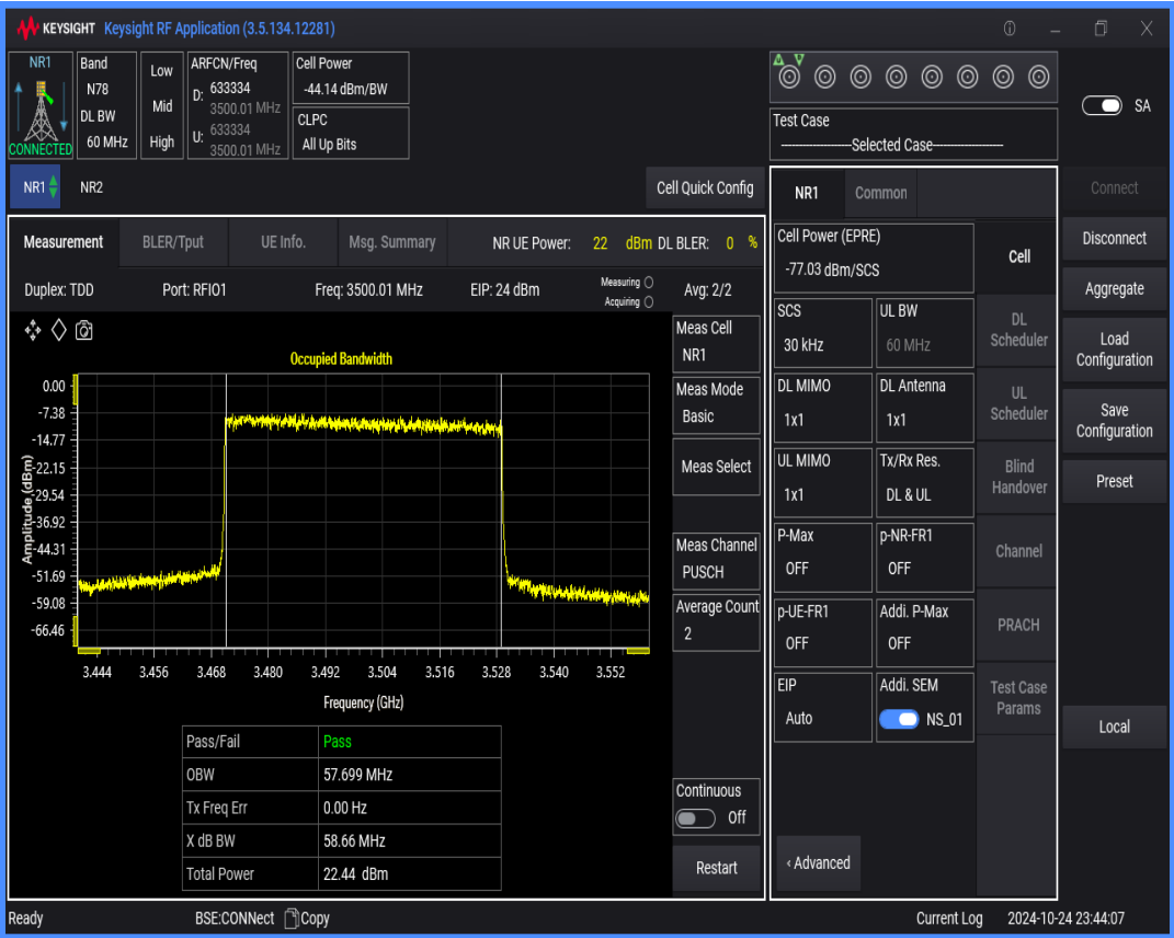
n78(3450-3550) SCS=30kHz DFT_QAM256 BW=60MHz Channel=633334 RB=162@0
