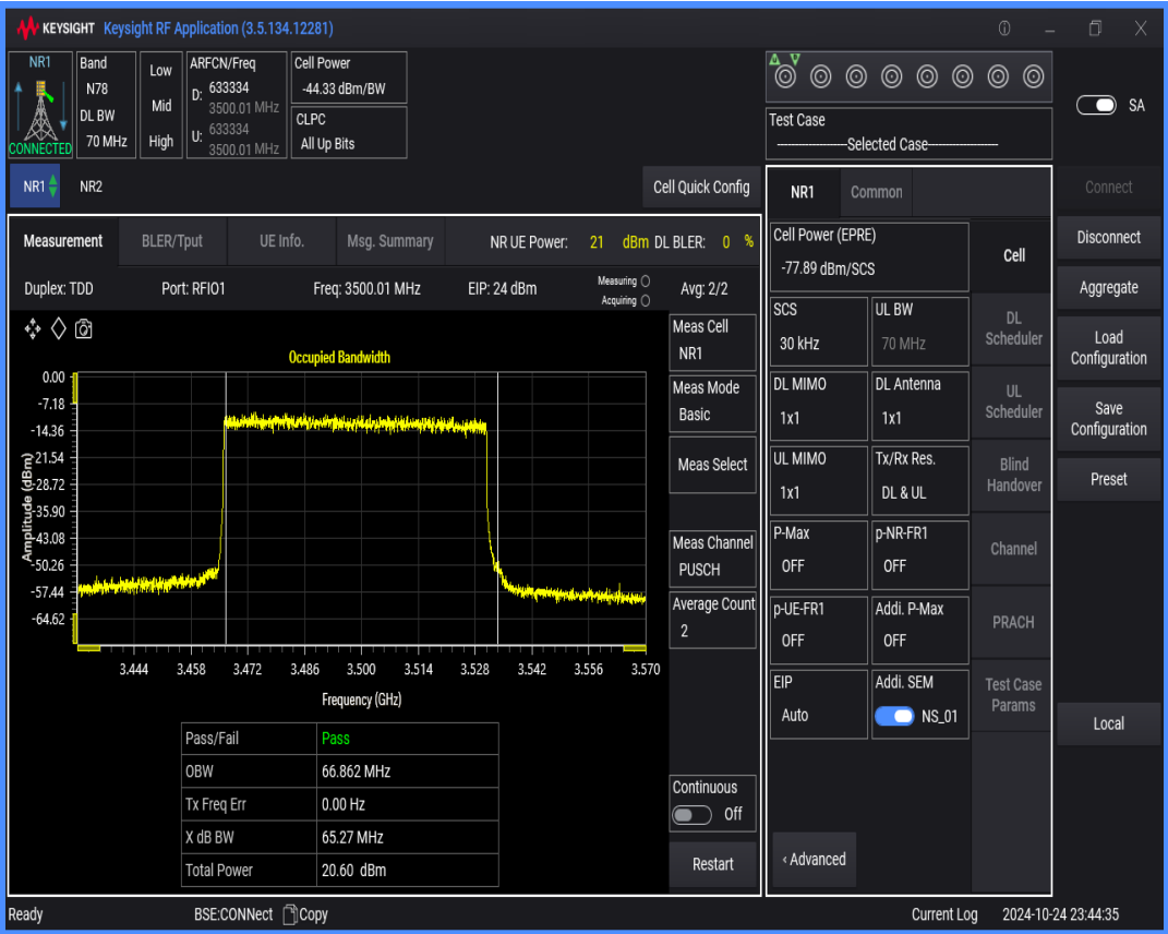
n78(3450-3550) SCS=30kHz DFT_QPSK BW=80MHz Channel=633334 RB=216@0
