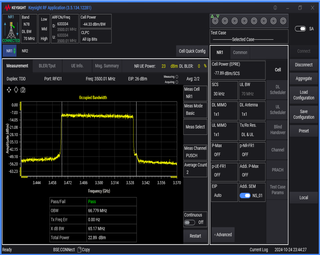
n78(3450-3550) SCS=30kHz DFT_QAM64 BW=70MHz Channel=633334 RB=180@0
