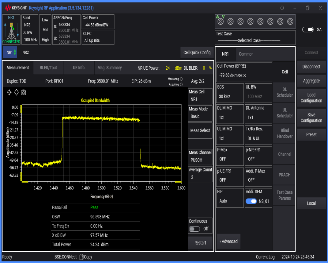
n78(3450-3550) SCS=30kHz DFT_QPSK BW=100MHz Channel=633334 RB=270@0
