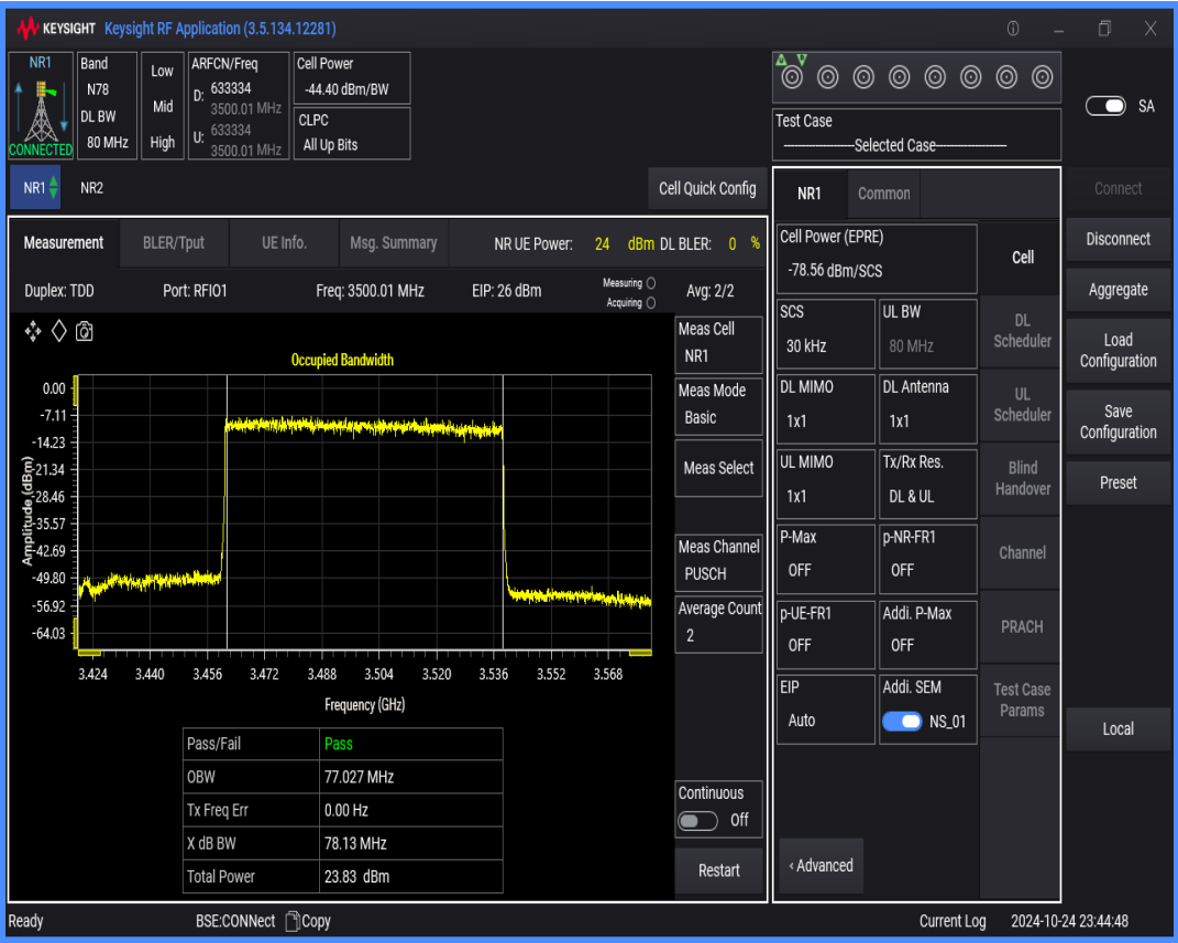
n78(3450-3550) SCS=30kHz DFT_BPSK BW=80MHz Channel=633334 RB=216@0
