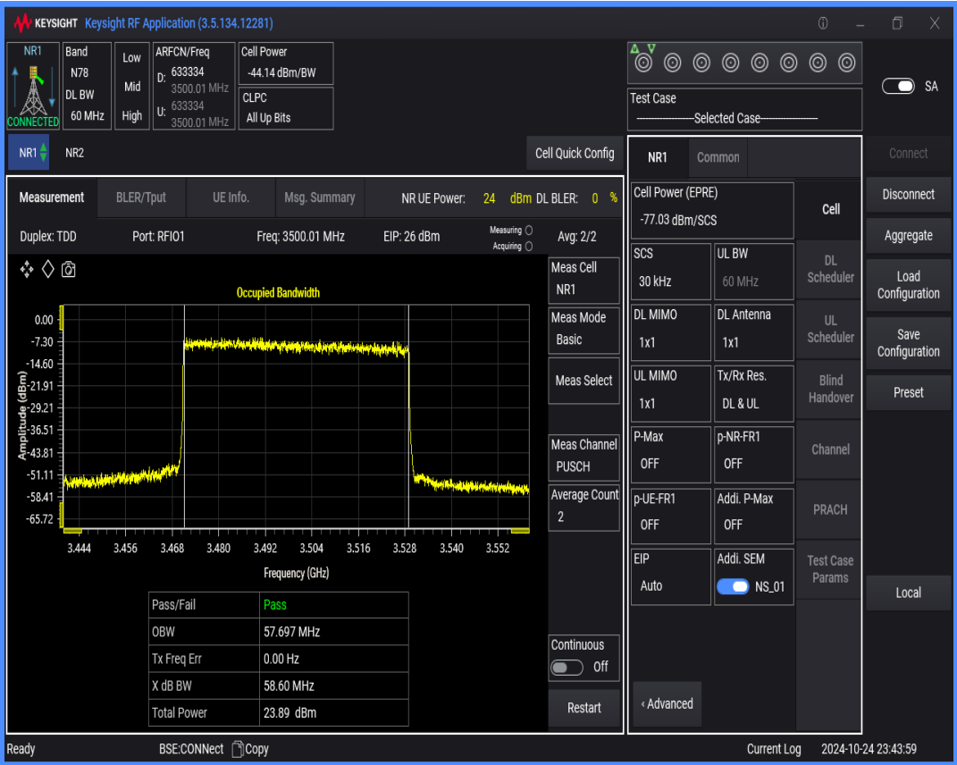
n78(3450-3550) SCS=30kHz DFT_QAM16 BW=60MHz Channel=633334 RB=162@0
