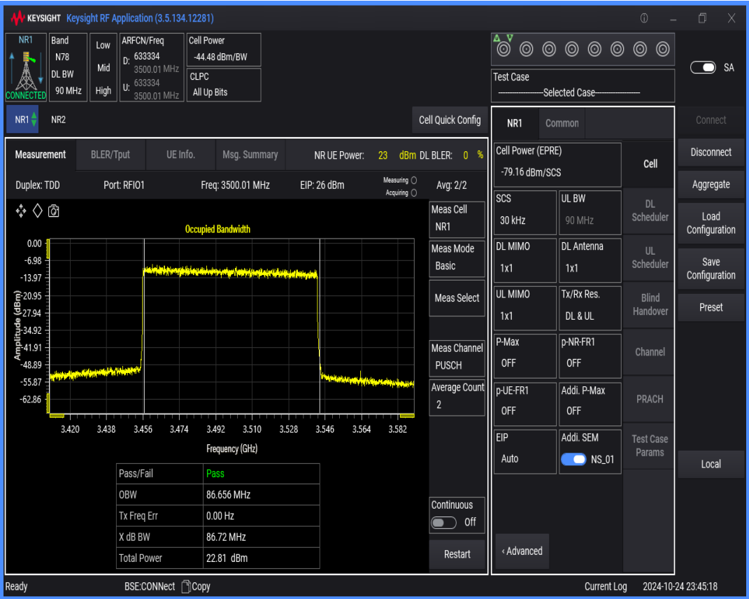
n78(3450-3550) SCS=30kHz DFT_QAM64 BW=90MHz Channel=633334 RB=240@0
