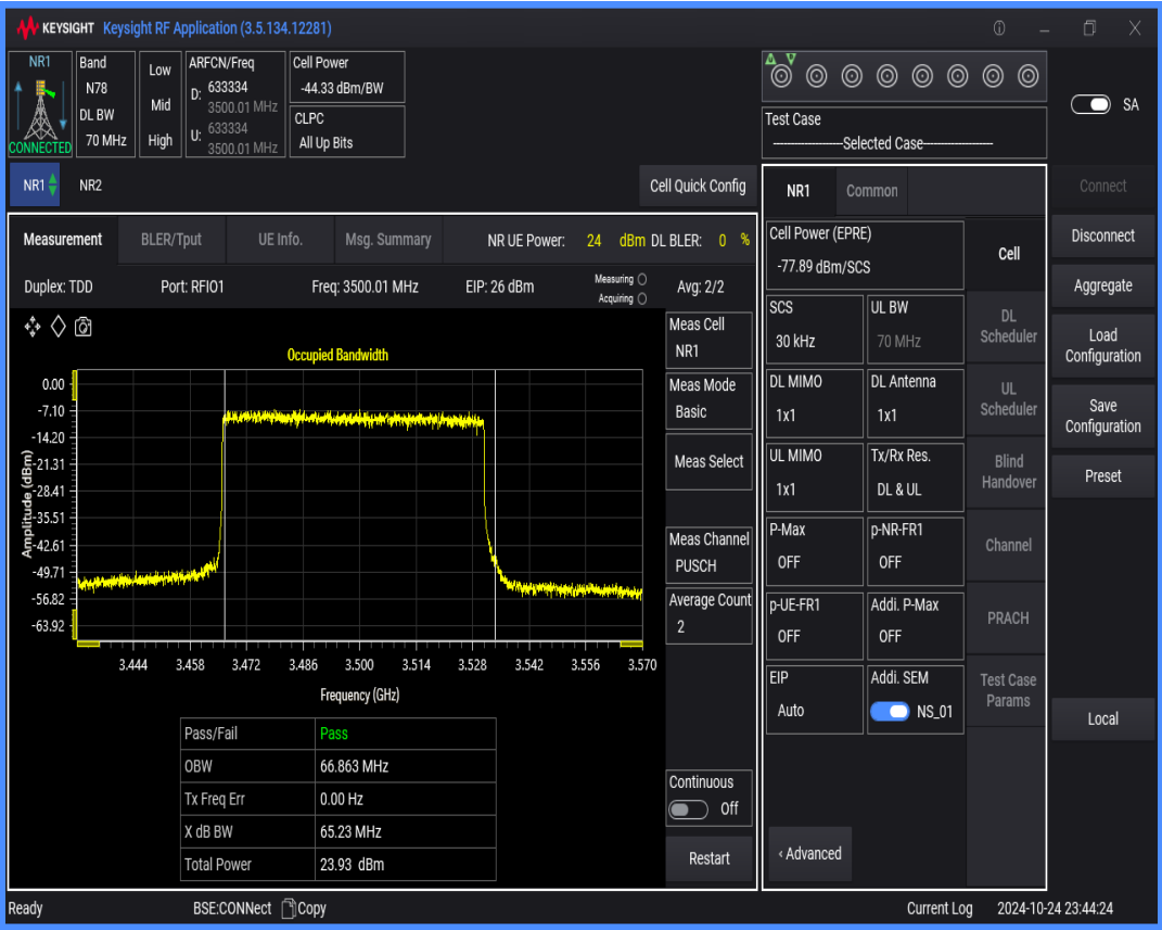
n78(3450-3550) SCS=30kHz DFT_QAM16 BW=70MHz Channel=633334 RB=180@0
