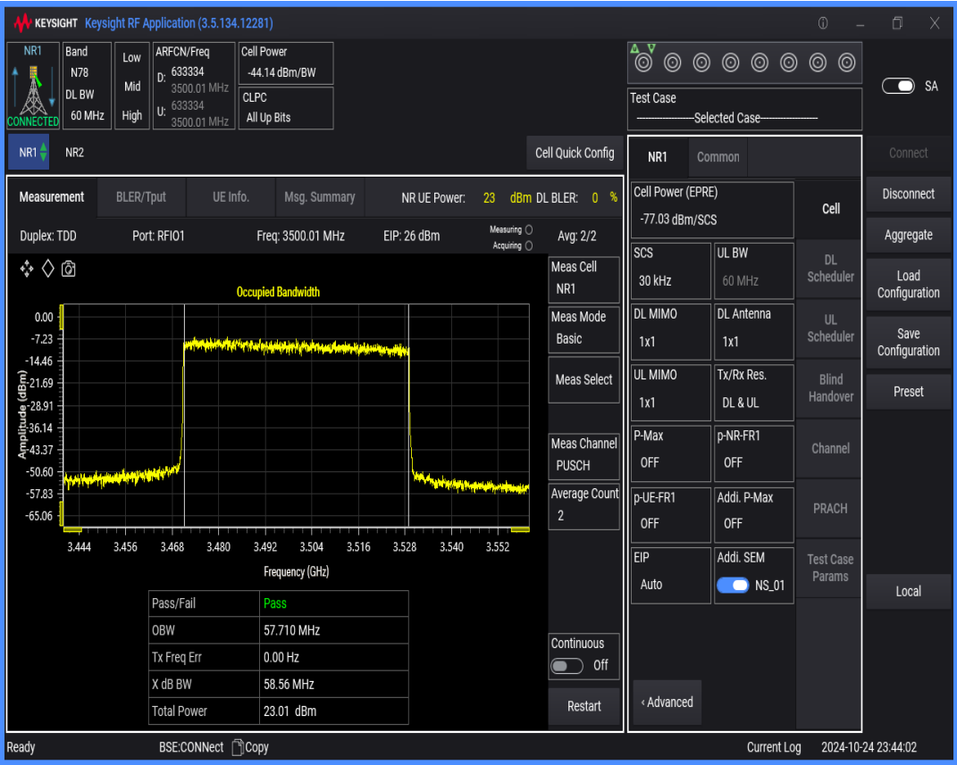
n78(3450-3550) SCS=30kHz DFT_QAM64 BW=60MHz Channel=633334 RB=162@0
