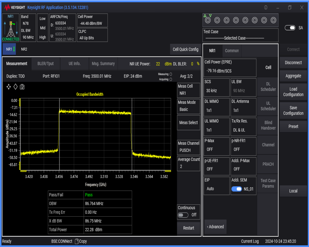
n78(3450-3550) SCS=30kHz DFT_QAM256 BW=90MHz Channel=633334 RB=240@0
