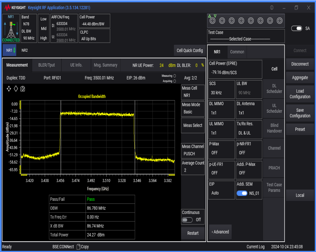
n78(3450-3550) SCS=30kHz DFT_QPSK BW=90MHz Channel=633334 RB=240@0
