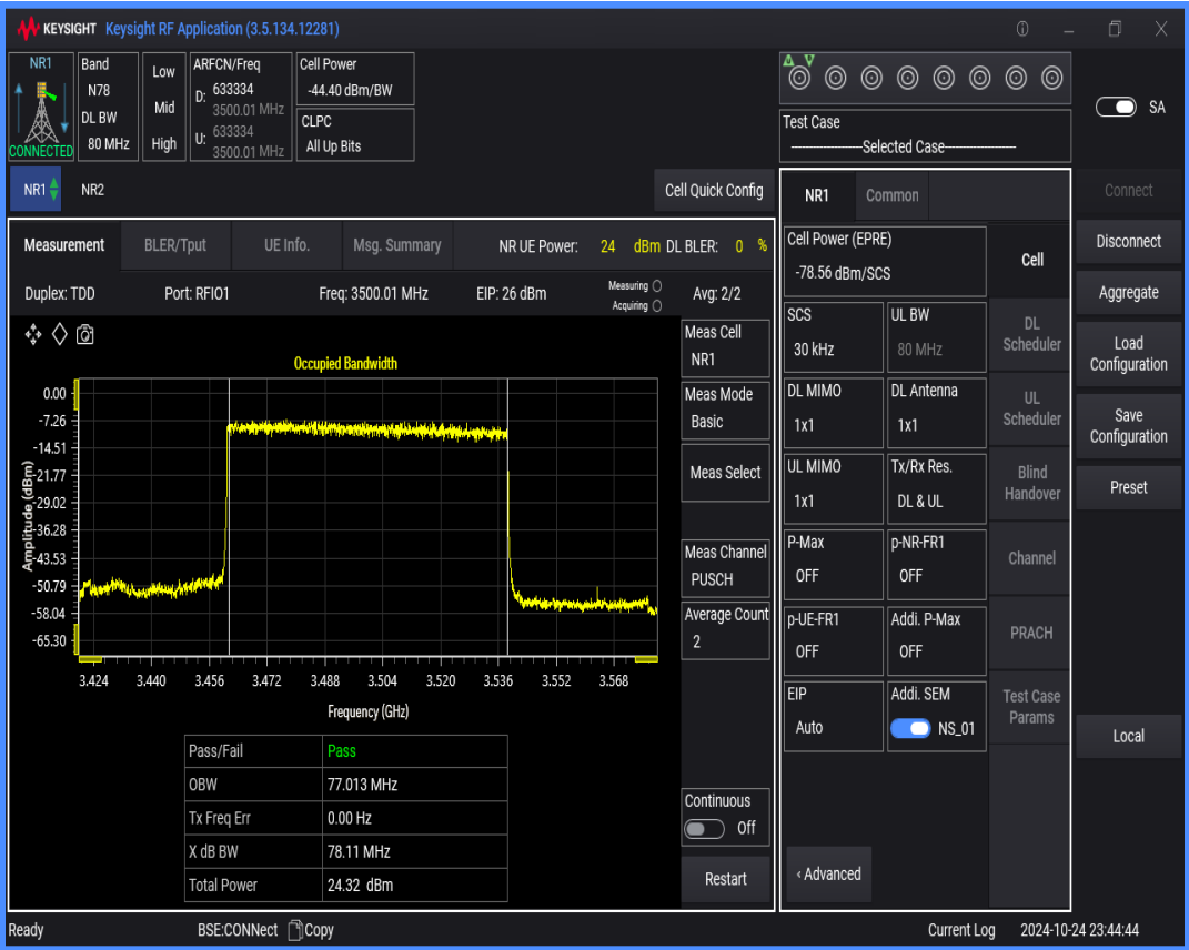
n78(3450-3550) SCS=30kHz DFT_QAM16 BW=80MHz Channel=633334 RB=216@0
