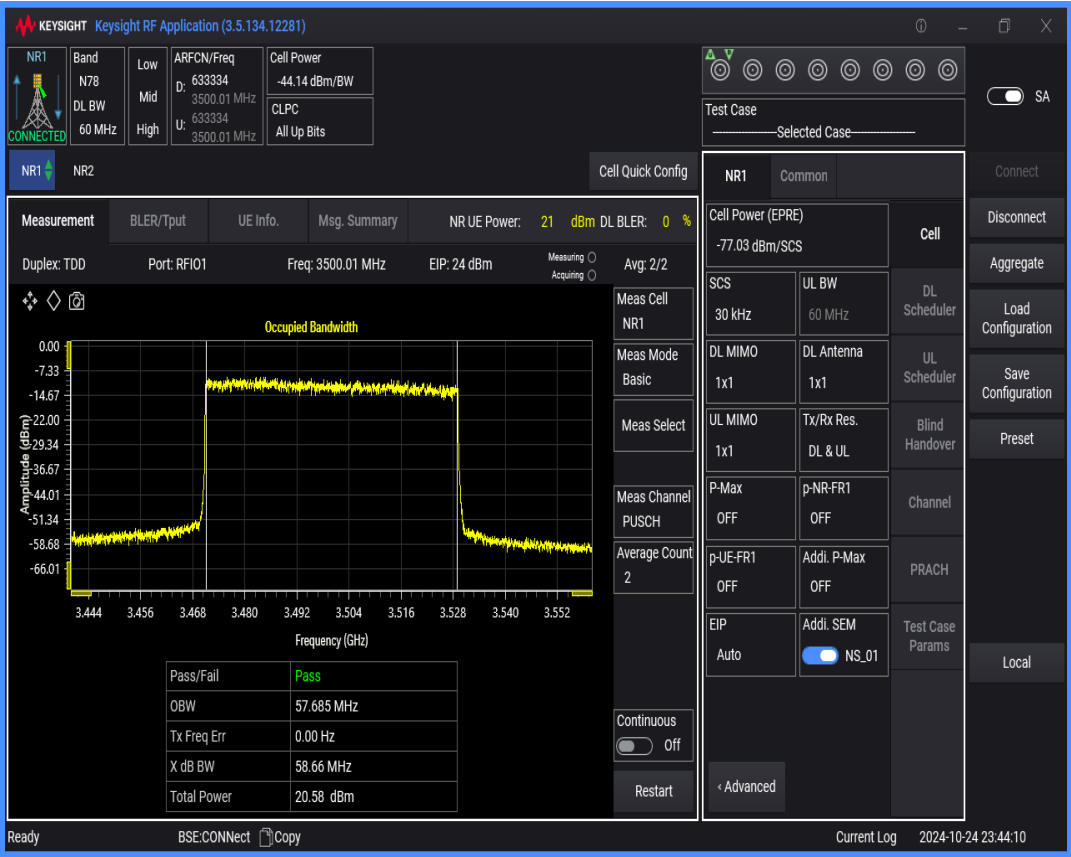
n78(3450-3550) SCS=30kHz DFT_BPSK BW=70MHz Channel=633334 RB=180@0
