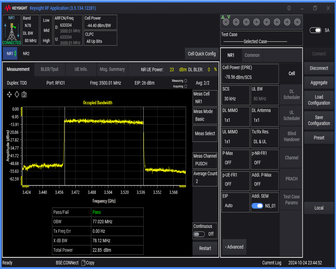
n78(3450-3550) SCS=30kHz DFT_QAM64 BW=80MHz Channel=633334 RB=216@0
