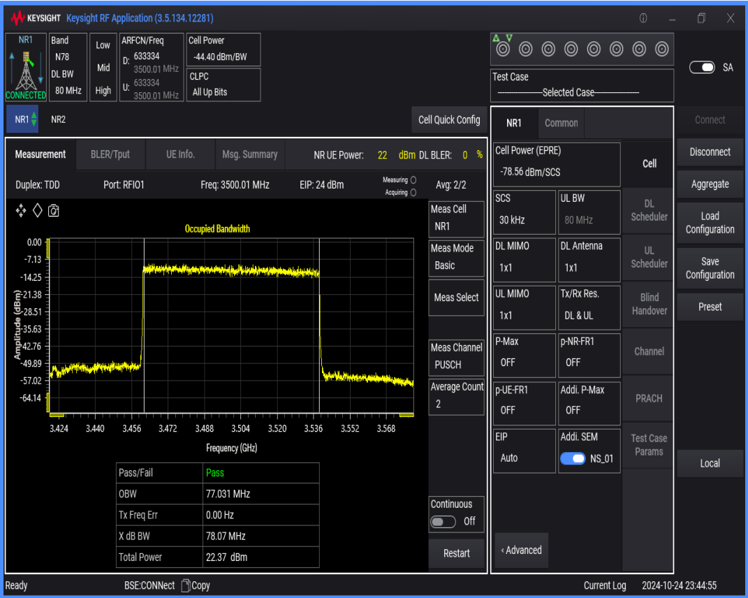
n78(3450-3550) SCS=30kHz DFT_QAM256 BW=80MHz Channel=633334 RB=216@0
