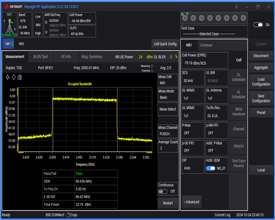
n78(3450-3550) SCS=30kHz DFT_QAM16 BW=90MHz Channel=633334 RB=240@0
