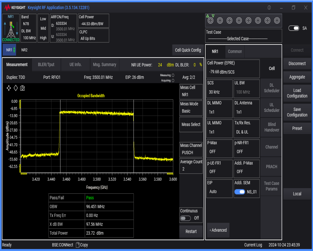
n78(3450-3550) SCS=30kHz DFT_QAM16 BW=100MHz Channel=633334 RB=270@0
