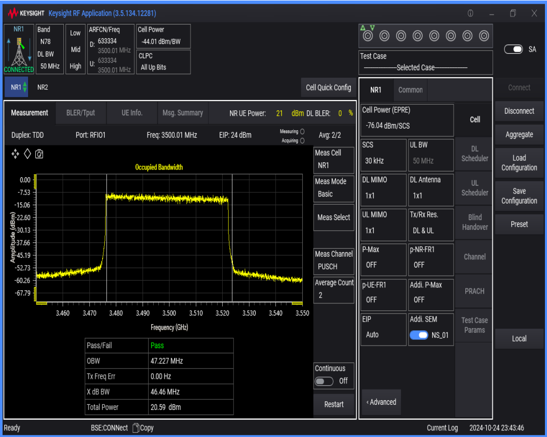
n78(3450-3550) SCS=30kHz DFT_BPSK BW=60MHz Channel=633334 RB=162@0
