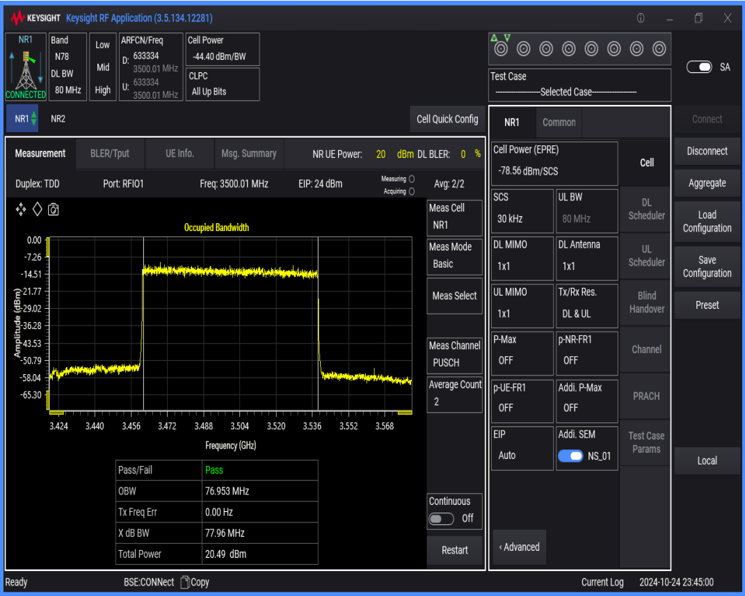
n78(3450-3550) SCS=30kHz DFT_BPSK BW=90MHz Channel=633334 RB=240@0
