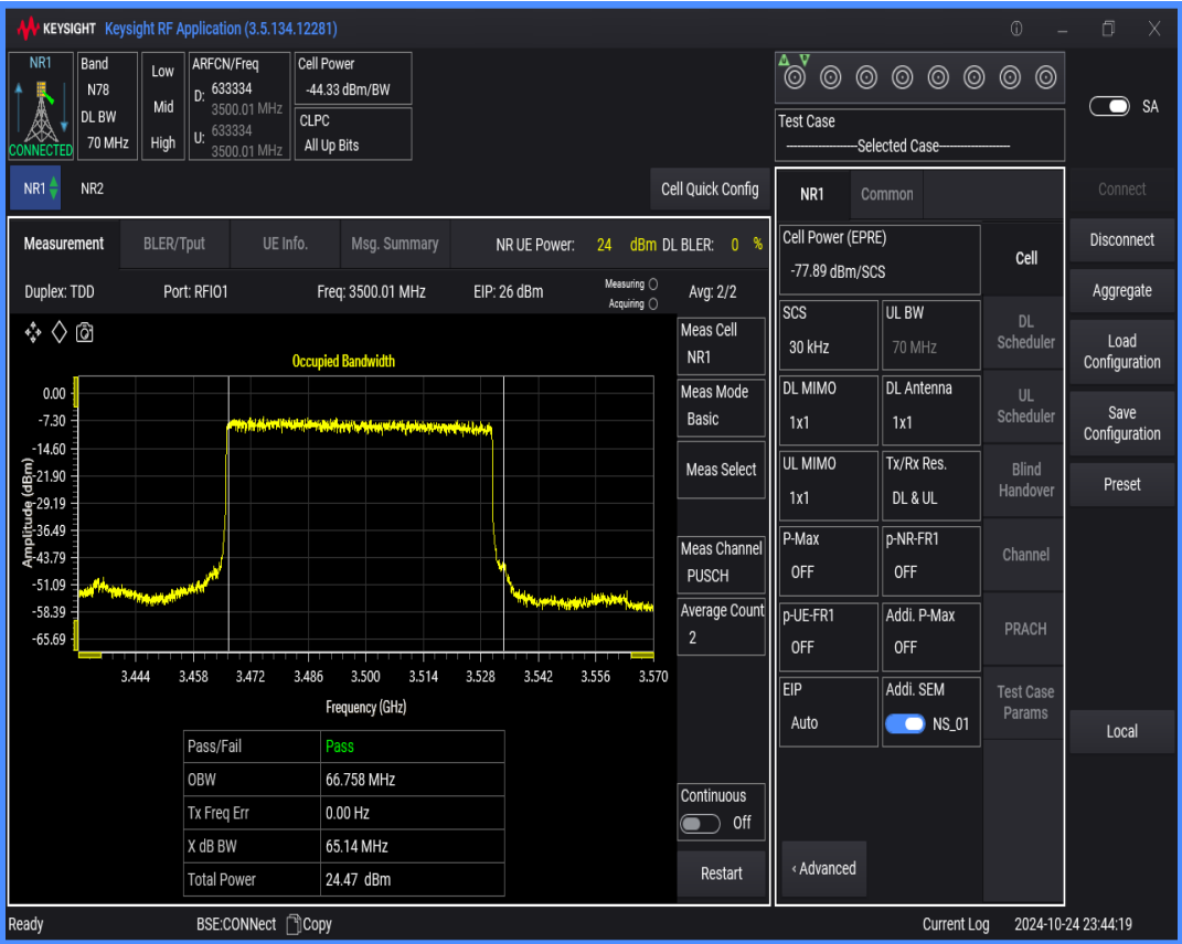
n78(3450-3550) SCS=30kHz DFT_QPSK BW=70MHz Channel=633334 RB=180@0
