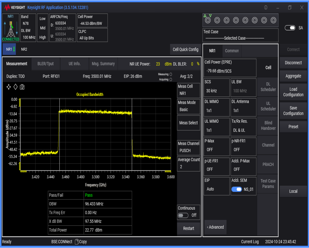
n78(3450-3550) SCS=30kHz DFT_QAM64 BW=100MHz Channel=633334 RB=270@0
