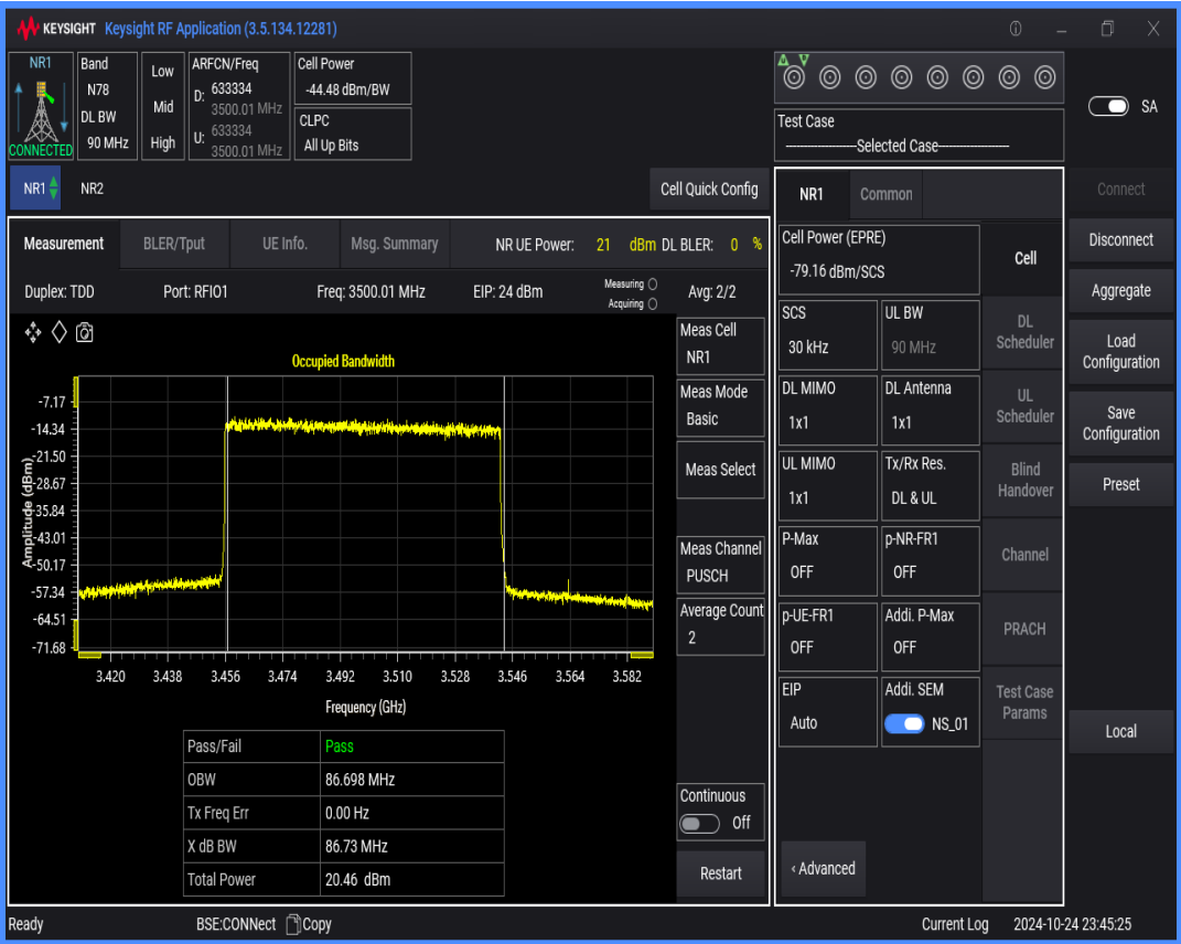
n78(3450-3550) SCS=30kHz DFT_BPSK BW=100MHz Channel=633334 RB=270@0
