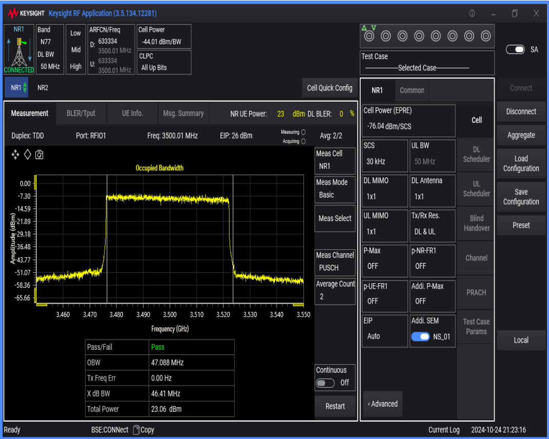
n77(3450-3550) SCS=30kHz DFT_QAM64 BW=50MHz Channel=633334 RB=128@0
