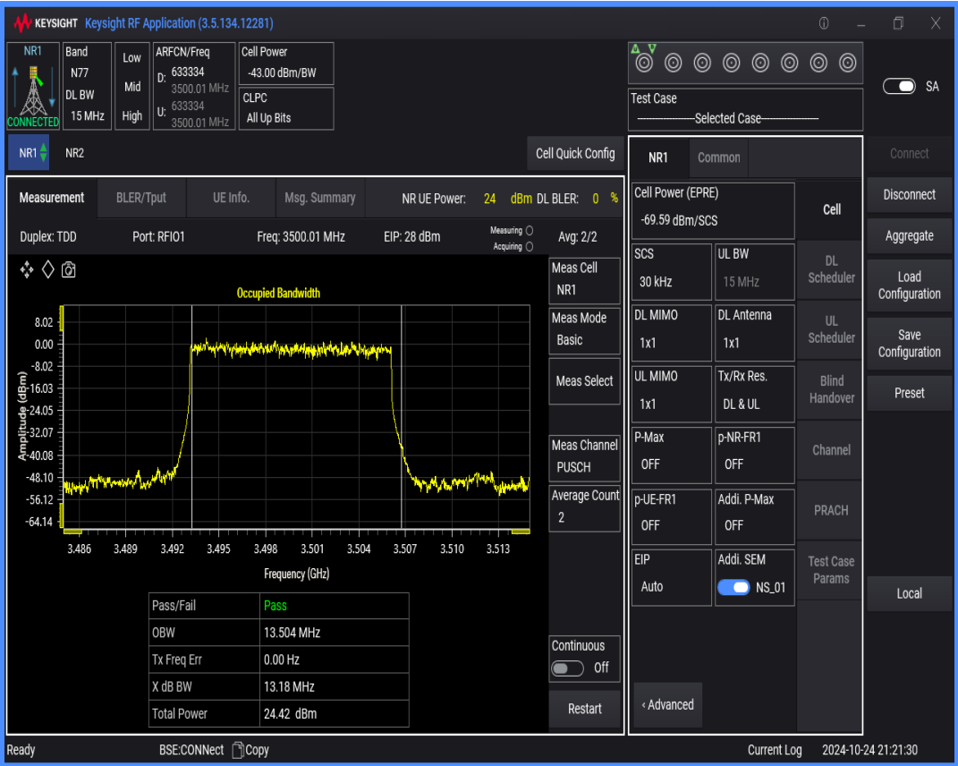
n77(3450-3550) SCS=30kHz DFT_QPSK BW=15MHz Channel=633334 RB=36@0
