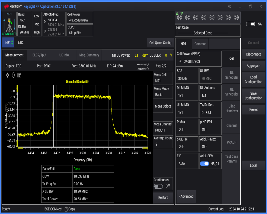
n77(3450-3550) SCS=30kHz DFT_BPSK BW=30MHz Channel=633334 RB=75@0
