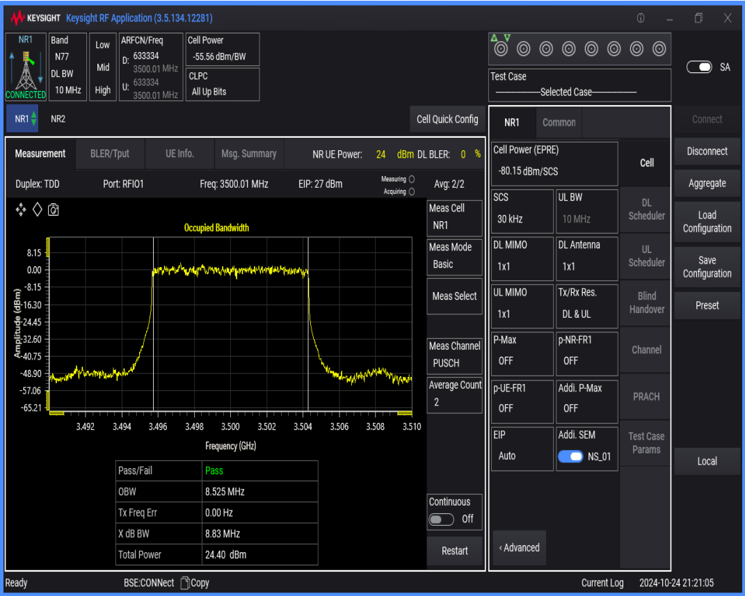
n77(3450-3550) SCS=30kHz DFT_QPSK BW=10MHz Channel=633334 RB=24@0
