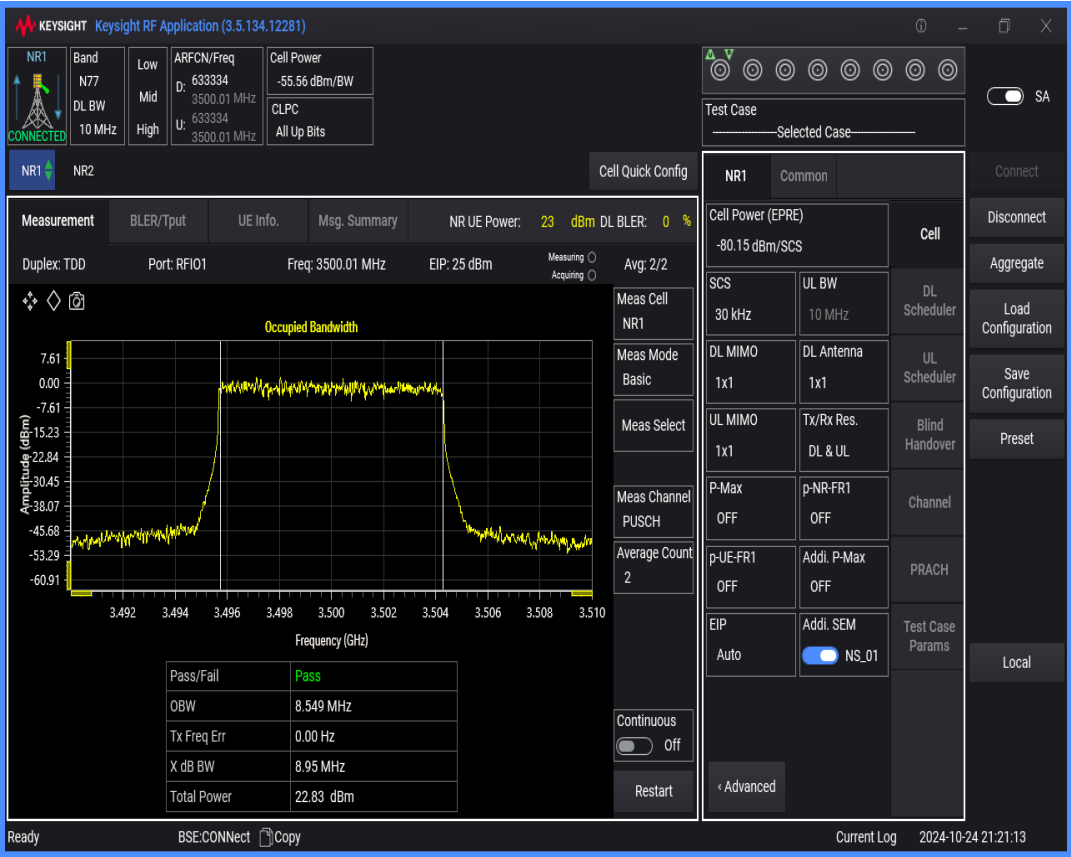
n77(3450-3550) SCS=30kHz DFT_QAM64 BW=10MHz Channel=633334 RB=24@0
