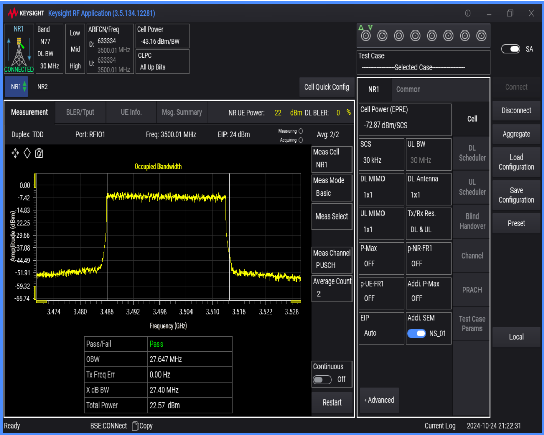
n77(3450-3550) SCS=30kHz DFT_BPSK BW=40MHz Channel=633334 RB=100@0
