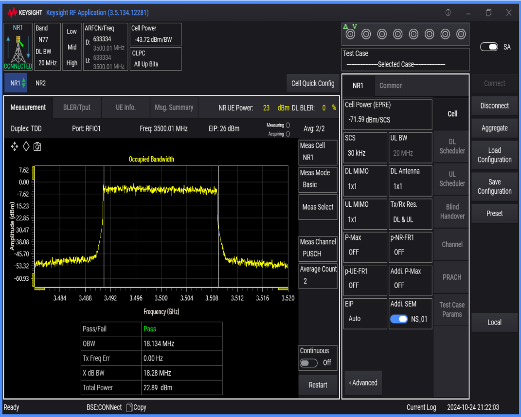
n77(3450-3550) SCS=30kHz DFT_QAM64 BW=20MHz Channel=633334 RB=50@0
