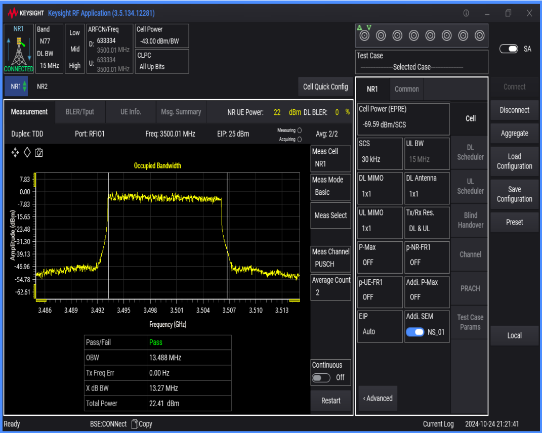
n77(3450-3550) SCS=30kHz DFT_QAM16 BW=15MHz Channel=633334 RB=36@0
