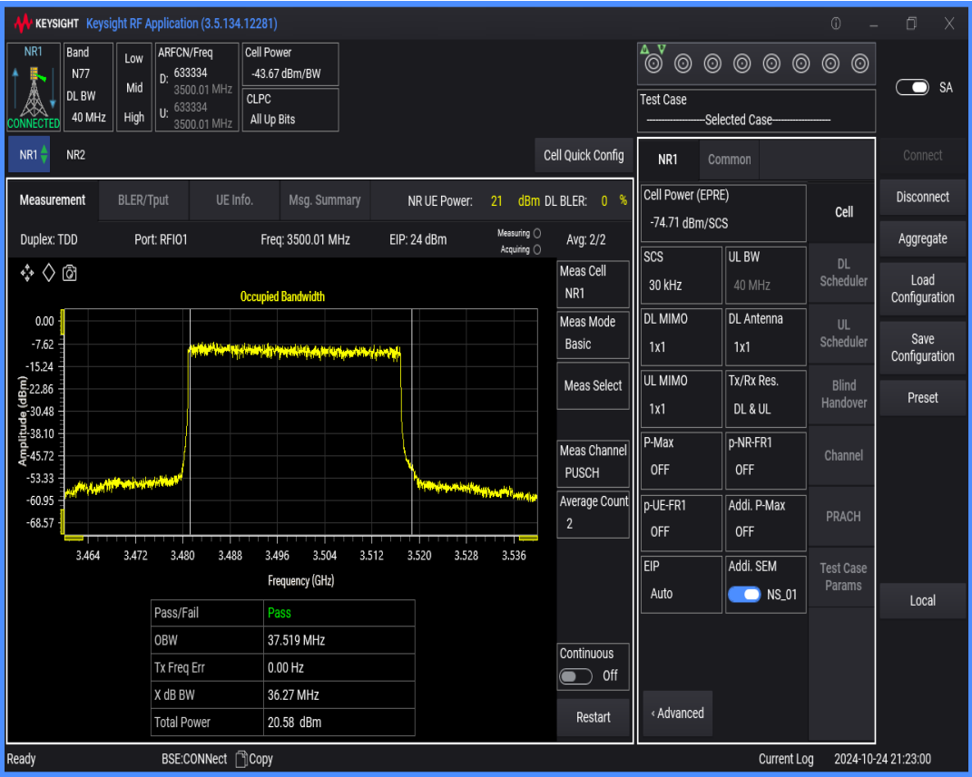
n77(3450-3550) SCS=30kHz DFT_BPSK BW=50MHz Channel=633334 RB=128@0
