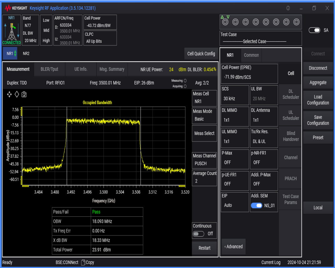
n77(3450-3550) SCS=30kHz DFT_QAM16 BW=20MHz Channel=633334 RB=50@0
