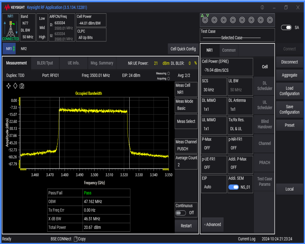
n77(3450-3550) SCS=30kHz DFT_BPSK BW=60MHz Channel=633334 RB=162@0
