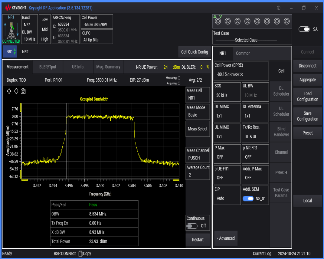
n77(3450-3550) SCS=30kHz DFT_QAM16 BW=10MHz Channel=633334 RB=24@0
