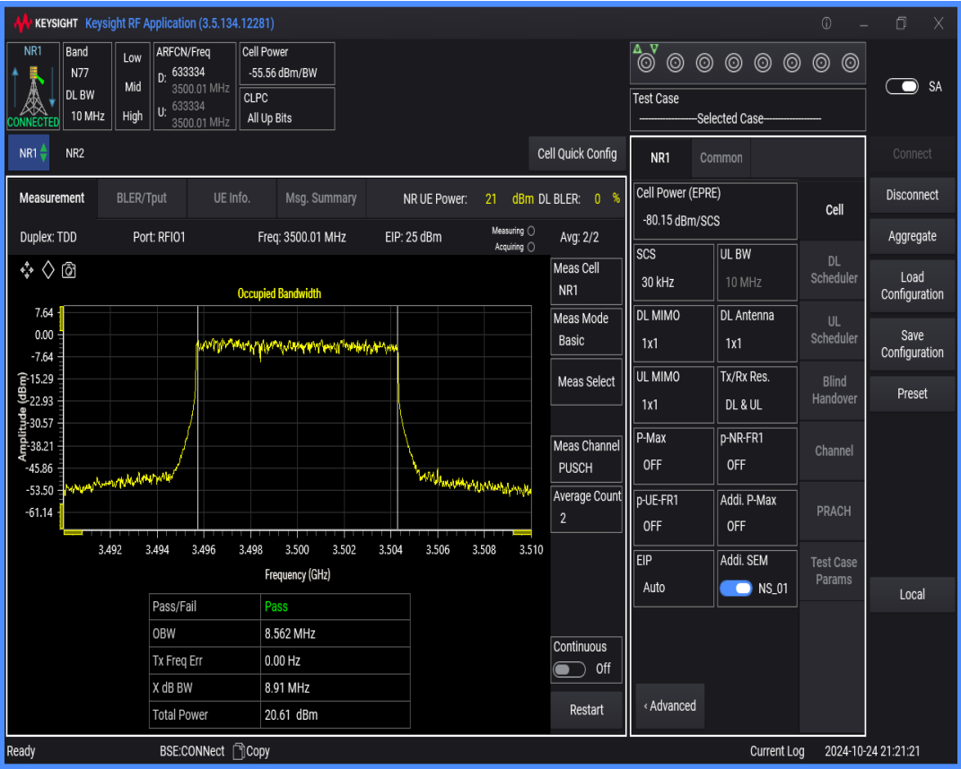
n77(3450-3550) SCS=30kHz DFT_BPSK BW=15MHz Channel=633334 RB=36@0
