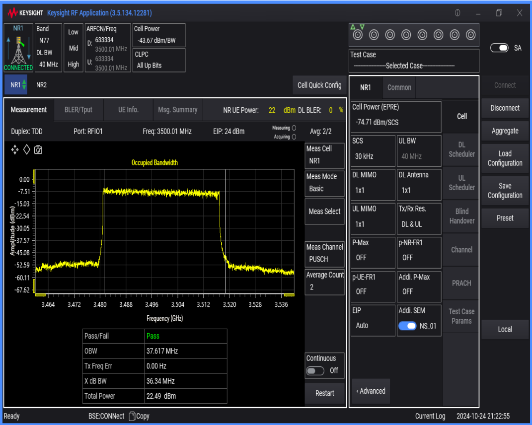
n77(3450-3550) SCS=30kHz DFT_QAM256 BW=40MHz Channel=633334 RB=100@0
