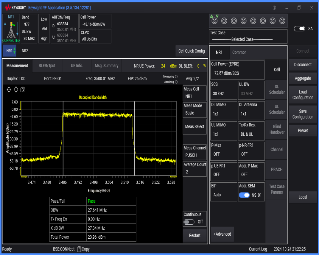
n77(3450-3550) SCS=30kHz DFT_QAM16 BW=30MHz Channel=633334 RB=75@0
