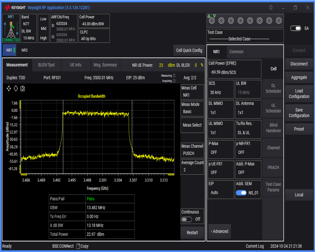
n77(3450-3550) SCS=30kHz DFT_QAM256 BW=15MHz Channel=633334 RB=36@0
