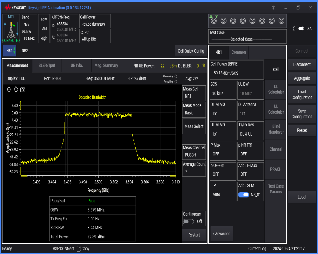
n77(3450-3550) SCS=30kHz DFT_QAM256 BW=10MHz Channel=633334 RB=24@0
