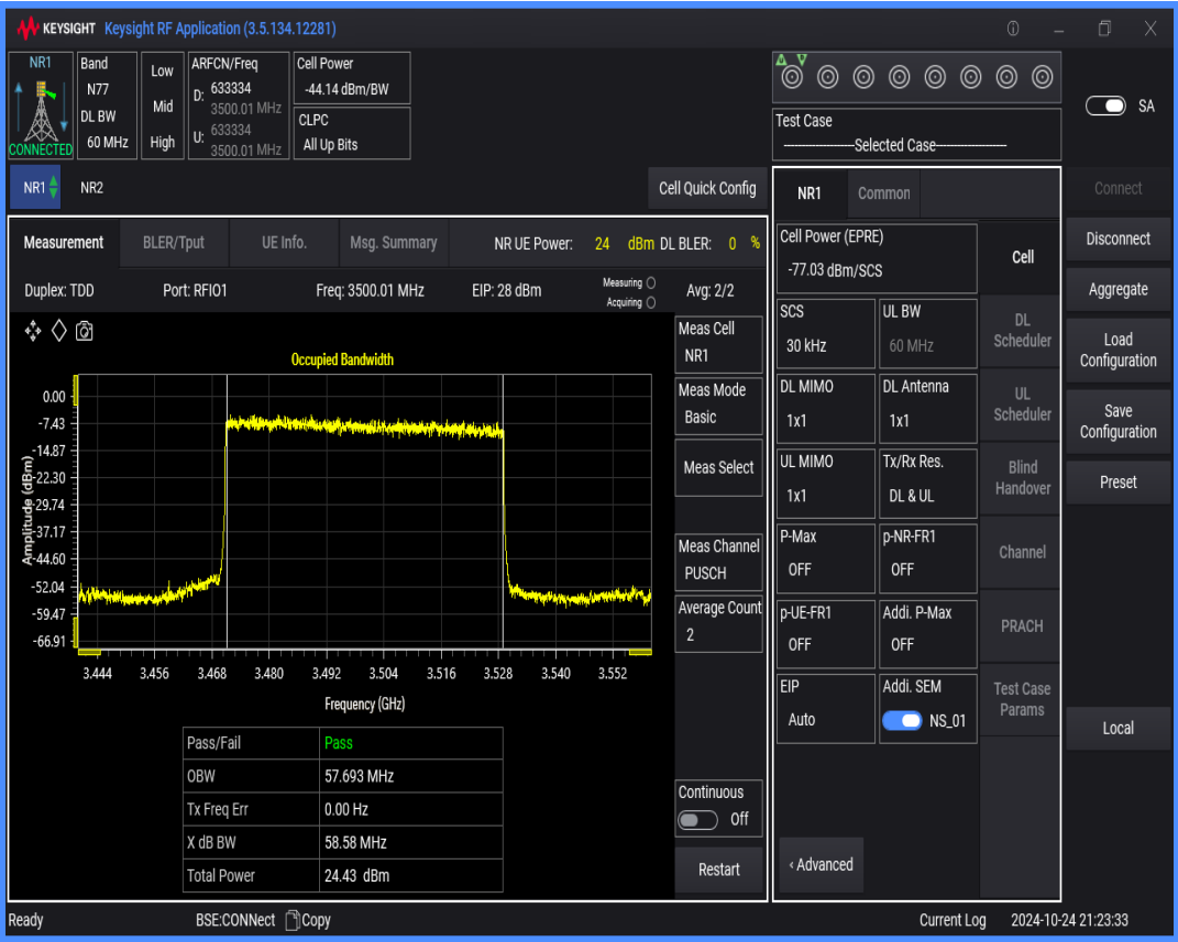
n77(3450-3550) SCS=30kHz DFT_QPSK BW=60MHz Channel=633334 RB=162@0
