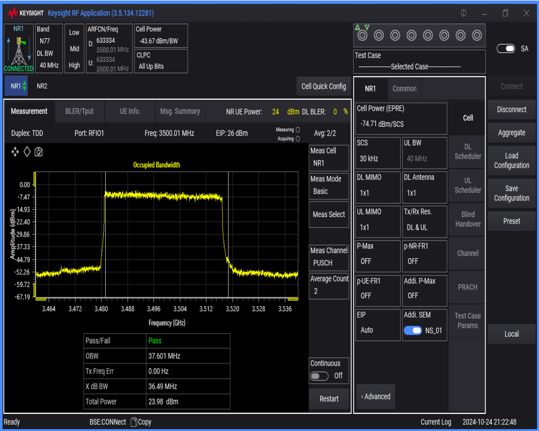
n77(3450-3550) SCS=30kHz DFT_QAM16 BW=40MHz Channel=633334 RB=100@0
