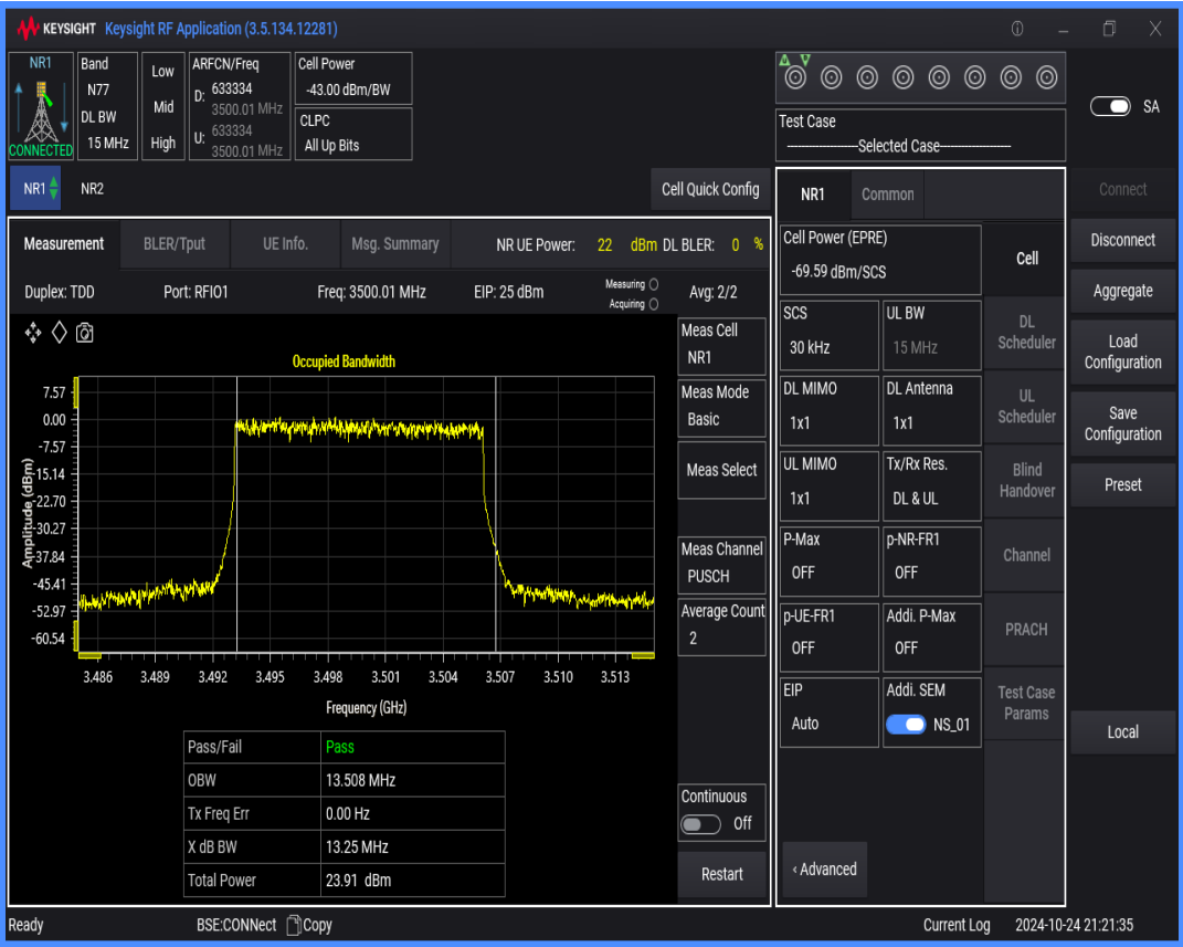
n77(3450-3550) SCS=30kHz DFT_QAM64 BW=15MHz Channel=633334 RB=36@0
