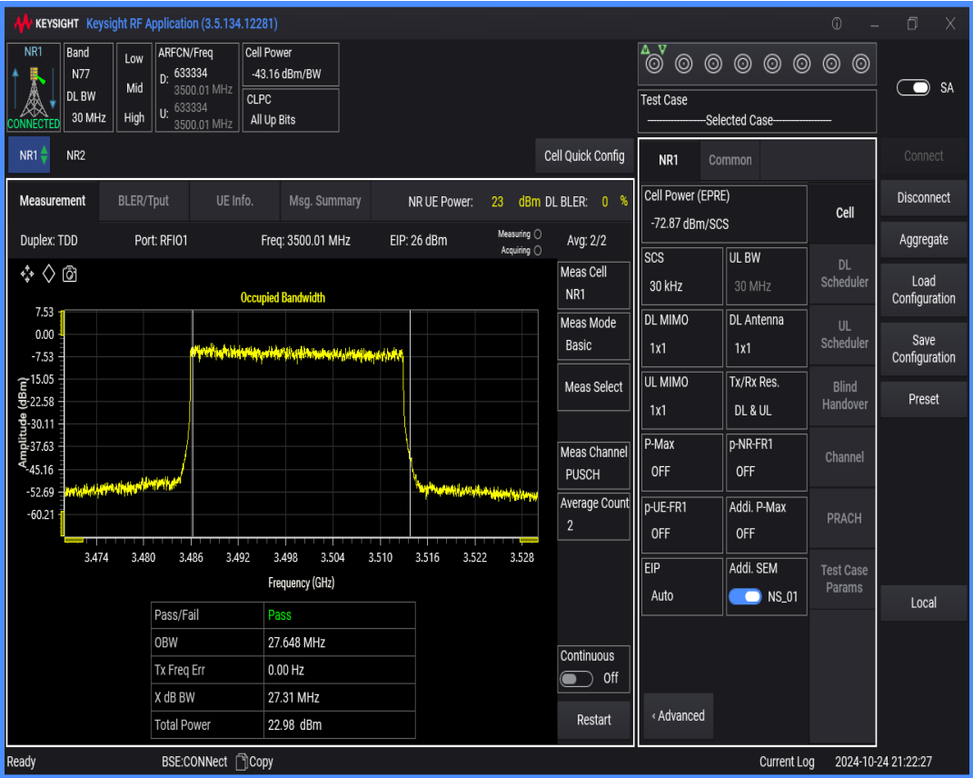
n77(3450-3550) SCS=30kHz DFT_QAM256 BW=30MHz Channel=633334 RB=75@0
