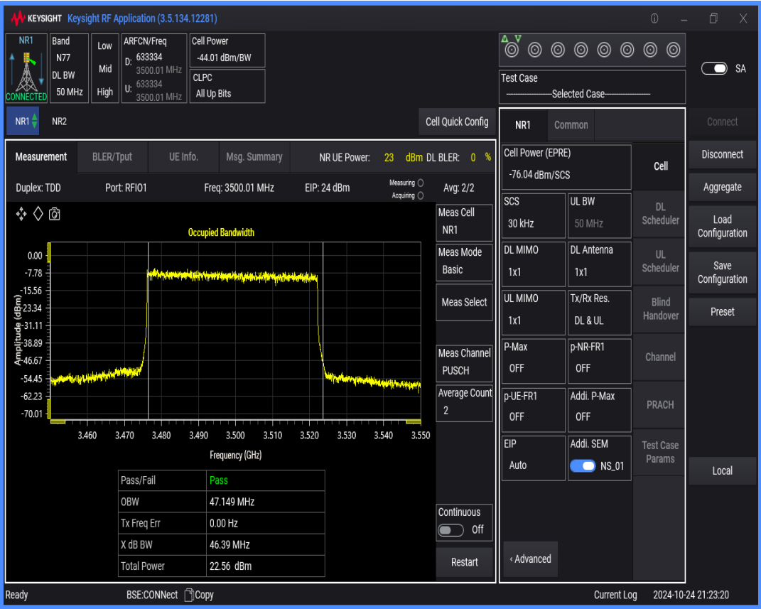
n77(3450-3550) SCS=30kHz DFT_QAM256 BW=50MHz Channel=633334 RB=128@0
