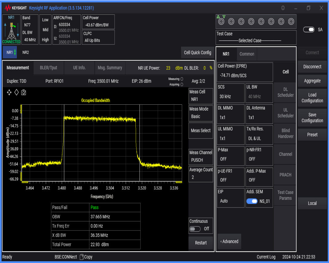
n77(3450-3550) SCS=30kHz DFT_QAM64 BW=40MHz Channel=633334 RB=100@0
