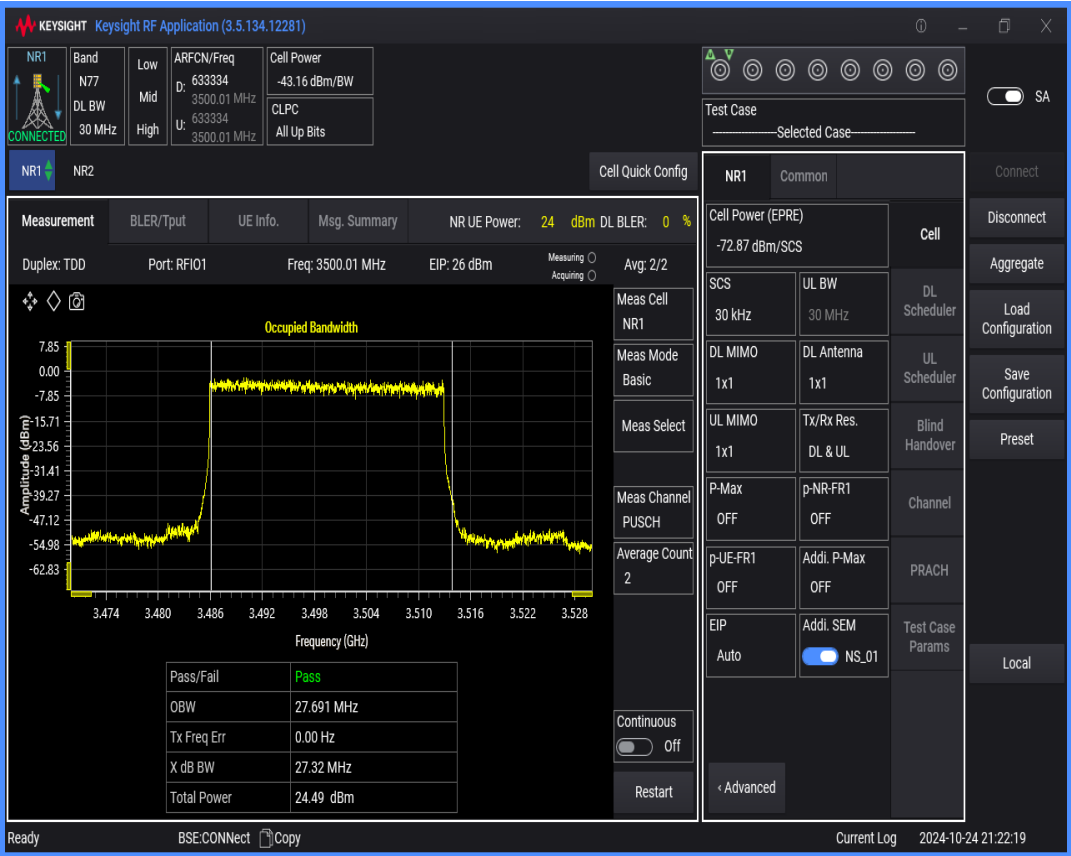
n77(3450-3550) SCS=30kHz DFT_QPSK BW=30MHz Channel=633334 RB=75@0
