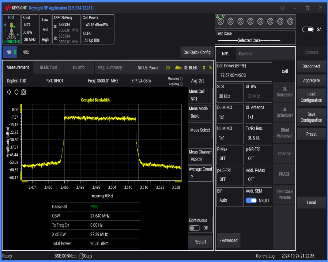
n77(3450-3550) SCS=30kHz DFT_QAM64 BW=30MHz Channel=633334 RB=75@0
