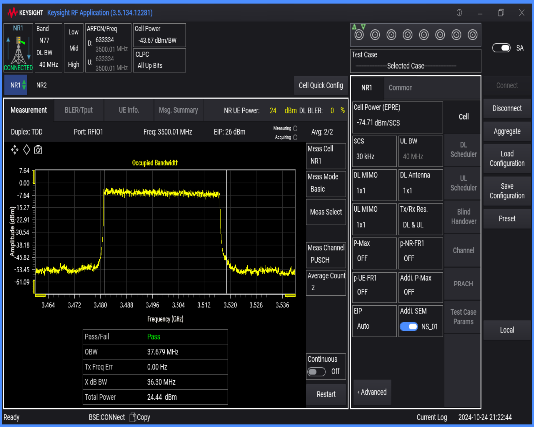
n77(3450-3550) SCS=30kHz DFT_QPSK BW=40MHz Channel=633334 RB=100@0
