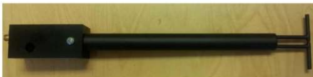
Figure 1 – MVG COMOSAR Validation Dipole
