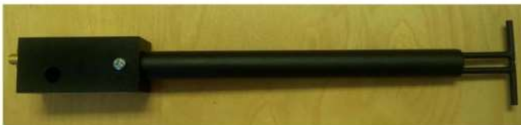
Figure 1 – MVG COMOSAR Validation Dipole
