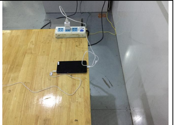
Conducted Emissions Test Setup Side View
