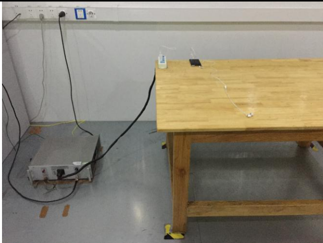
Conducted Emissions Test Setup Front View
