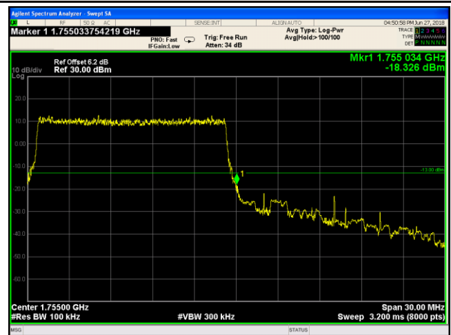
LTE Band IV - High Channel 16QAM-15
