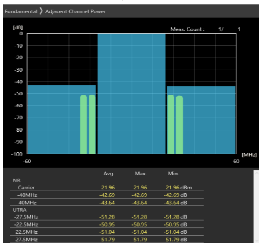
40MHz_30kHz_3570MHz-OFDM QPSK_RB50@25 -44.69,-46.78dB
