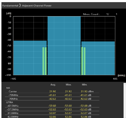
70MHz_30kHz_3585MHz-OFDM QPSK_RB90@45 -43.97,-46.08dB
