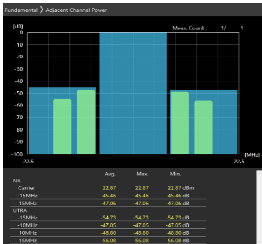
15MHz_30kHz_3557.5MHz-OFDM QPSK_RB36@0 -42.85,-43.43dB
