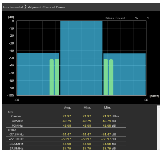
40MHz_30kHz_3570MHz-OFDM QPSK_RB50@25 -44.74,-46.82dB
