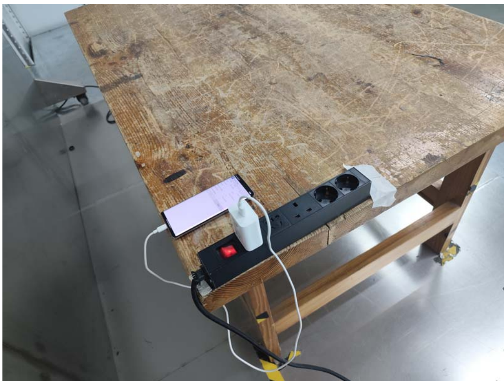
Conducted Emissions Side View
