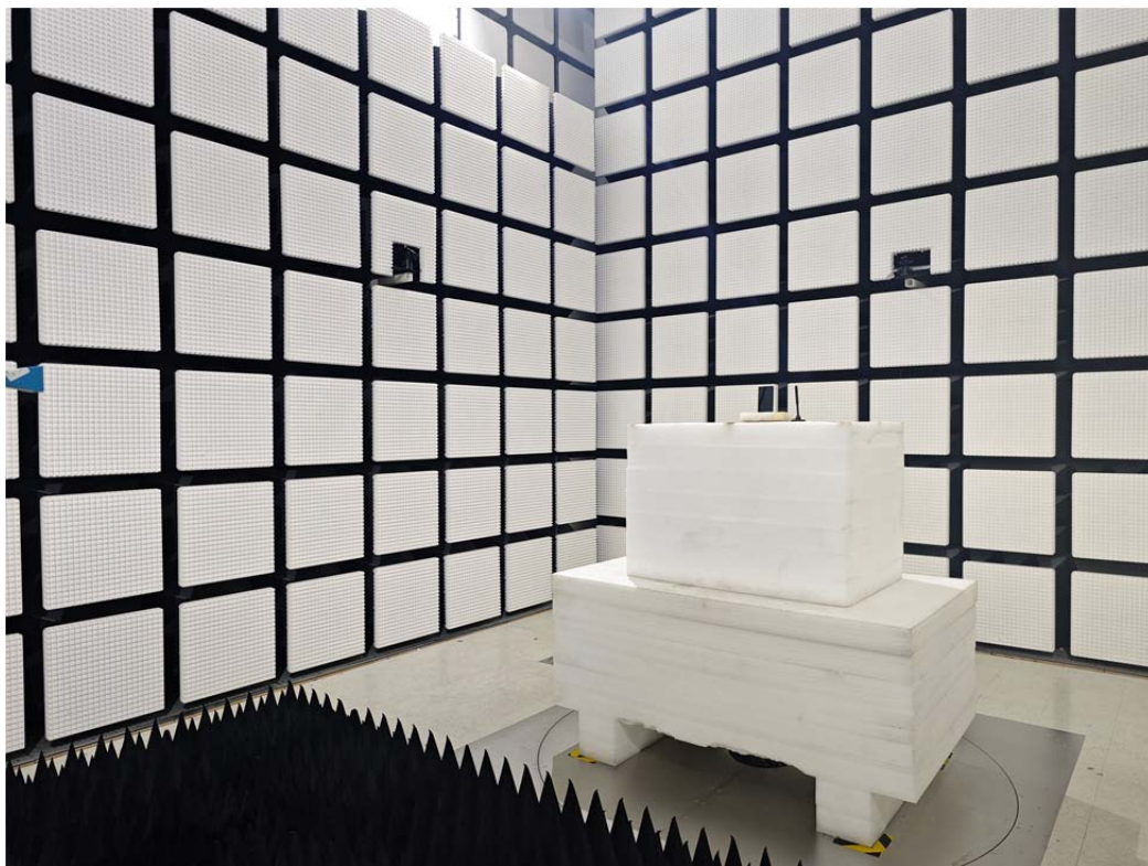
Radiated Emission Above 18-26.5GHz View
