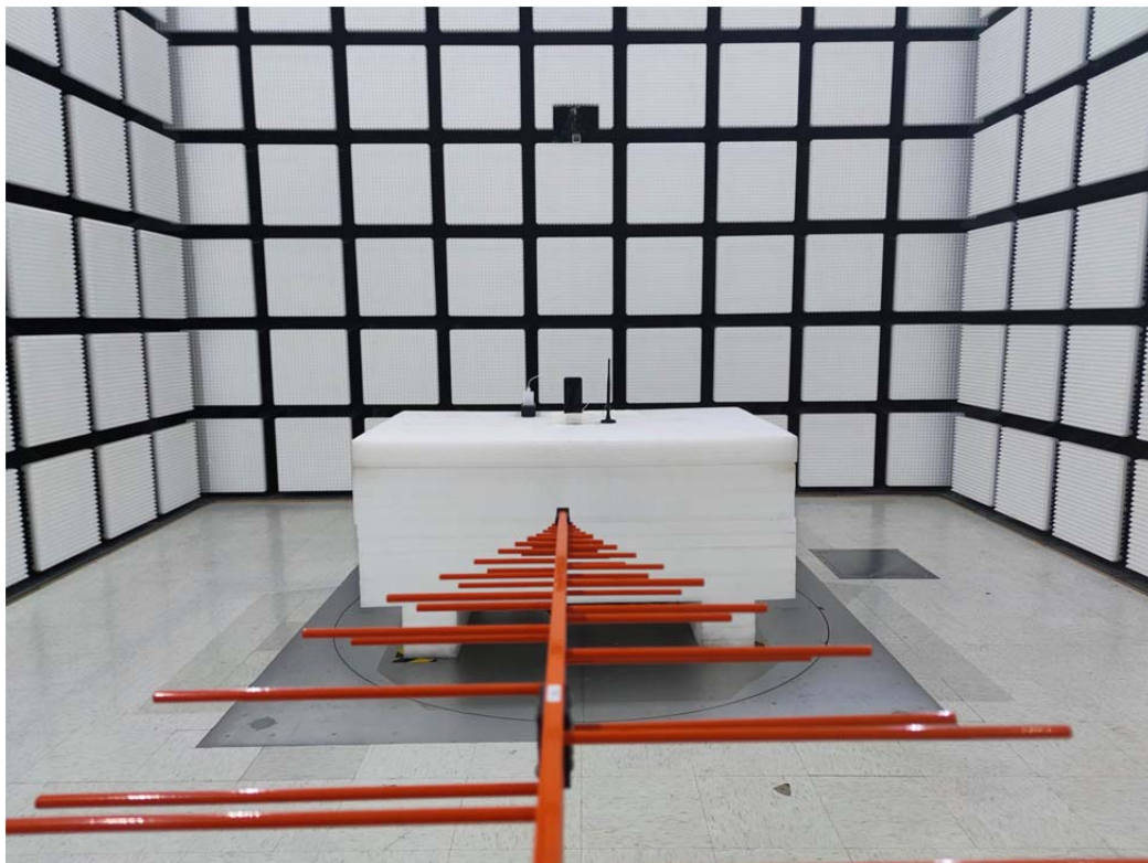
Radiated Emission 30 MHz-1 GHz View
