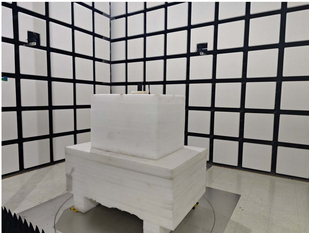
Radiated Emission Above 26.5-40GHz View
