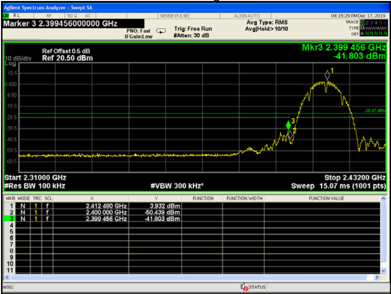
TX 11b: Band edge-left side
