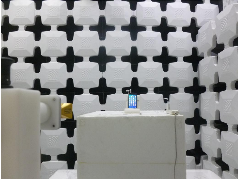
Radiated Spurious Emissions Test Setup Above 1GHz
