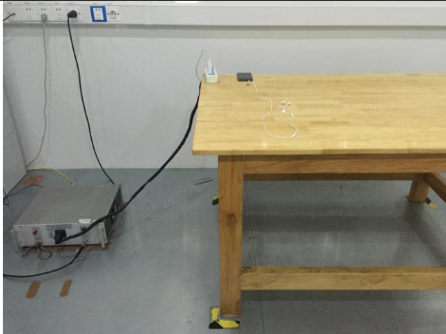
Conducted Emissions Test Setup Front View
