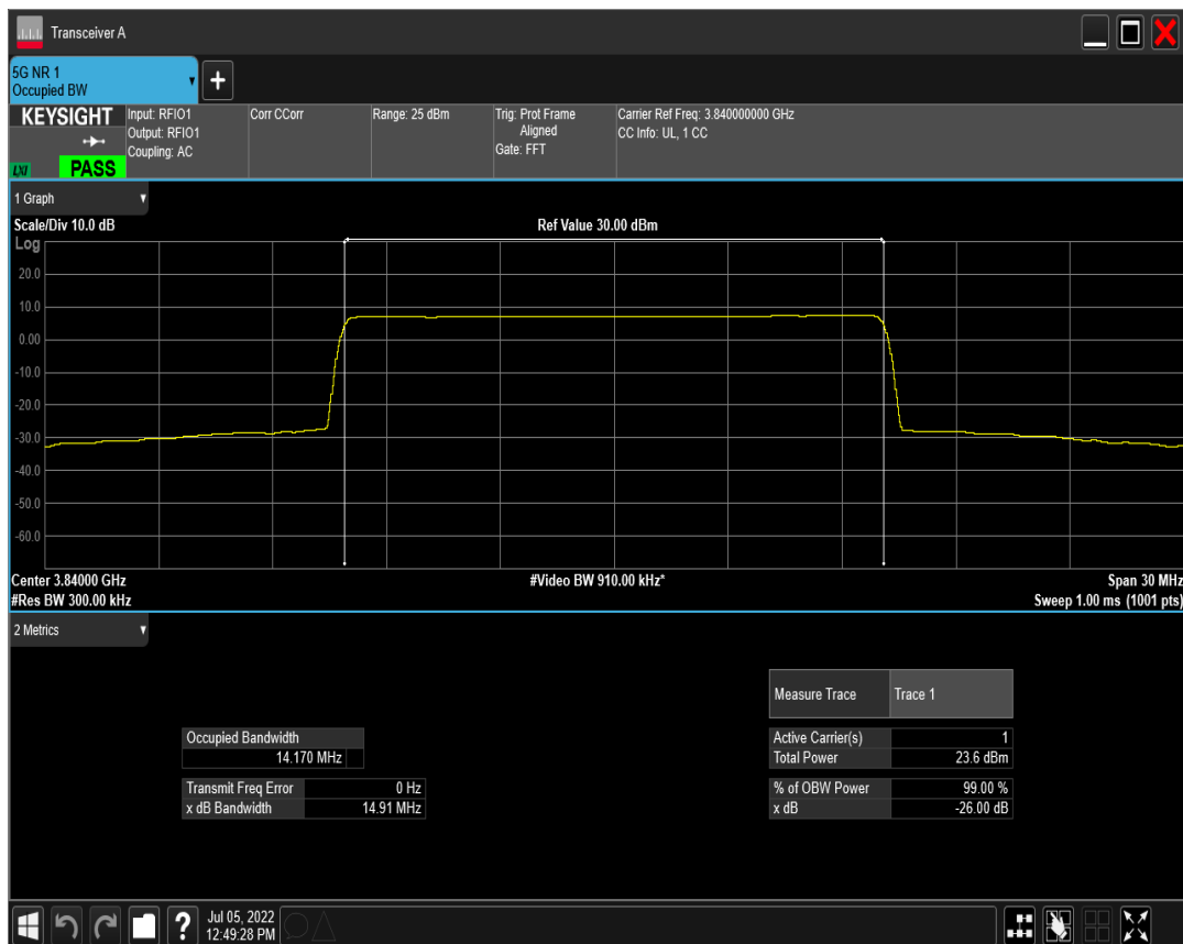
n77(3700-3980) SCS=15kHz DFT_BPSK BW=15MHz Channel=664832 RB=75@0
