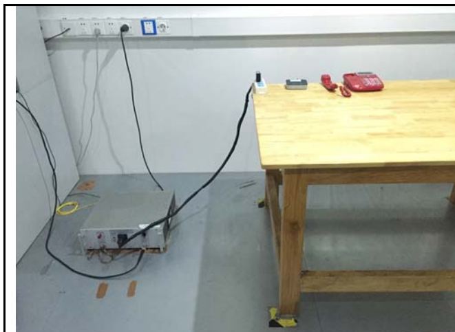
Conducted Emissions Test Setup – Front View
