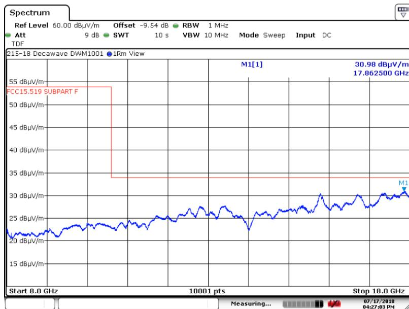
6.5.10. 8 to 18 GHz Vertical at 1 Meter, -9.54 dB offset in analyzer CH2
