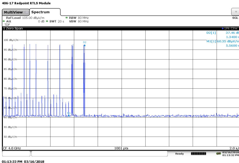
**Note:** Marker 1 is when the anchor (support equipment) stops transmitting, Marker D2 shows the EUT shutting off after 1.3 Seconds
