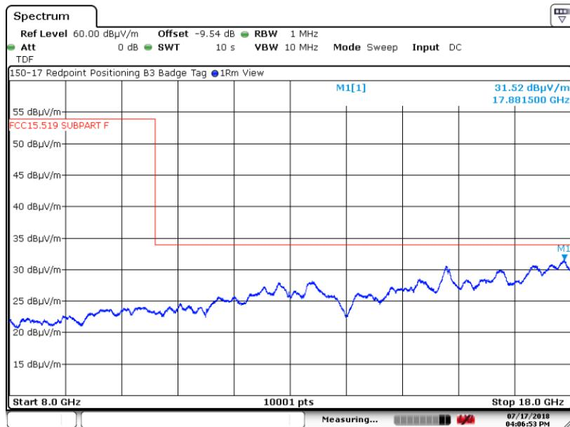
6.5.18. 8 to 18 GHz Vertical at 1 Meter, -9.54 dB offset in analyzer CH5
