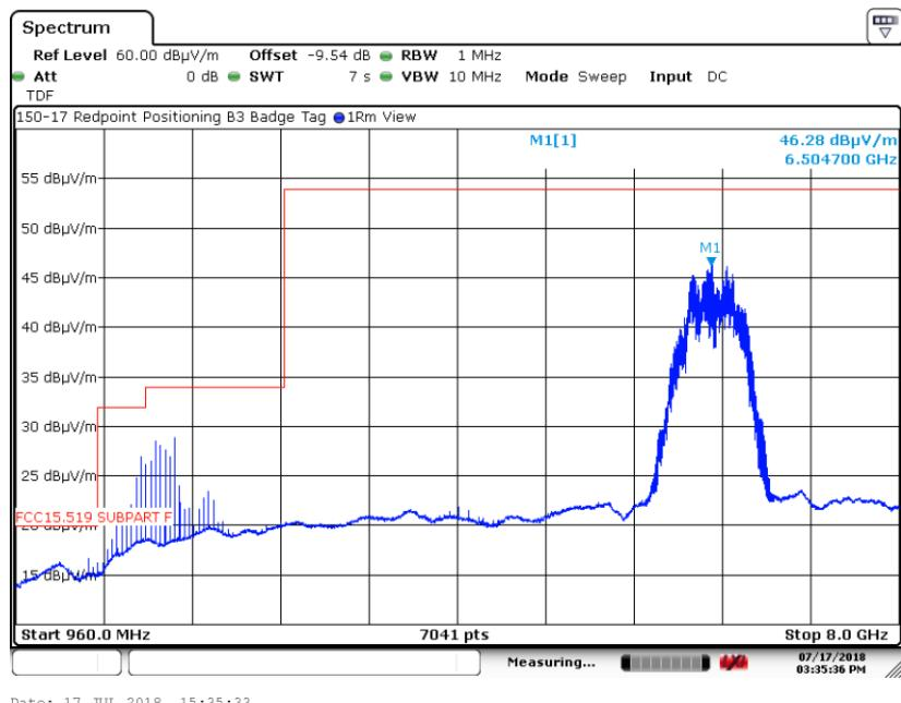
6.5.16. 960 MHz to 8 GHz Vertical at 1 Meter, -9.54 dB offset in analyzer CH5
