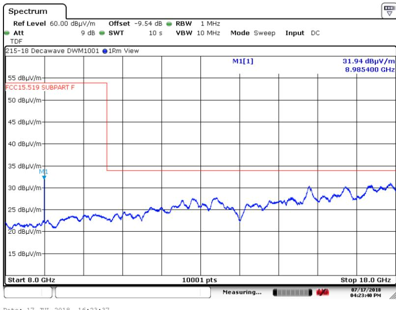
6.5.14. 8 to 18 GHz Vertical at 1 Meter, -9.54 dB offset in analyzer CH3
