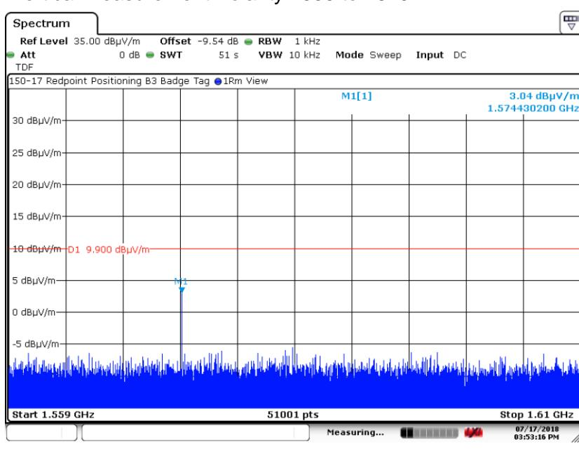
**Test Number: 150-17****Issue Date: 8/3/2018****6. Measurement Data (continued)****6.7. Radiated Emissions of UWB Transmission (15.519 (c), 15.521 (d))**
