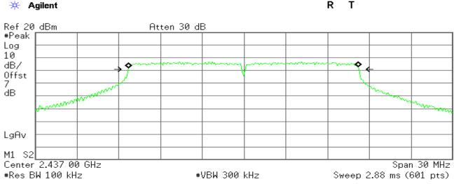
Occupied Bandwidth 16.4691 MHz Occ BW % Pwr 99.00 % x dB -6.00 dB
