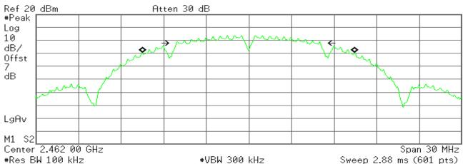
Occupied Bandwidth 14.9488 MHz Occ BW % Pwr 99.00 % x dB -6.00 dB
