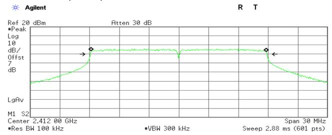
Occupied Bandwidth 17.6601 MHz Occ BW % Pwr 99.00 % x dB -6.00 dB
