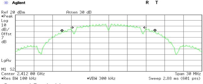
Occupied Bandwidth 14.9570 MHz Occ BW % Pwr 99.00 % x dB -6.00 dB
