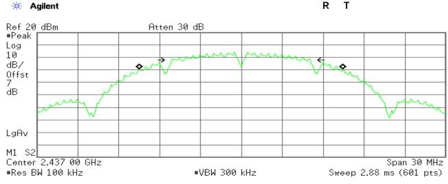
Occupied Bandwidth 14.9735 MHz Occ BW % Pwr 99.00 % x dB -6.00 dB
