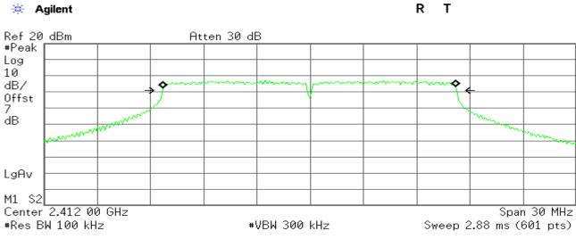
Occupied Bandwidth 16.4714 MHz Occ BW % Pwr 99.00 % x dB -6.00 dB
