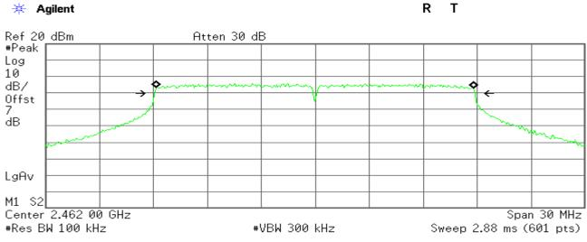
Occupied Bandwidth 17.6595 MHz Occ BW % Pwr 99.00 % x dB -6.00 dB
