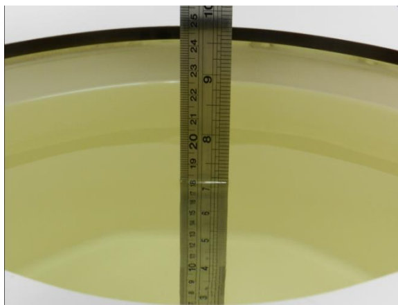
Fig 10.1 Photo of Liquid Height for Body SAR
