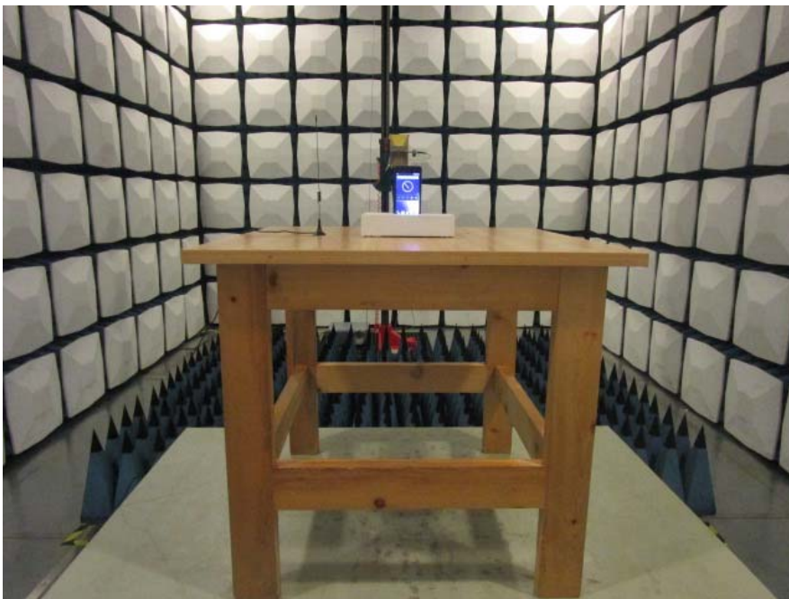
Radiated Emission View---Above 1GHz
