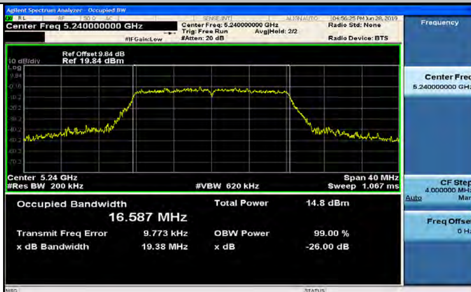
(26dB)Emission Bandwidth Measurement_11A_5240_Ant2
