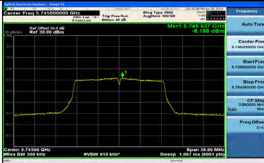
Maximum Power Spectral Density_TNVN_11A_5785_Ant2
