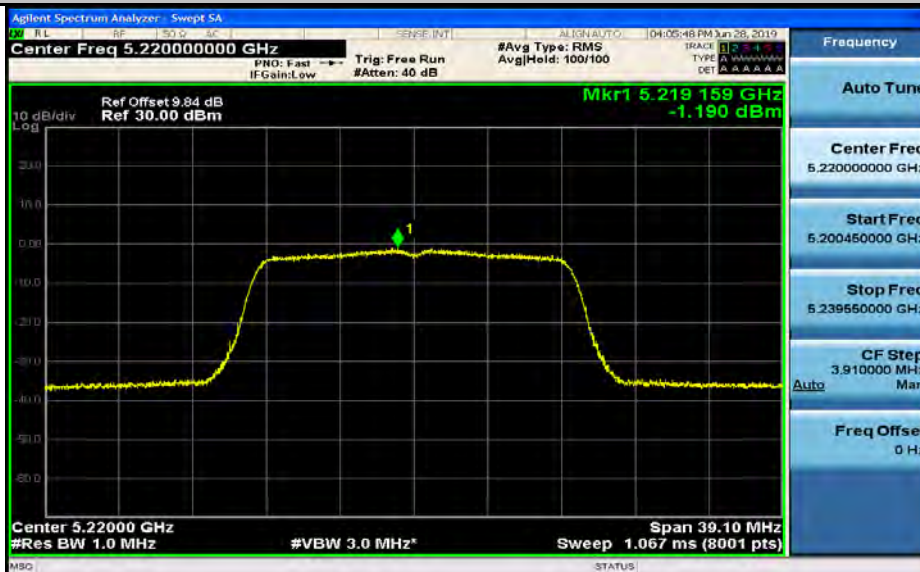
Maximum Power Spectral Density_TNVN_11A_5240_Ant1
