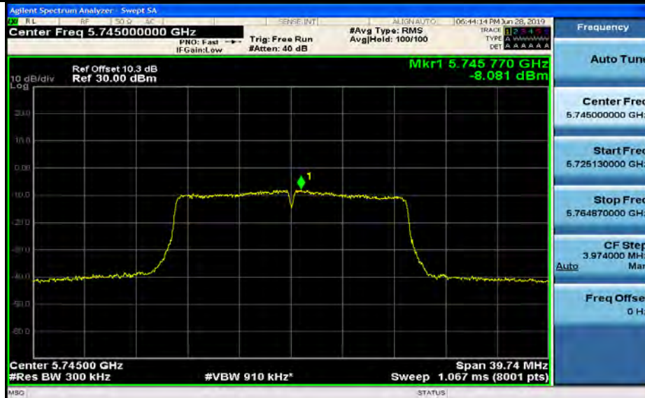
Maximum Power Spectral Density_TNVN_11N20_5785_Ant1
