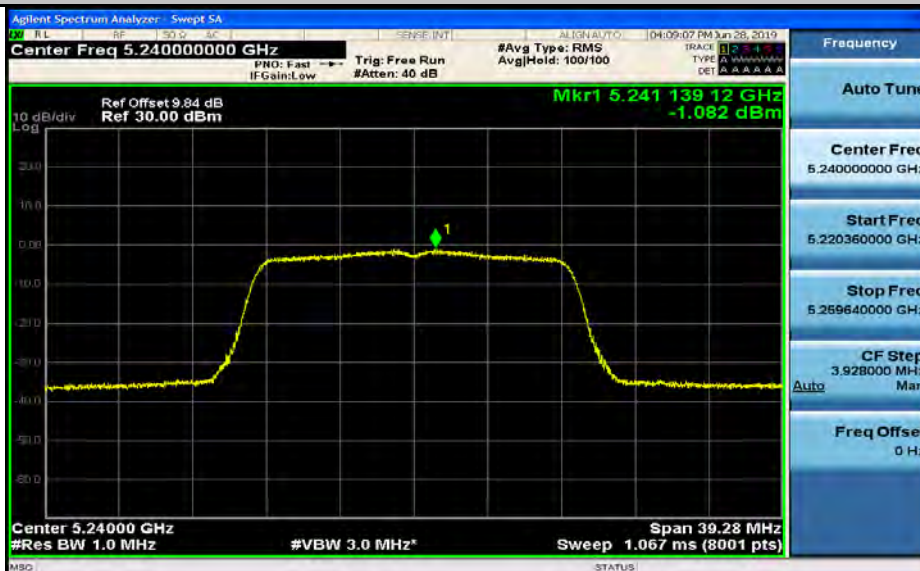
Maximum Power Spectral Density_TNVN_11A_5240_Ant1
