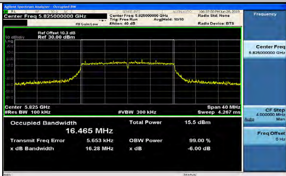
(6dB)Minimum Emission Bandwidth Measurement_11A_5825_Ant1
