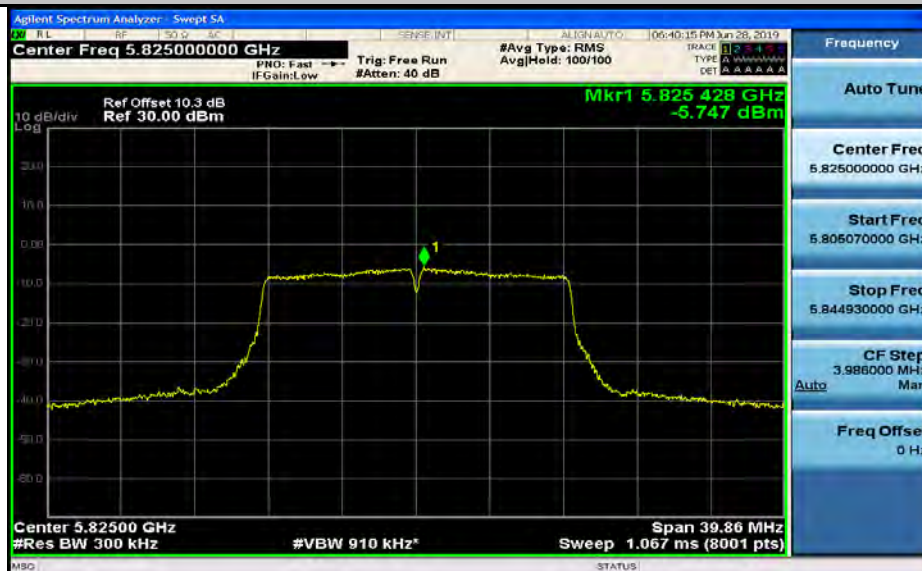
Maximum Power Spectral Density_TNVN_11A_5825_Ant1
