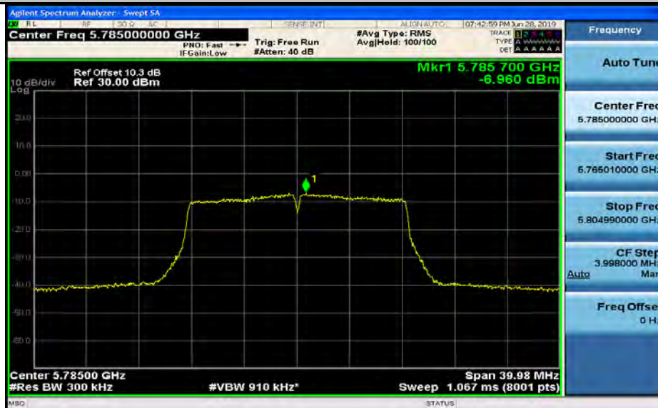
Maximum Power Spectral Density_TNVN_11A_5825_Ant2
