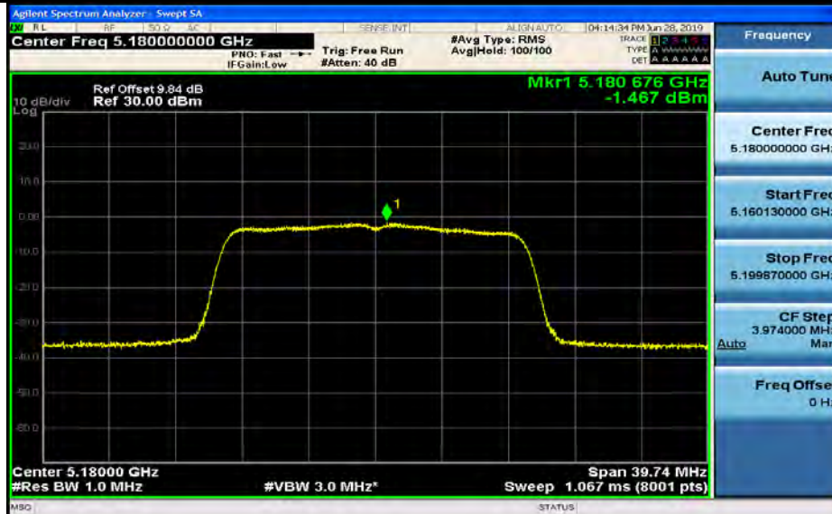
Maximum Power Spectral Density_TNVN_11N20_5220_Ant1
