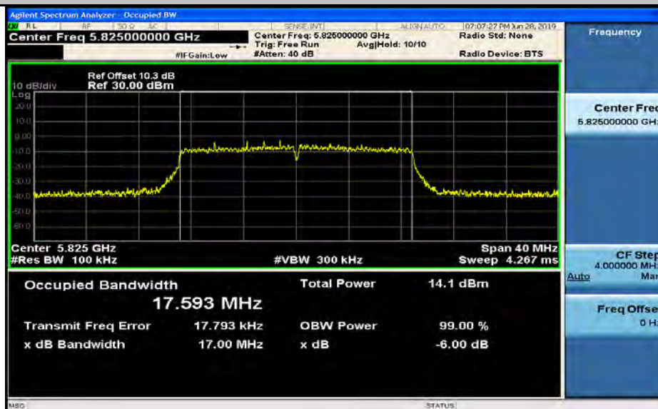
(6dB)Minimum Emission Bandwidth Measurement_11N20_5825_Ant1
