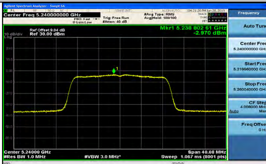
Maximum Power Spectral Density_TNVN_11N20_5240_Ant1
