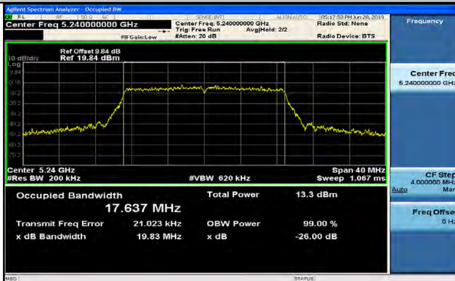
(26dB)Emission Bandwidth Measurement_11N20_5240_Ant2
