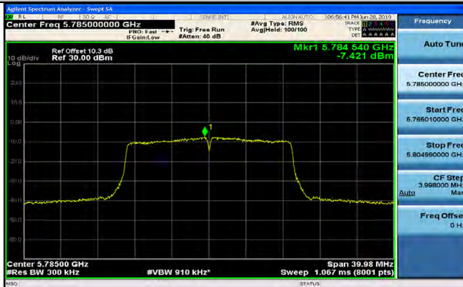
Maximum Power Spectral Density_TNVN_11N20_5825_Ant1
