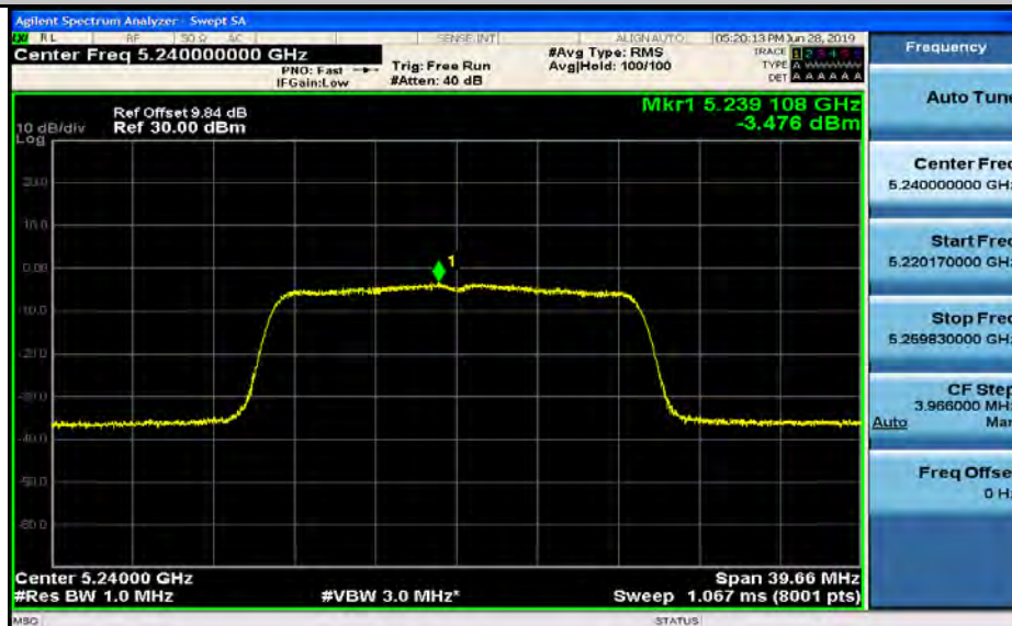
Maximum Power Spectral Density_TNVN_11N20_5240_Ant2
