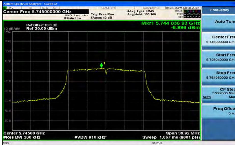
Maximum Power Spectral Density_TNVN_11A_5785_Ant1
