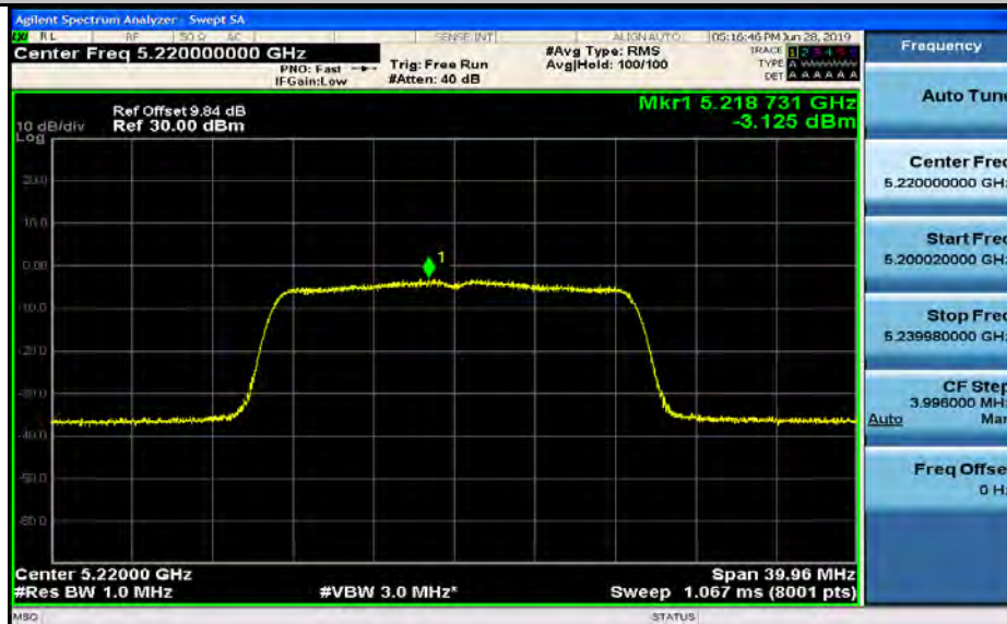
Maximum Power Spectral Density_TNVN_11N20_5240_Ant2
