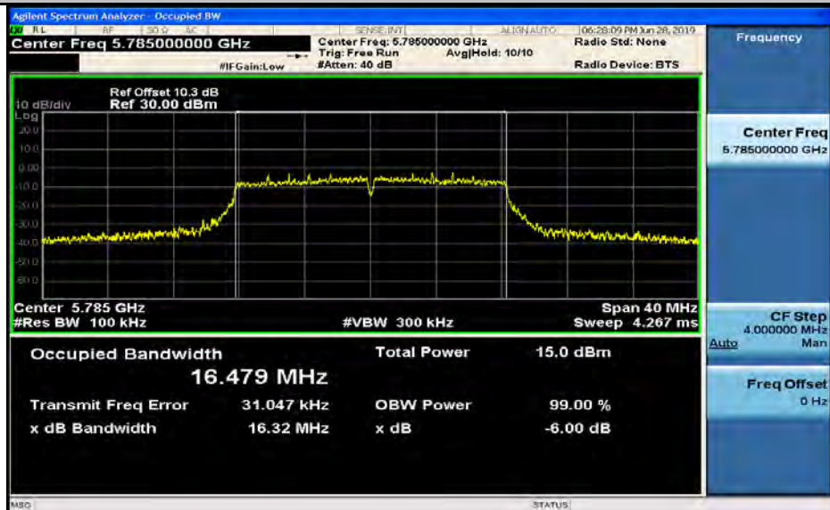
(6dB)Minimum Emission Bandwidth Measurement_11A_5825_Ant1
