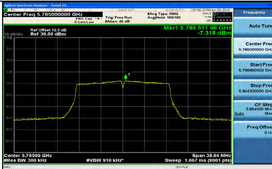
Maximum Power Spectral Density_TNVN_11N20_5825_Ant2
