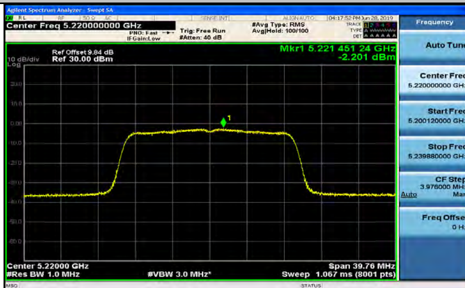
Maximum Power Spectral Density_TNVN_11N20_5240_Ant1
