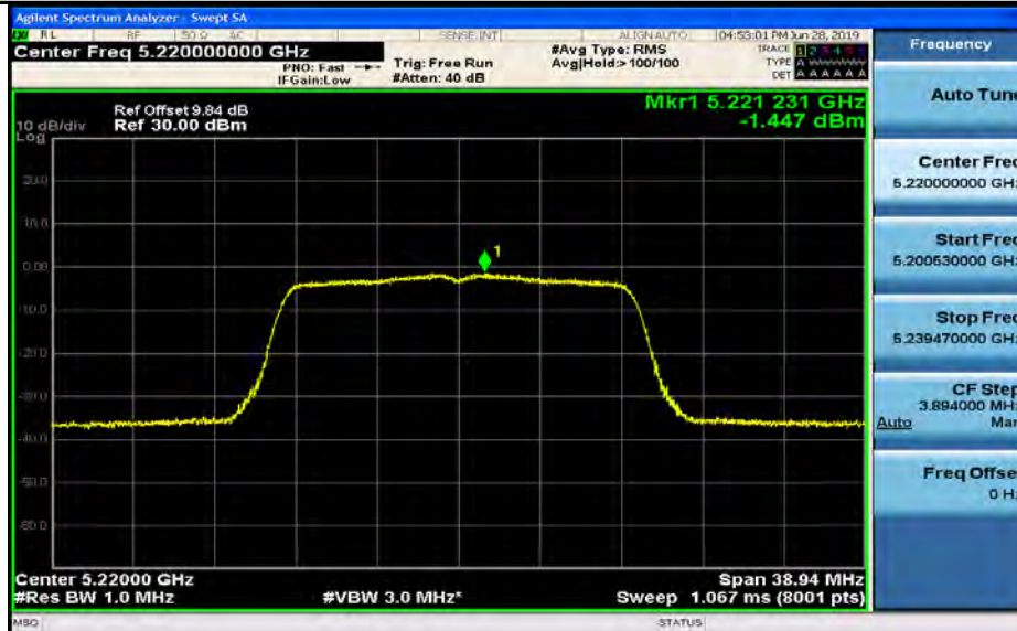
Maximum Power Spectral Density_TNVN_11A_5240_Ant2
