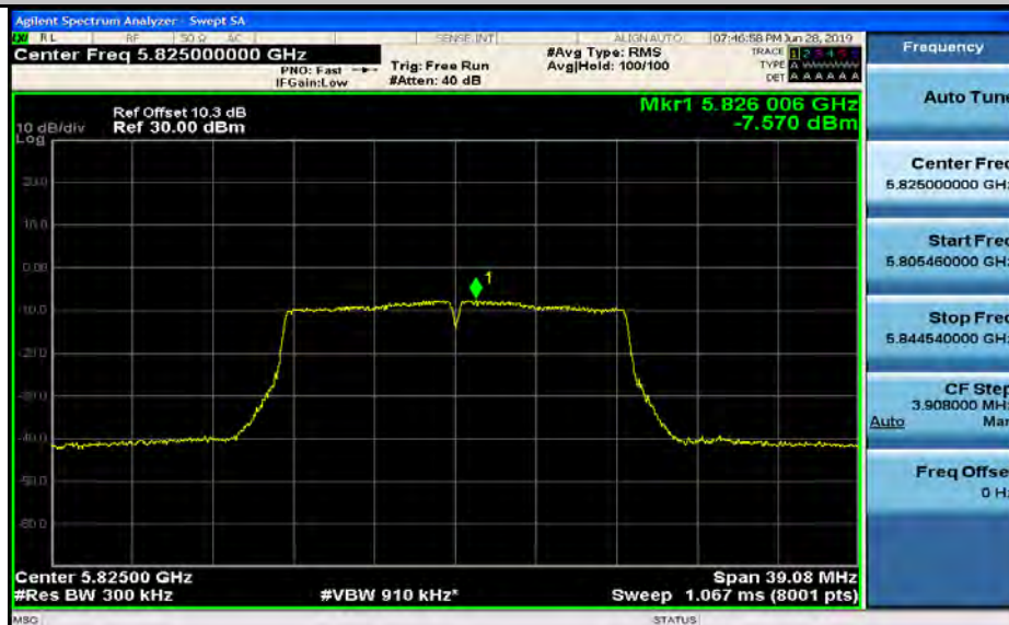
Maximum Power Spectral Density_TNVN_11A_5825_Ant2
