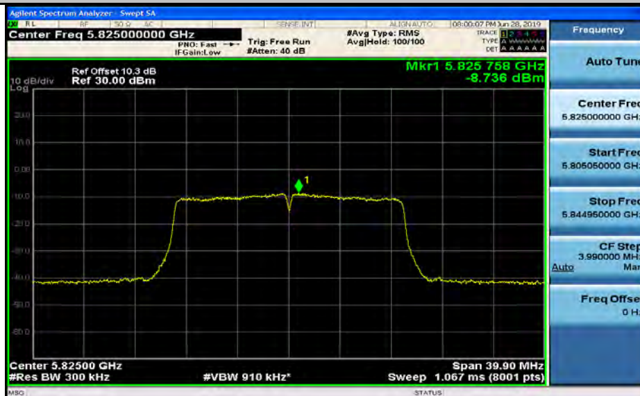
Maximum Power Spectral Density_TNVN_11N20_5825_Ant2
