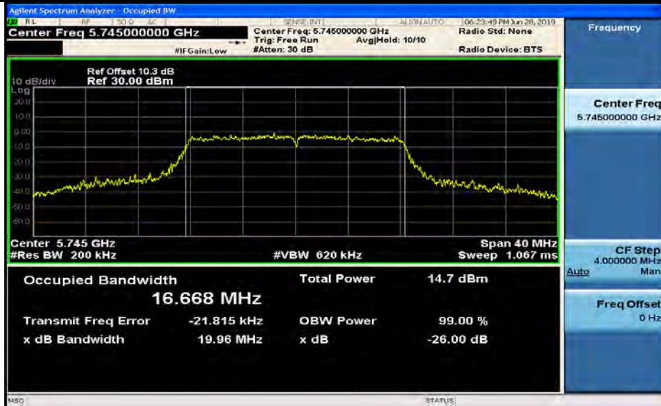
(26dB)Emission Bandwidth Measurement_11A_5785_Ant1
