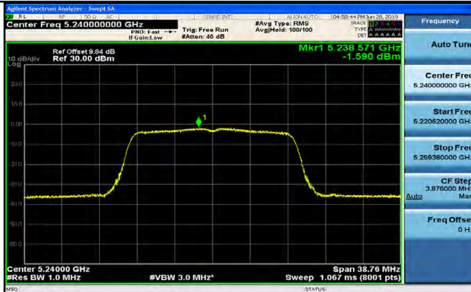
Maximum Power Spectral Density_TNVN_11A_5240_Ant2
